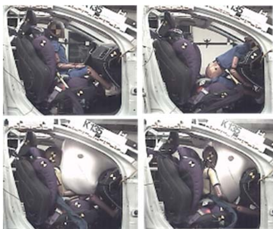
Fig. 16(c). Situation 14, HIII6y/Q6, belt placed behind the back , front-mid seat position, pulse A; top row : tests without airbag; bottom row : with airbag. First airbag contact ( left ), max. forward position ( right ).
