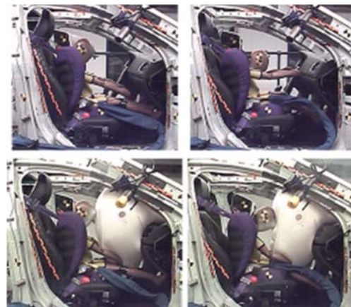
Fig. 10(b). Situation 7, Q6, mid-mid seat position, crash pulse C; top row : tests without airbag; bottom row : with airbag. First airbag contact ( left ), max. excursion ( right ).
