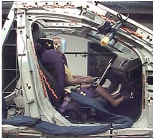
Fig. 2. Sled test set-up.
