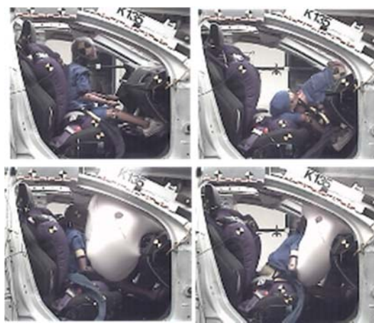
Fig. 16(d). Situation 17, HIII6y/Q6, belt placed behind the back mid-mid seat position, pulse B; top row : tests without airbag; bottom row : with airbag. First airbag contact ( left ), max. forward position ( right ).
