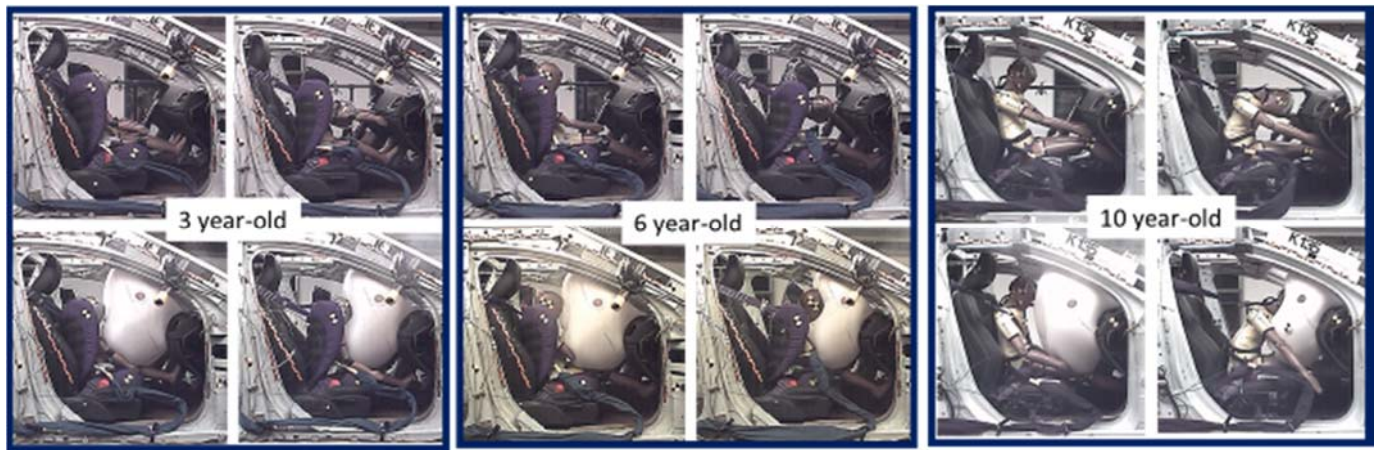
Fig. 4. Situations 2, 6 and 19, comparing the dummy sizes (Q3, Q6, Q10) in mid-mid seat position. Top row : tests without airbag; bottom row : with airbags. First airbag contact ( left in each pair ), and max. excursion ( right in each pair ).
