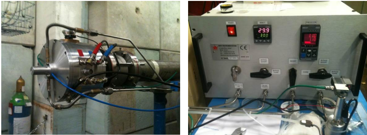
Fig. 2. (Color online) Left: The new LICORNE neutron source convertor; Right: The hydrogen gas pressure and flow control system.
