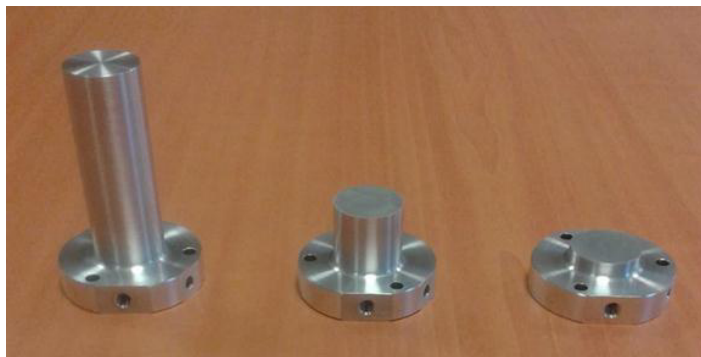
Fig. 3 (Color online) The exchangeable gas cells of different lengths (7.5cm, 3.5cm and 2cm).
