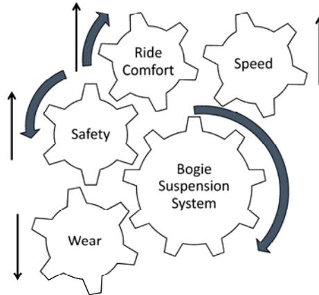
Fig. 1: Conflicting effects of bogie suspension system on vehicle performance.
