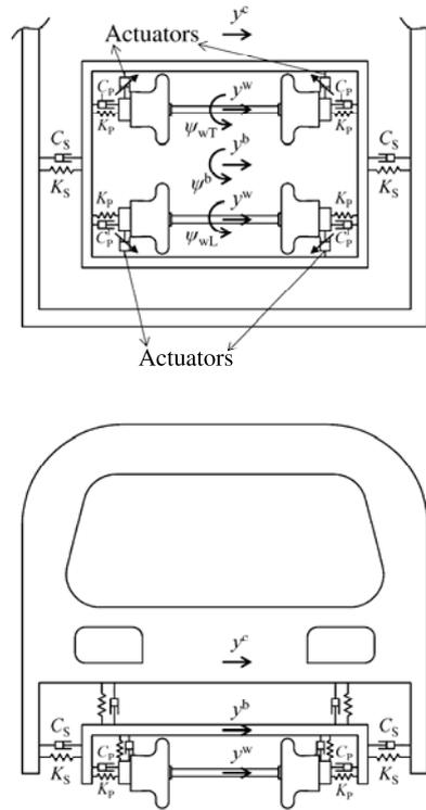
Fig. 4: Half-car railway vehicle model B.
