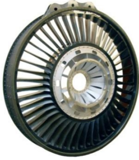
Figure 1.2: A hybrid composite/metal fan frame for a commercial aircraft engine that was developed by GKN Aerospace as a demonstrator [5].
