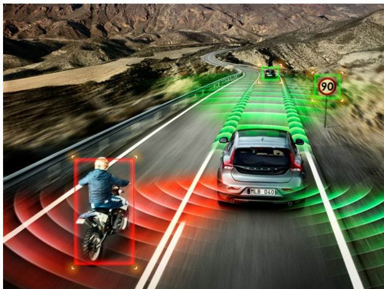
Figure 2.2: Advanced Driver Assistance Systems e.g., Adaptive Cruise Control, Lane Keeping Aid, Road Sign Information, and Blind Spot Information System [9].
