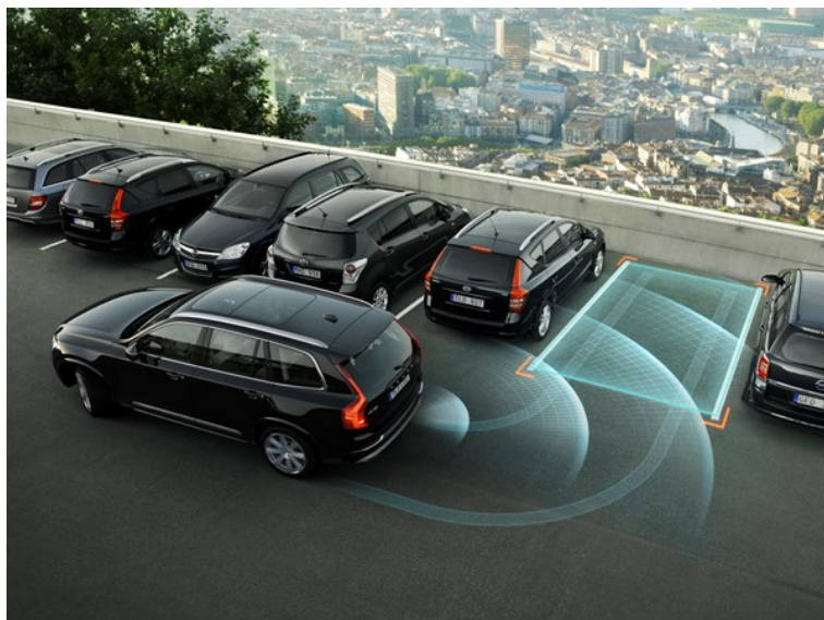
Figure 2.3: Parking assistance system for automatic reversing into a parking space [9].
