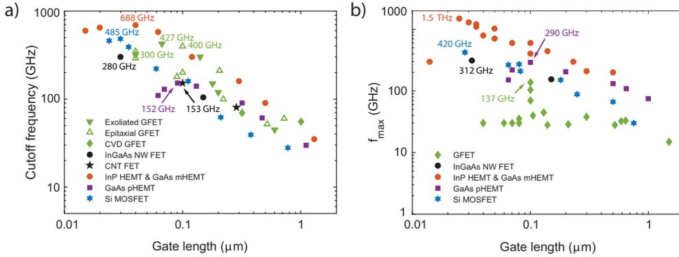
**Fig. 1.1:** State-of-the-art de-embedded a)  $f_T$  and b)  $f_{max}$  for HEMTs, Si CMOS, CNT [11,17] and NW FETs [15,16] against reported intrinsic GFETs [11,17–21].
