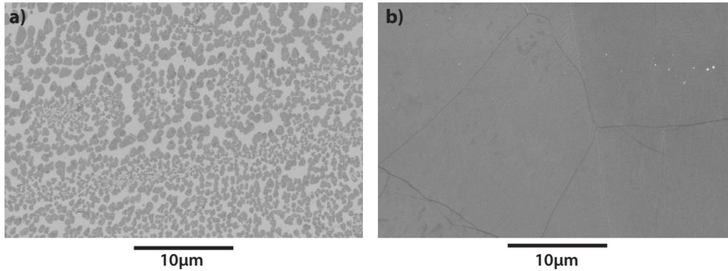
**Fig. 2.5:** SEM images of as-synthesised in-house CVD graphene on Cu foil that demonstrates a) the high nucleation density on a partially covered sample and in b) mutually rotated graphene domains on a continuously grown sample.
