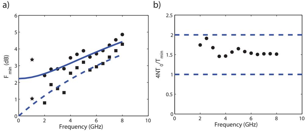
**Fig. 3.10:** a) Measured (●) and intrinsic (■)  $F_{min}$  of a  $2 \times 30 \mu\text{m}$  device at  $I_{ds} = 370$  mA/mm [Paper F]. Values from [Paper E] given by (★). b) The measured noise parameters fulfils the requirement that  $1 < 4NT_0/T_{min} < 2$  [113].
