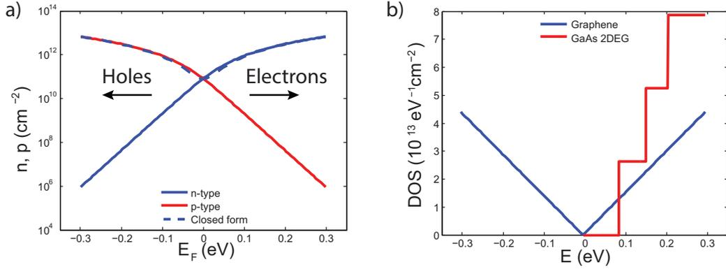
**Fig. 2.3:** a) Carrier concentrations versus  $E_F$  at room temperature [23] and b) DOS in graphene compared with an AlGaAs/GaAs 2DEG with  $n_s = 0.67 \cdot 10^{12} \text{ cm}^{-2}$  [44].
