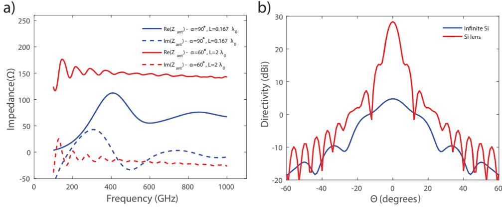
**Fig. 4.12:** a) Simulated antenna impedance from CST for the bow-tie antennas in [Paper B] ( $\sim 65 \Omega$ ) and [151] ( $\sim 150 \Omega$ ). The lengths are given in free-space wavelengths at 600 GHz. b) Simulated antenna patterns from CST for the bow-tie antenna in [Paper B] on an infinite Si substrate and an hyperhemispherical Si lens with diameter  $d = 2R = 5 \text{ mm} = 10\lambda_0$  at 600 GHz and extension  $L = R/\sqrt{\epsilon_r}$ .
