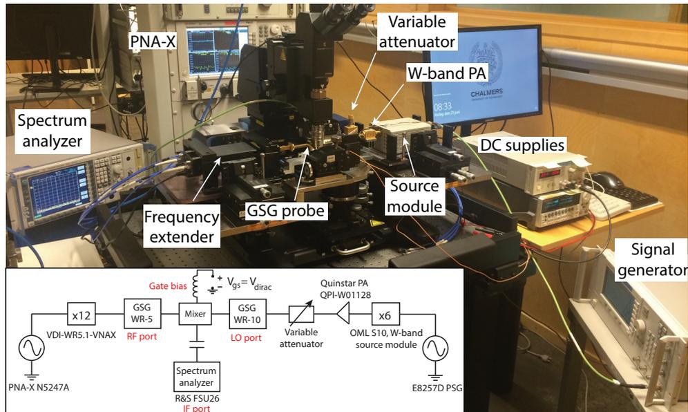
**Fig. 4.10:** The on-wafer RF measurement setup used to characterise the G-band subharmonic resistive GFET mixer IC reported in [Paper C]. The reference receiver of the PNA is used to level the mixer input power at the extender output.
