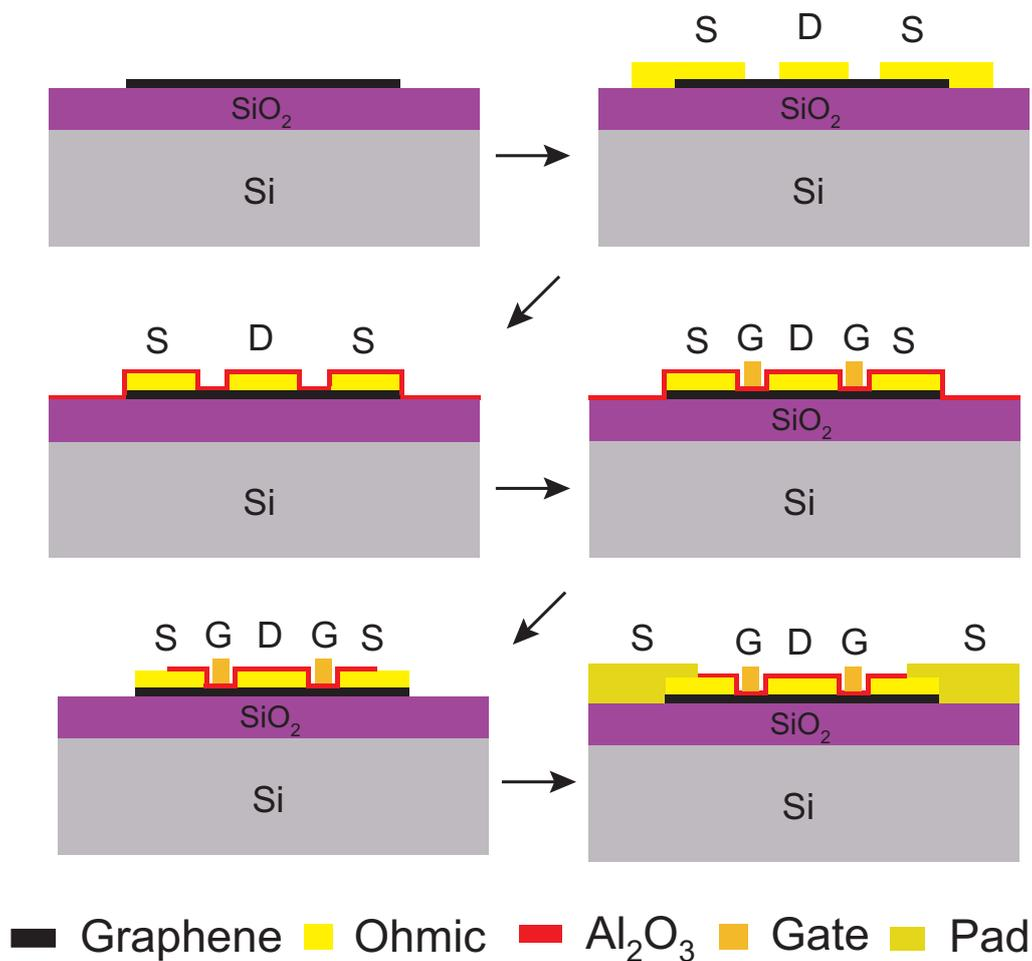
**Fig. 3.1:** Schematics of the fabrication steps for a two-finger GFET.
