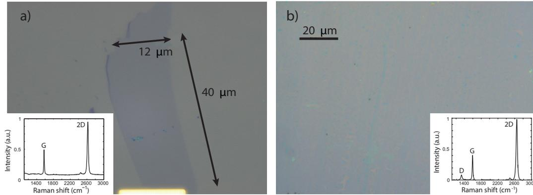
**Fig. 2.4:** Optical identification of single-layer graphene on SiO<sub>2</sub>/Si substrate by a) exfoliation and b) CVD growth on Cu catalyst in a virtually hole-free area. The insets show the respective Raman signature characteristic of monolayer graphene.
