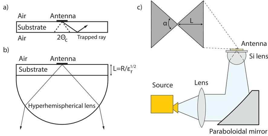
**Fig. 4.11:** a) Planar antenna radiating on a substrate illustrating the trapped rays. b) The same planar antenna on a hyperhemispherical lens to prevent reflected rays. c) Quasi-optical circuit used to match the Gaussian beam wavefront from the source to the lens [Paper B]. The inset shows the bow-tie angle  $\alpha$  and the bow-tie length  $L$ .
