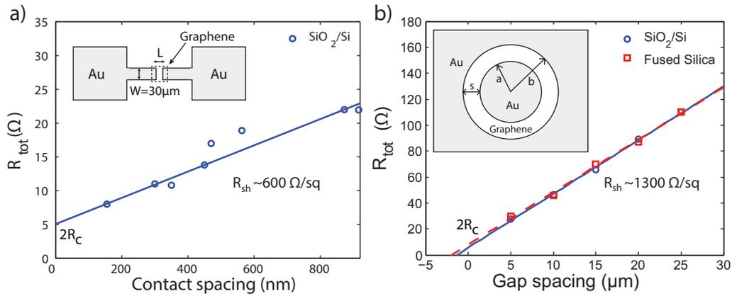
**Fig. 3.4:** TLM results for CVD graphene on  $\text{SiO}_2/\text{Si}$  substrates with a) Pd based contact which gives  $R_c W = 80 \Omega\mu\text{m}$  [Paper F] and b) Ti metallised contact with  $R_c W = 900 \Omega\mu\text{m}$  [Paper G]. The insets illustrate the TLM structure layouts.
