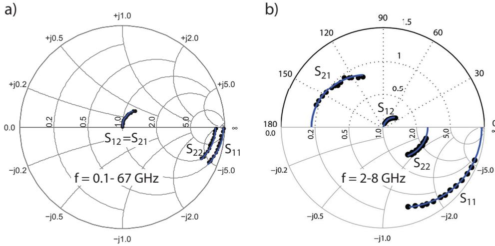
**Fig. 3.8:** The S-parameters of a) passive GFET, which is reciprocal ( $S_{12} = S_{21}$ ) with  $L_g = 1 \mu\text{m}$  and  $W_g = 2 \times 1.25 \mu\text{m}$  [Paper A], and b) active GFET, which has forward gain ( $S_{21} > 1$ ) with  $L_g = 1 \mu\text{m}$  and  $W_g = 2 \times 60 \mu\text{m}$  [Paper F].
