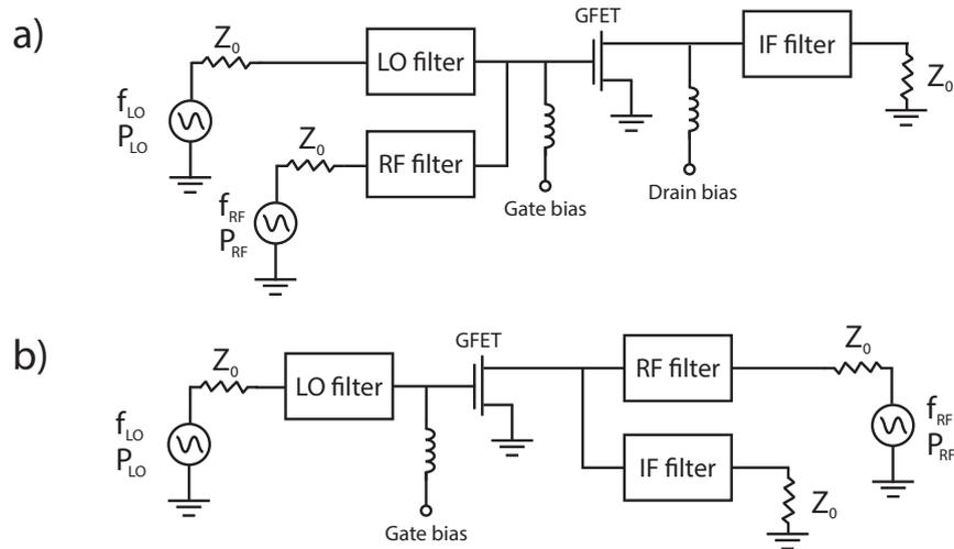
**Fig. 4.5:** Schematic circuits for single-ended a) active and b) resistive GFET mixers.
