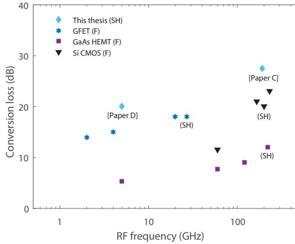
**Fig. 4.6:** Conversion loss for the GFET resistive mixers in [Paper C] and [Paper D] compared to the literature [83, 142, 143] and to other FET resistive mixers realised in the mature GaAs [132, 141] and Si CMOS [146, 147] technology nodes. The labels correspond to the following: F = Fundamental, SH = SubHarmonic.
