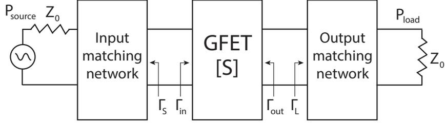
**Fig. 4.2:** Schematic drawing of a single-stage small-signal GFET amplifier layout.
