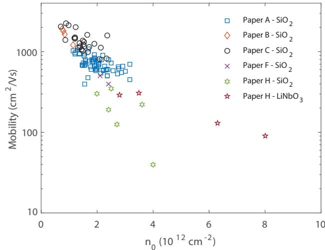
**Fig. 3.5:** Compilation of hole mobilities versus the residual concentrations extracted from fitting of Eq. 2.4 using top gates. All devices were fabricated on CVD graphene in different batches during the work on the papers appended to this thesis.
