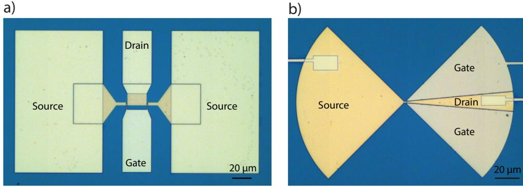
**Fig. 3.2:** Two finalised GFETs outlined with a) coplanar access pads for on-wafer characterisation and b) a broadband bow-tie antenna for free-space characterisation.
