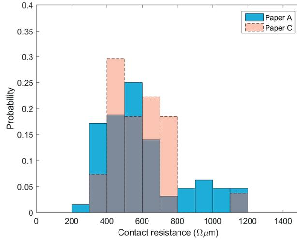
**Fig. 3.3:** Two-probe contact resistance extracted with Eq. 2.4. The distribution is for  $\sim 100$  GFETs from batches fabricated in the process of [Paper A] and [Paper C].
