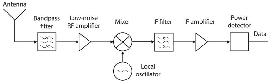
**Fig. 1.2:** The block diagram of a typical heterodyne receiver. The mixer is not present in an incoherent receiver, resulting in lower spectral resolution.
