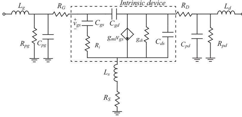
**Fig. 3.7:** The linear small-signal equivalent circuit of an FET, which is divided into DC-bias-independent parasitics and DC-bias-dependent intrinsic elements.
