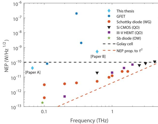
**Fig. 4.13:** Comparison of NEP for GFET detectors in [Paper A] and [Paper B] to literature [153–155] and to other solid-state rectifiers: Schottky diodes [156–158], Si CMOS [13], III-V HEMTs [159, 160], and Sb backward diodes [161]. The labels correspond to: OW = On-Wafer, WG = WaveGuide, and QO = Quasi-Optical.
