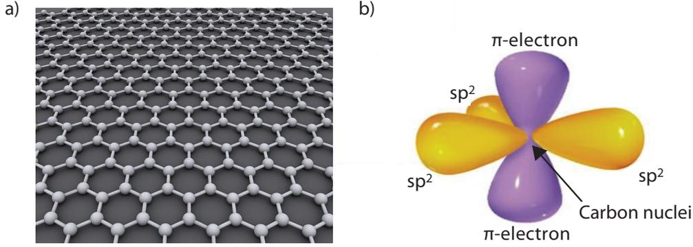
**Fig. 2.1:** a) Graphene honeycomb lattice. b) Visualisation of electron clouds in  $sp^2$ -hybridisation, localised in plane  $\sigma$ -bonds and out of plane delocalised  $\pi$ -electrons [34].
