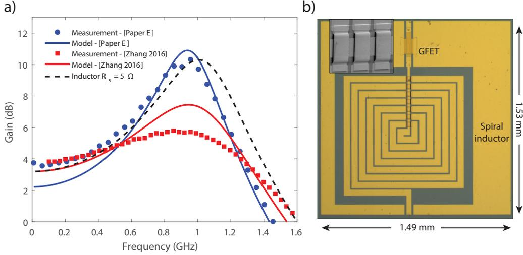
**Fig. 4.3:** a) Performance of small-signal GFET amplifiers using an exfoliated GFET ( $L_g = 1 \mu\text{m}$ ,  $W_g = 2 \times 30 \mu\text{m}$ ) and a wire inductor [Paper E], as well as a CVD GFET ( $L_g = 1 \mu\text{m}$ ,  $W_g = 2 \times 120 \mu\text{m}$ ) and a planar inductor [96]. The dashed black line shows the CVD GFET matched with a similar but low-loss planar inductor. b) Micrograph of the planar amplifier with SEM image of the airbridges in the inset.
