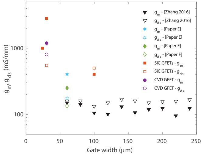
**Fig. 3.6:** Extrinsic transconductance and output conductance of the CVD GFETs in [96], [Paper F] and the exfoliated GFET [Paper E]. For comparison, the reported values for ultrathin gate oxide SiC [21, 97, 98] and CVD [99] GFETs are given.
