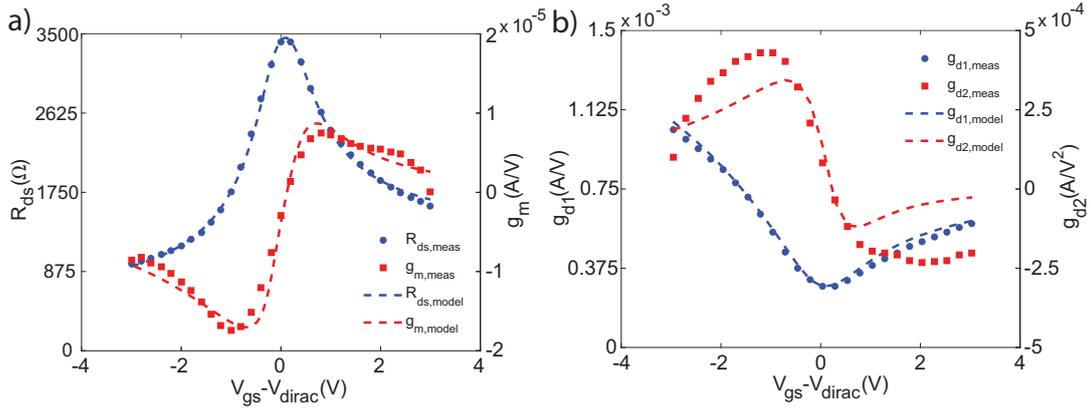
**Fig. 3.14:** Comparison of measured and modelled a) transfer characteristics, transconductance and b) drain current derivatives w.r.t. the drain voltage [Paper A].
