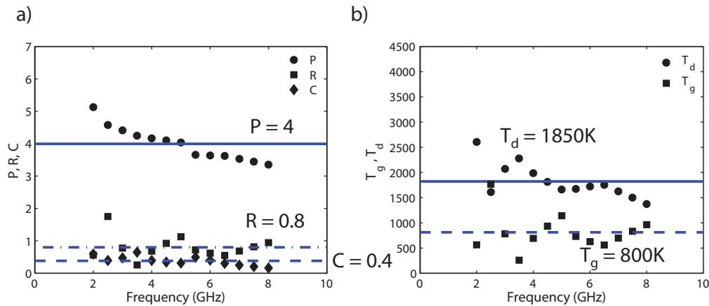
**Fig. 3.11:** a) Extracted  $P$  (●),  $R$  (■) and  $C$  (◆) coefficients of PRC model versus frequency. b) Extracted  $T_g$  (●) and  $T_d$  (■) of Pospieszalski model versus frequency. Lines and labels show mean values over all frequency points.
