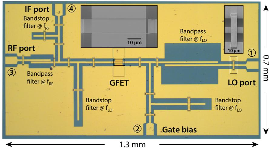
Fig. 4.7: The G-band subharmonic resistive GFET mixer IC reported in [Paper C].
