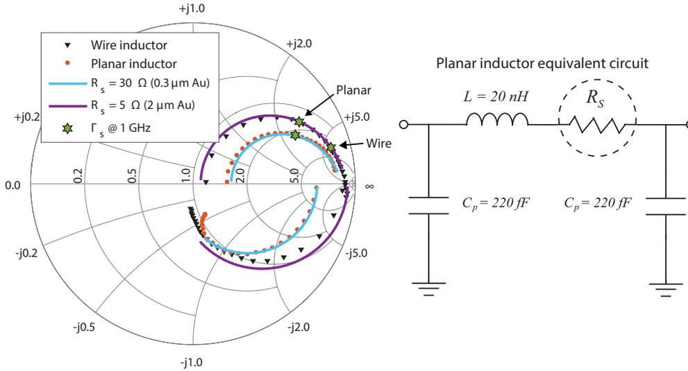
**Fig. 4.4:** Measured S-parameters up to 2 GHz for the surface mount wire inductor ( $L = 36 \text{ nH}$  from the datasheet) [Paper E] and the planar inductor ( $L = 20 \text{ nH}$  from the extracted equivalent circuit) [96]. A simulated planar inductor with thicker gold is included for comparison. The models were verified by EM simulation.
