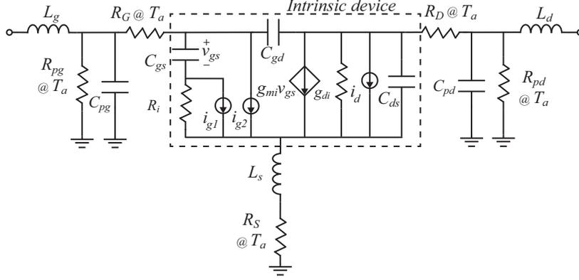
**Fig. 3.9:** Small-signal circuit for the GFET noise model at a given bias, with the Pospieszalski ( $i_{g1}$ ,  $i_d$ ) [113] and PRC ( $i_{g2}$ ,  $i_d$ ) [114] noise currents [Paper F].
