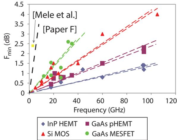
**Fig. 3.12:** Intrinsic  $F_{min}$  of the GFET with  $L_g = 1 \mu\text{m}$  [Paper F] compared with Si and III-V technologies [123], and the SiC GFET result for a  $L_g = 150 \text{ nm}$  device [124].
