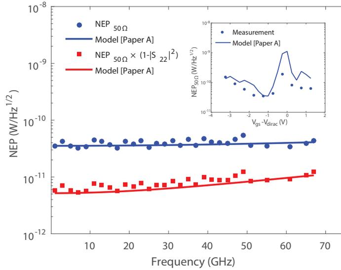
**Fig. 4.14:** The Volterra model agreement of NEP for a GFET ( $L_g = 0.5 \mu\text{m}$  and  $W_g = 2 \times 1.25 \mu\text{m}$ ) versus frequency and gate voltage (in the inset) [Paper A].
