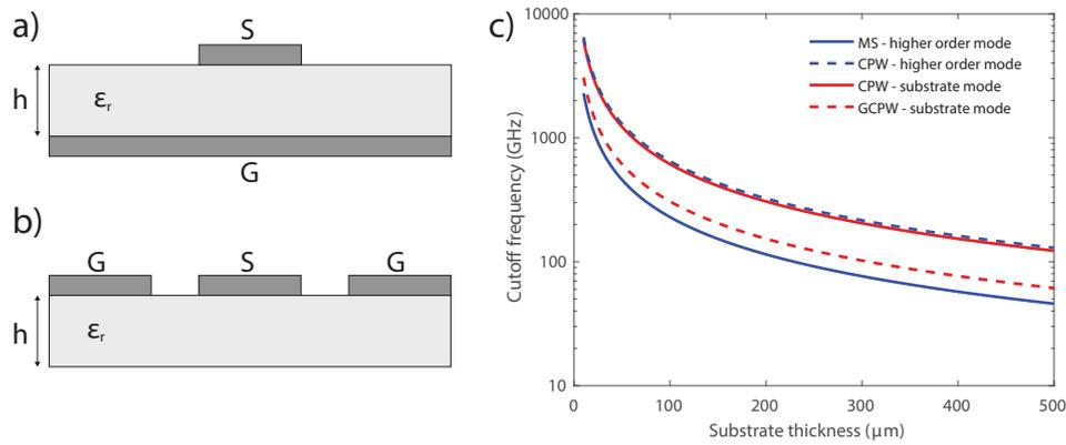
**Fig. 4.1:** Cross-sections of the a) microstrip (MS) and b) coplanar waveguide (CPW). c) Comparison of cutoff frequencies on Si for the first higher-order modes on MS and CPW. The lowest-order substrate mode for CPW is also shown [136,137].
