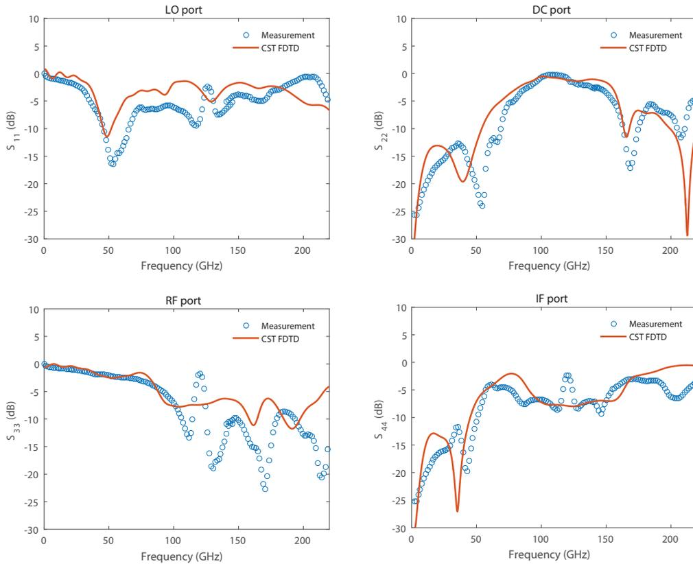
Fig. 4.8: Reflection S-parameters of the airbridged four-port CPW mixer circuit.
