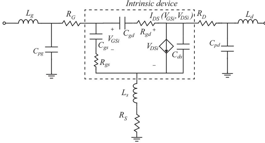
**Fig. 3.13:** Nonlinear representation of an FET using an equation-based description for the current source. The embedding circuit is assumed to be linear [Paper A].
