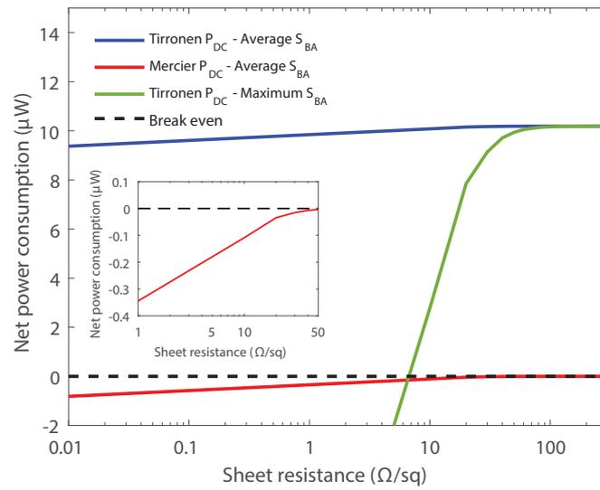
**Fig. 4.15:** The net power consumption of the transceiver assuming a single data transmission event per day [Paper 1]. Energy is harvested in the communication frequency bands around 2 GHz using a graphene dipole antenna.
