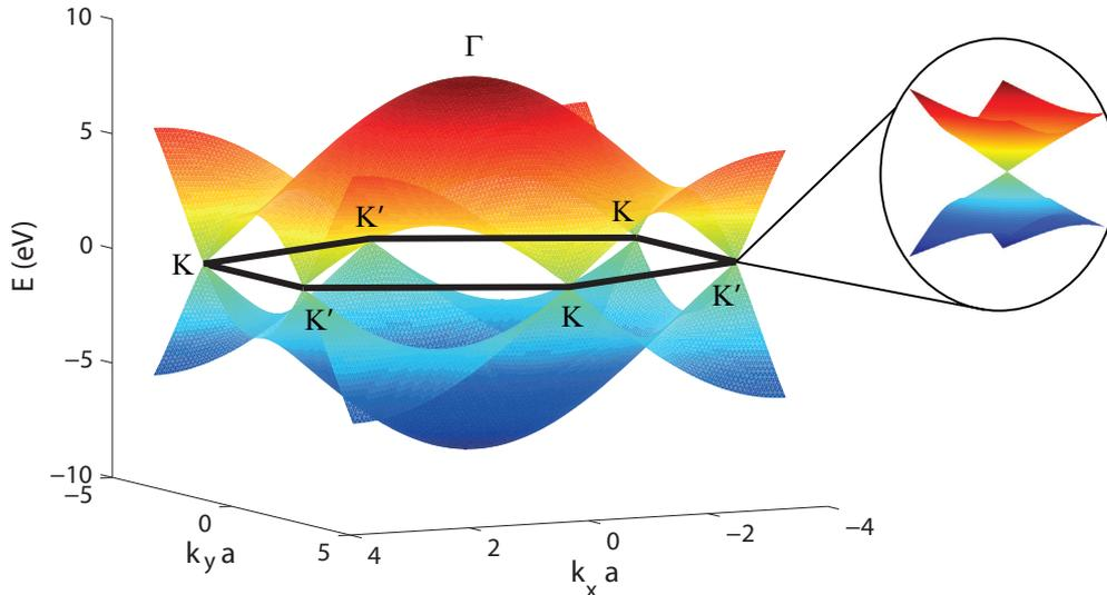
**Fig. 2.2:** Band structure of graphene in the tight binding approximation within the 1st Brillouin zone (Eq. 2.1). Inset shows the famous Dirac cone (Eq. 2.2).
