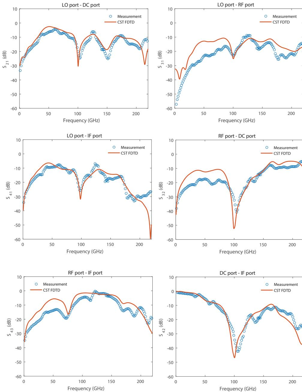
**Fig. 4.9:** Transmission S-parameters of the airbridged four-port CPW mixer circuit.
