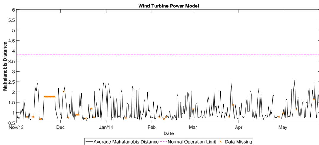
Figure A.7: Application of ANN based CMS to Turbine 4
