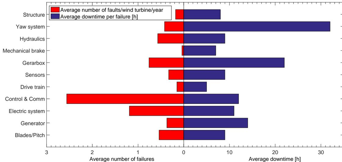
Figure 3.2: The average number of failures and downtime per failure for different subsystems for the wind turbine population under consideration
