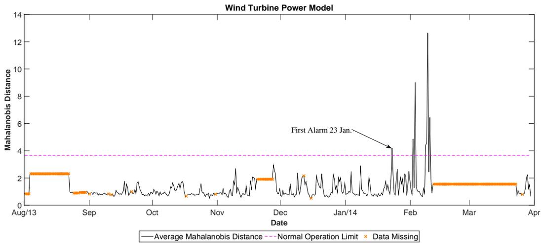
Figure A.2: Application of ANN based CMS to Turbine 1
