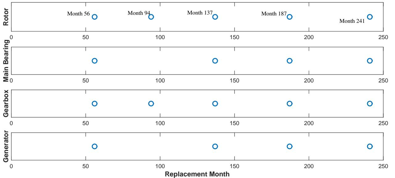
Figure 5.1: An optimal ABPM schedule from the PMSPIC model
