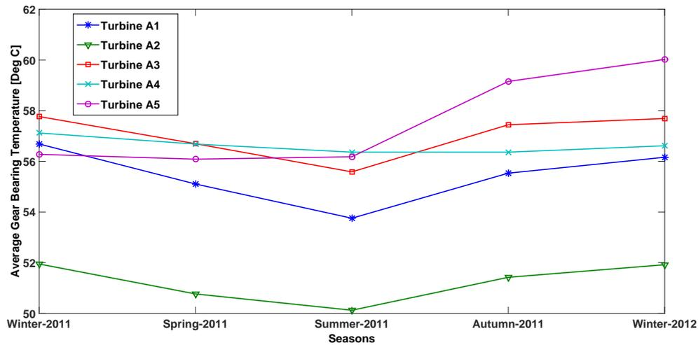
Figure 4.11: Seasonal average gearbox bearing temperatures for five wind turbines in a wind farm
