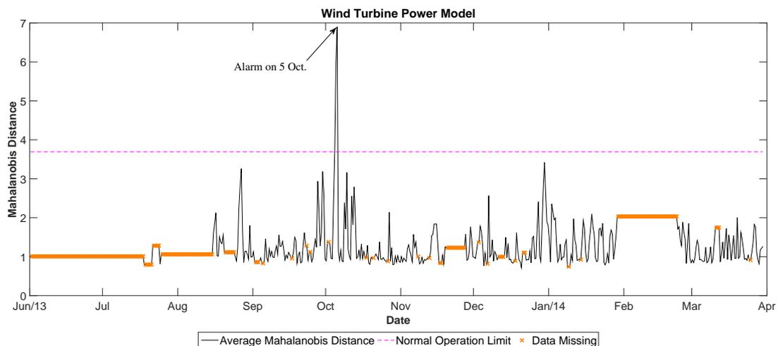
Figure A.4: Application of ANN based CMS to Turbine 3
