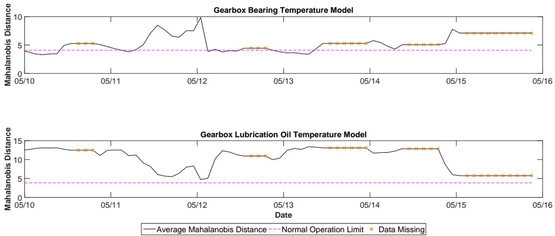
Figure A.10: Application of ANN based CMS to data with 10-sec. average values for Turbine 5
