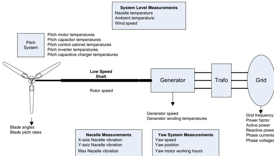
Figure A.1: Schematic representation of data from Direct Drive wind turbine.
