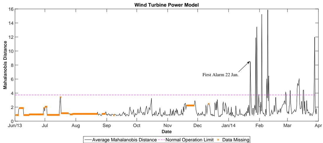
Figure A.3: Application of ANN based CMS to Turbine 2
