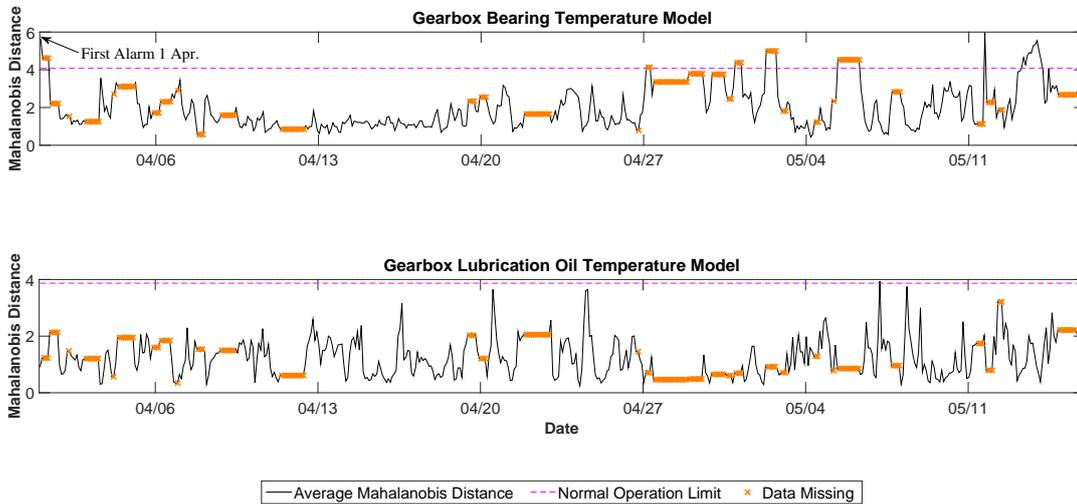
Figure A.9: Application of ANN based CMS to Turbine 5
