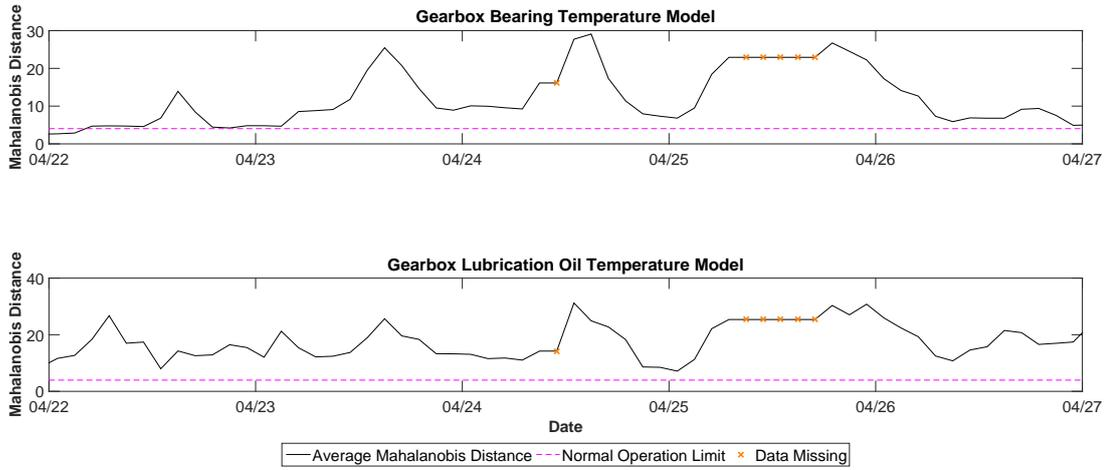
Figure A.13: Application of ANN based CMS to data with 10-sec. average values for Turbine 6
