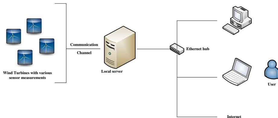
Figure 4.1: A schematic representation of a typical SCADA system for wind turbines
