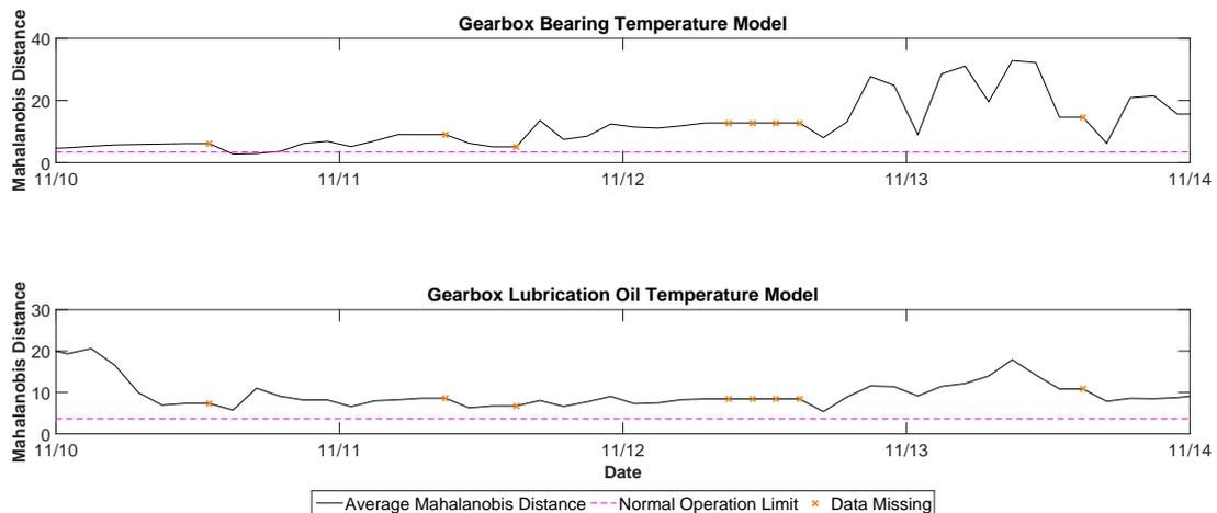
Figure A.16: Application of ANN based CMS to data with 10-sec. average values for Turbine 7
