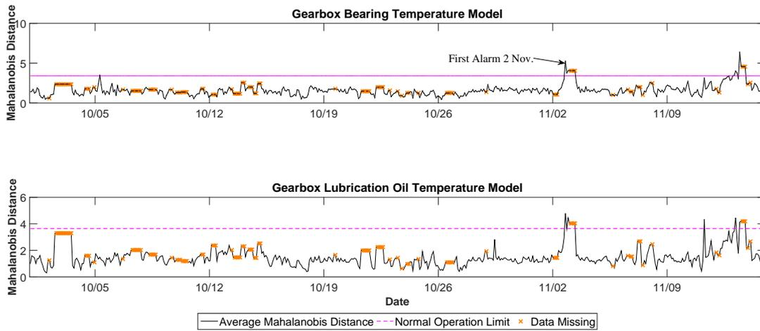
Figure A.15: Application of ANN based CMS to Turbine 7
