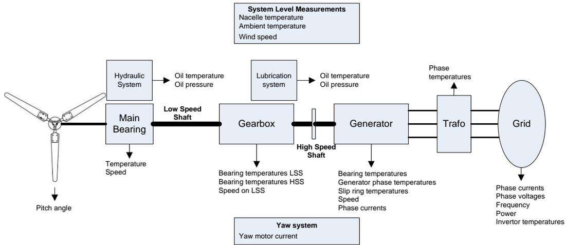
Figure A.8: Schematic representation of data from In-direct Drive wind turbine
