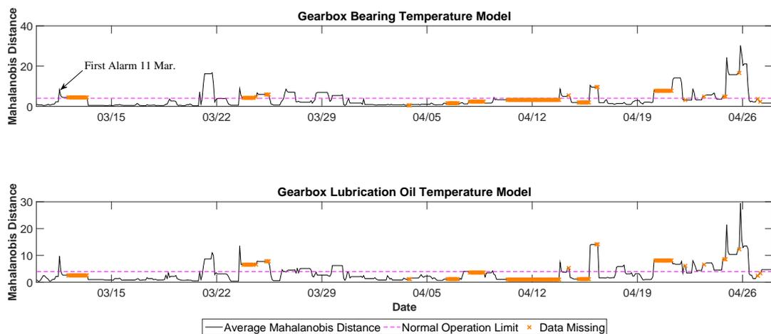
Figure A.12: Application of ANN based CMS to Turbine 6
