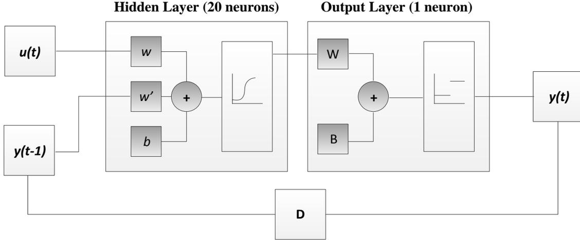
Figure 4.3: A schematic representation of the NARX ANN model configuration
