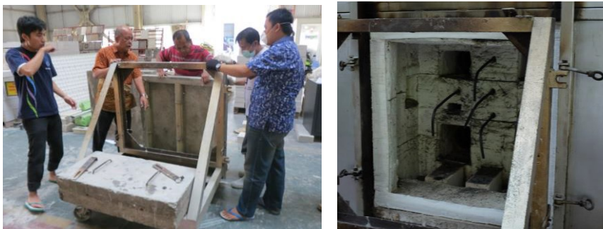
Picture 5: Specimen installation and furnace at [37]
