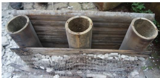
Picture 9: Removal of protective cover to assess bamboo cross-section after fire (left)
