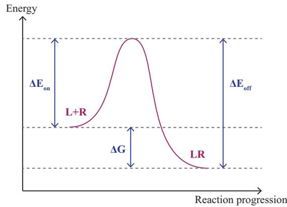
Figure 3.2: Arrhenius plot: The reaction constants for association and dissociation can be related to the activation energies for both processes and thus to the Gibbs free energy according to equations 3.4 and 3.5.
