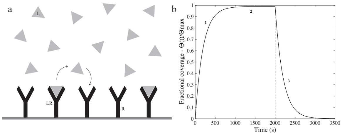
Figure 3.3: Illustration of the Langmuir model. a) Ligands in solution bind to and release from receptors immobilized on a surface. b) The fractional coverage expressed as a function of time can be divided into three parts: 1. Ligands binding to an empty surface 2. Equilibrium conditions (total rate of change is zero) 3. Exponential decay of bound ligands during rinsing step (no ligands in bulk solution).
