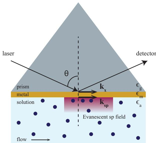
Figure 4.1: Working principle of SPR using the Kretschmann configuration. A thin metal film coated onto the backside of a glass prism is illuminated with a laser beam in total internal reflection. At a certain angle, surface plasmon resonance is achieved and an evanescent field is created at the metal/solution interface. A change in refractive index upon binding of molecules to the surface will result in a change of resonance angle.
