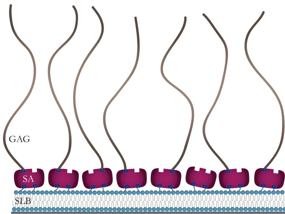
Figure 5.1: End-on immobilization of glycosaminoglycan chains onto a sensor surface via biotin/streptavidin to create a brush-like architecture. The streptavidin molecules are bound to a supported lipid bilayer containing a fraction of biotinylated lipids.
