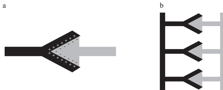
Figure 3.1: Illustration of the concept of specificity and multivalency. a) Non-directional forces can achieve high specificity if the three-dimensional arrangement is in favor of the interaction. b) Multivalent interactions can be collectively stronger than the separate monovalent interactions they are composed of.
