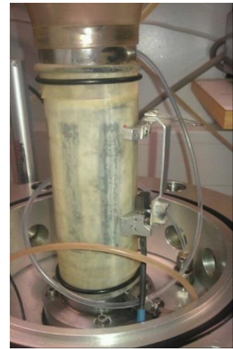
Figure A6.3 (a) Comparison of local vertical strains during shearing using the Hall effect device and external measurement using LVDT (b) 70 mm Hall effect gauge side view
