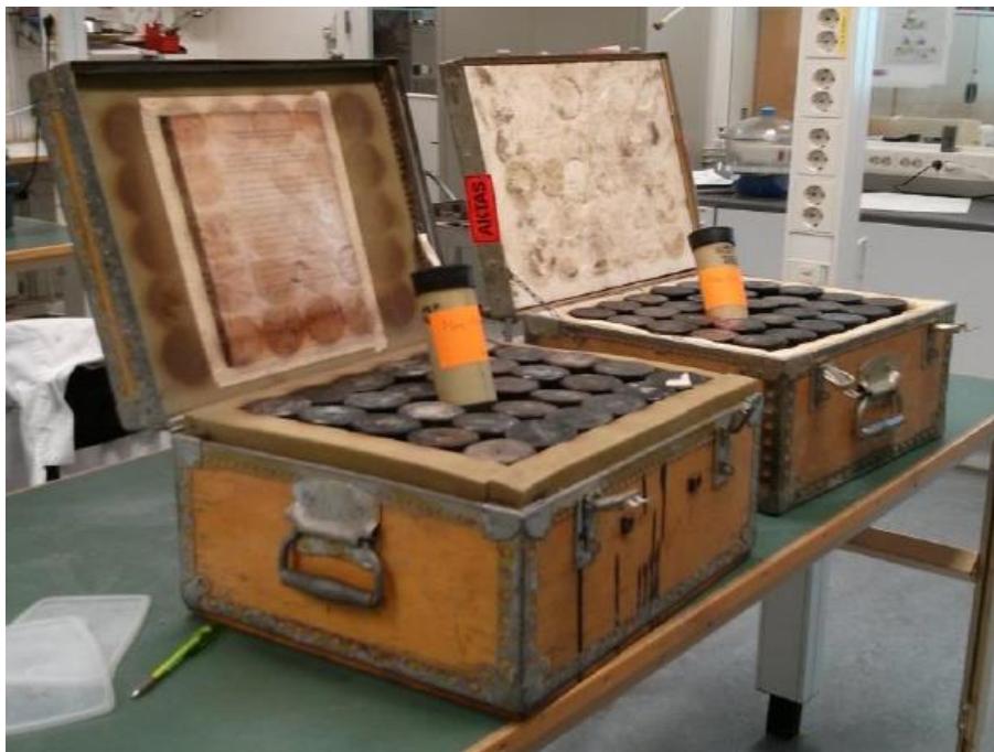
Figure 3.21 Sample transport boxes used in town driving vibration test lined with foam or polystyrene.
