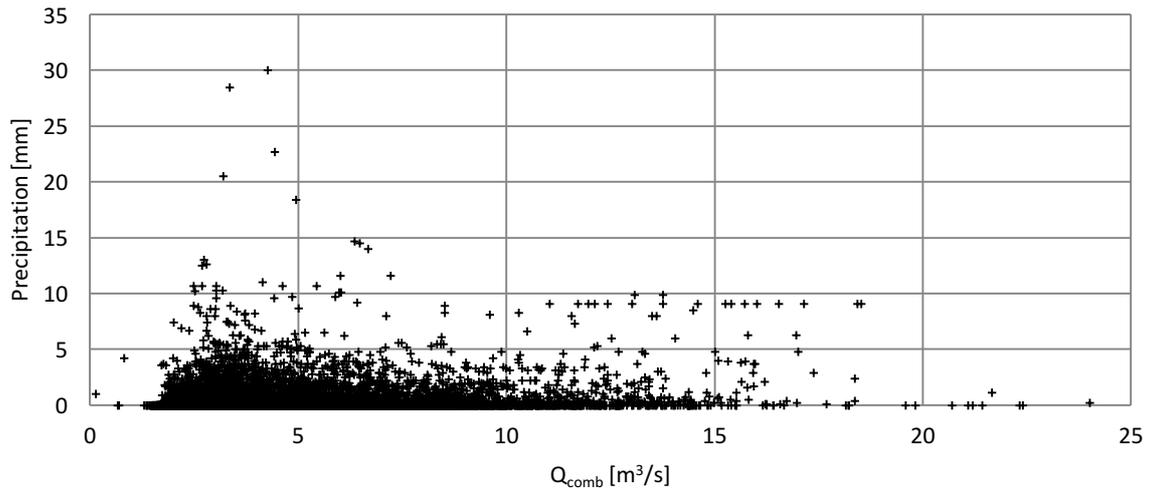
**Figure 4-13 Flow vs. precipitation 2005 - 2015 (hourly)**
