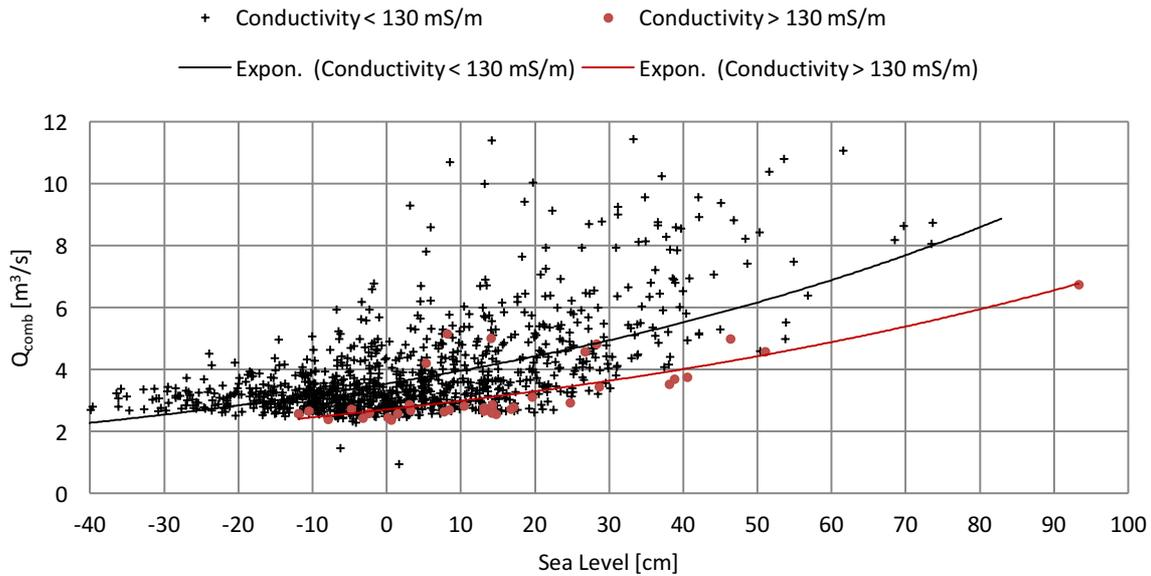
**Figure 4-9 Daily sea level vs.  $Q_{comb}$  at different conductivity conditions**
