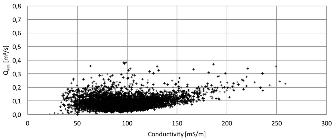
**Figure 4-18 Calculated  $Q_{\text{sea}}$  vs. conductivity 2005 – 2015 (six hourly average)**
