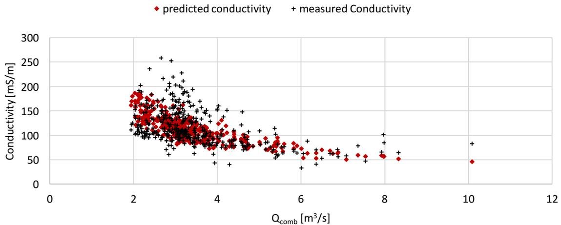
Figure 5-12  $Q_{comb}$  vs. predicted and measured conductivity (April till June 2011)
