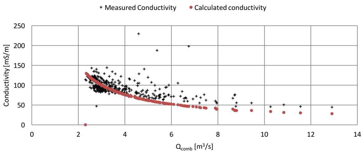
**Figure 4-16 Measured (daily average) and calculated conductivity summer 2013**
