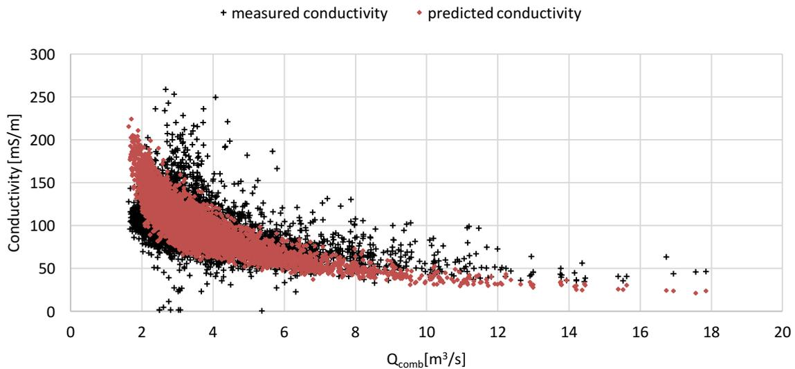
**Figure 5-2  $Q_{\text{comb}}$  vs. predicted and measured conductivity (6h averages) 2005 - 2015**
