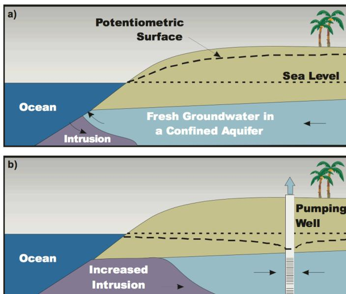
Figure 2-1 Seawater intrusion (Johnson 2007)
