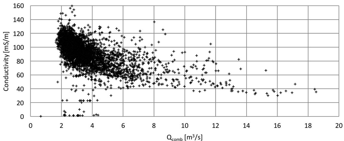
**Figure 4-12 Hourly flow vs. conductivity summer 2010**
