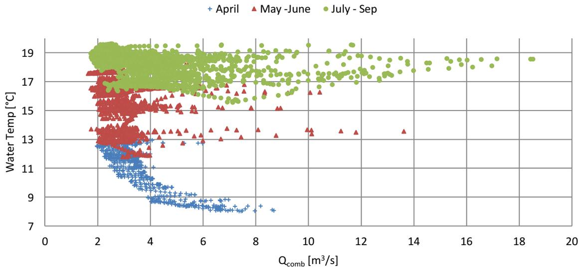
**Figure 4-11 Hourly flow vs. water temperature for different periods of the year summer 2010**
