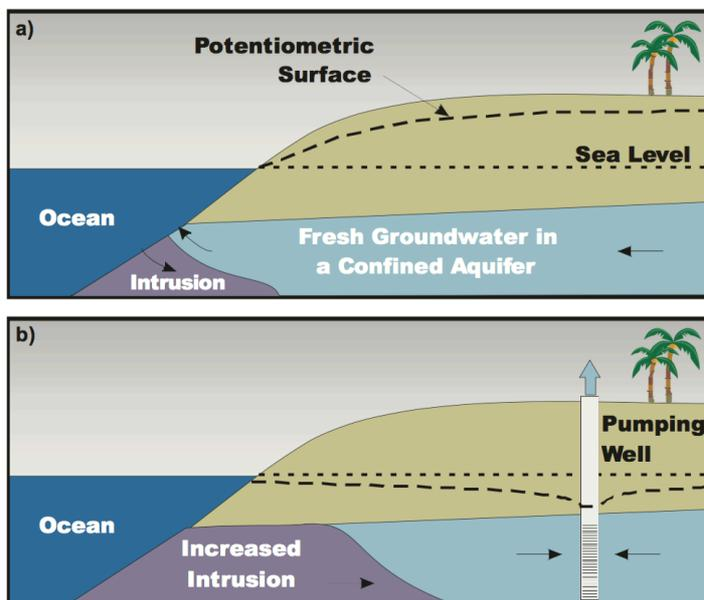
Figure 2-1 Seawater intrusion (Johnson 2007)
