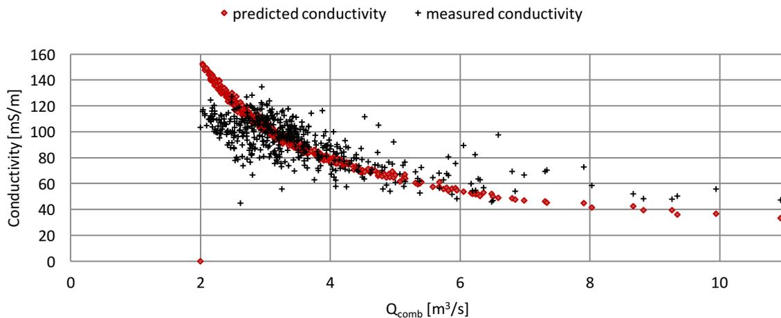
**Figure 5-7  $Q_{comb}$  vs. measured and predicted conductivity (6h average) April till July 2014**
