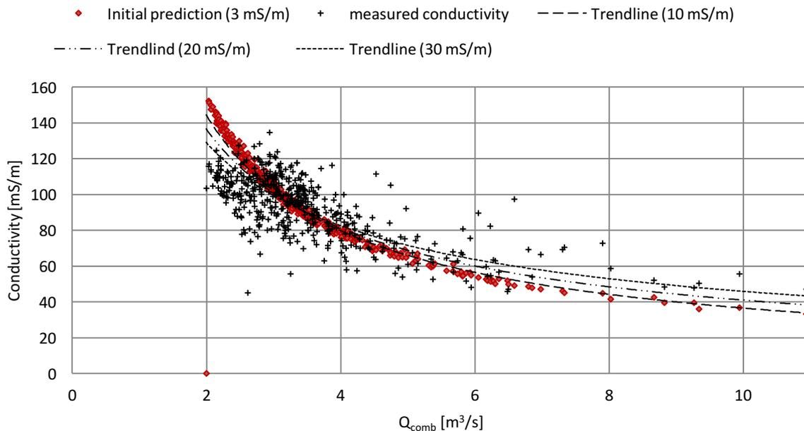
**Figure 5-16**  $Q_{\text{comb}}$  vs. conductivity for different  $\sigma_f$
