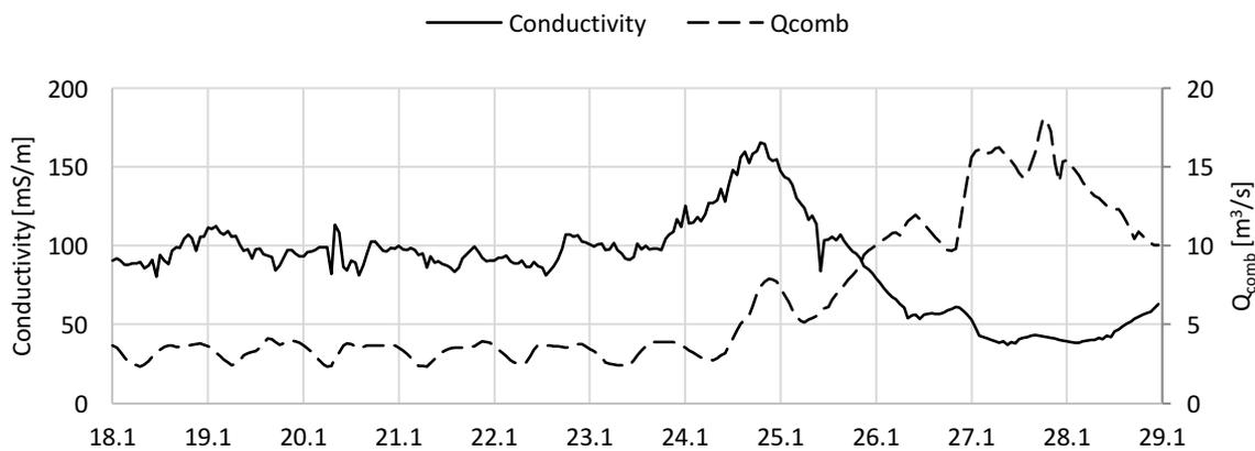
**Figure 4-6 Conductivity and  $Q_{comb}$  18.1.16 - 28.1.16 (hourly)**
