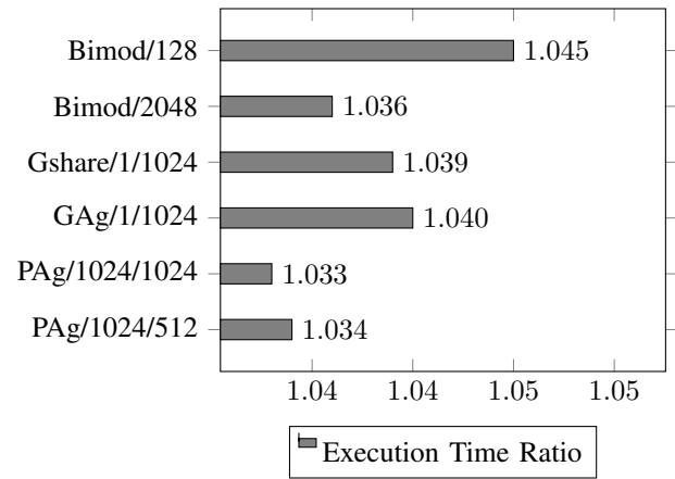
Fig. 2. Execution time ratio of different branch predictors obtained using the SPEC benchmark suite.
