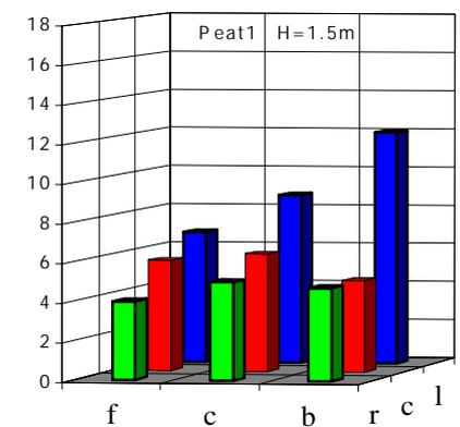
**Fig. 3.2.2.2** Oxygen concentration (%) in furnace cross-section at 1.5, 3.7, 5.4 and 9.9 meter during the Wood1 test. Input data: [Fig322\\_2.xls](#)
