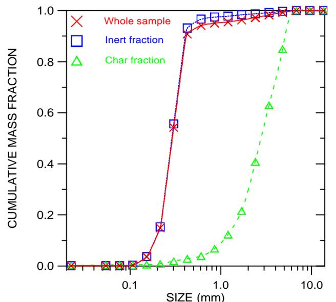
**Fig. 3.3.3.1** Cumulative mass fractions of the whole sample, the char fraction and the inert fraction. Sample taken during the Coal1 test from hole H2 (H=0.56 meter) in the combustion chamber. Input data: [Fig333\\_1.xls](#)
