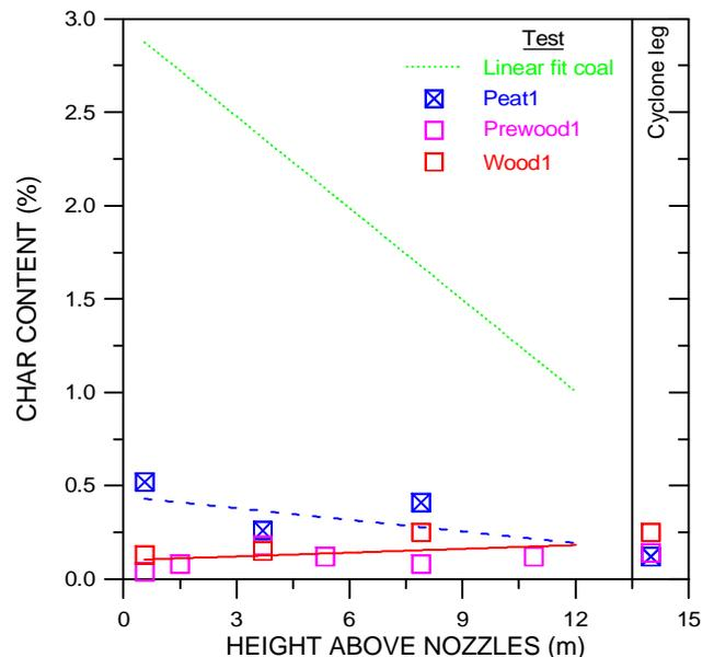
**Fig. 3.3.6.1** Comparison of the char concentrations in solid samples taken in the combustion chamber during the tests: Peat1, Wood1 and Prewood1. Dotted line adopted from Fig. 3.3.2.1. Input data: [Fig336\\_1.xls](#)
