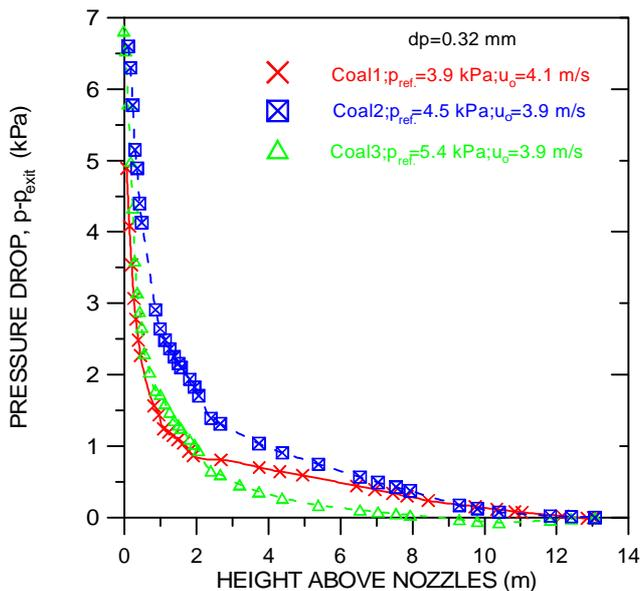
**Fig. 3.3.1.1** Vertical pressure drop profiles in the combustion chamber for the three coal tests. Input data: [Fig331\\_1.xls](#)
