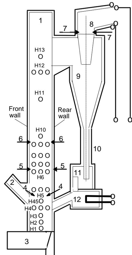
**Fig. 2.1.1** The 12-MW<sub>th</sub> CFB boiler at Chalmers University of Technology (1) combustion chamber; (2) fuel feed chute; (3) air plenum; (4) secondary air inlet at 2.1m; (5) secondary air inlet at 3.7m; (6) secondary air inlet at 5.4m; (7) secondary air inlet into cyclone exit duct; (8) cyclone exit duct (9) cyclone; (10) particle return leg; (11) particle seal; (12) heat exchanger. Measurement ports (H1 to H13) on the right boiler wall are indicated.
