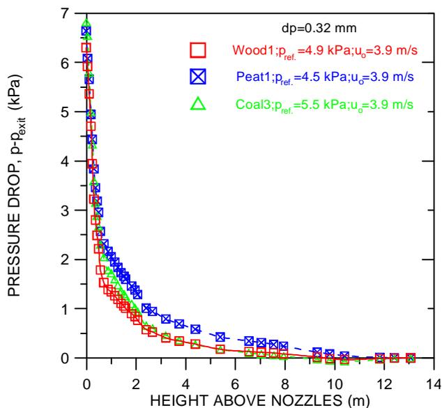
**Fig. 3.3.5.1** Vertical pressure drop profiles in the combustion chamber for the tests Coal3, Peat1 and Wood 1 tests. Input data: [Fig335\\_1.xls](#)
