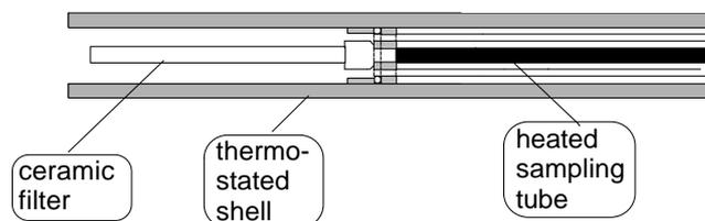
**Fig. 2.2.2** Front part of the gas sampling probe.
