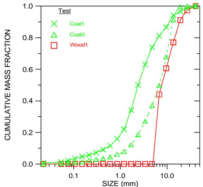
**Fig. 2.5.1** Cumulative mass fractions of fuel samples taken from the belt weighters during the Coal1, Coal3 and Wood1 measurement. Input data: [Fig2\\_5\\_1.xls](#)
