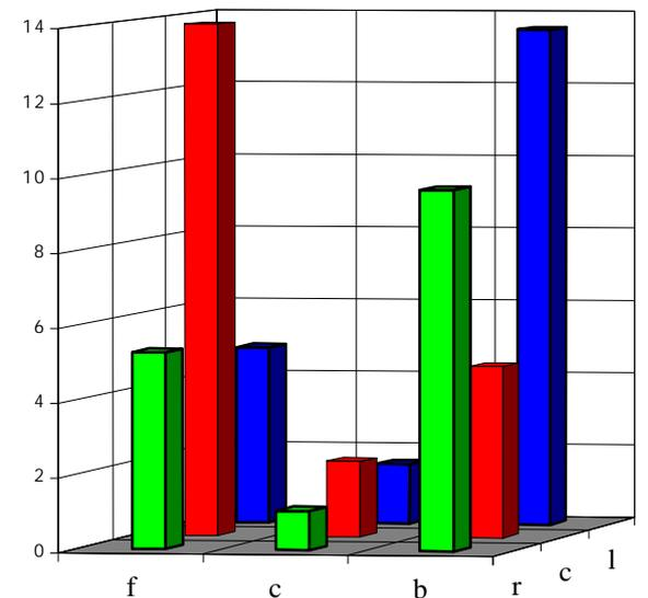
**Fig. 3.2.1.3** Oxygen concentration (%) in furnace cross-section at 9.9 meter (top) and 3.7 meter height (bottom) during the Coal2 test. Input data: [Fig321\\_3.xls](#)
