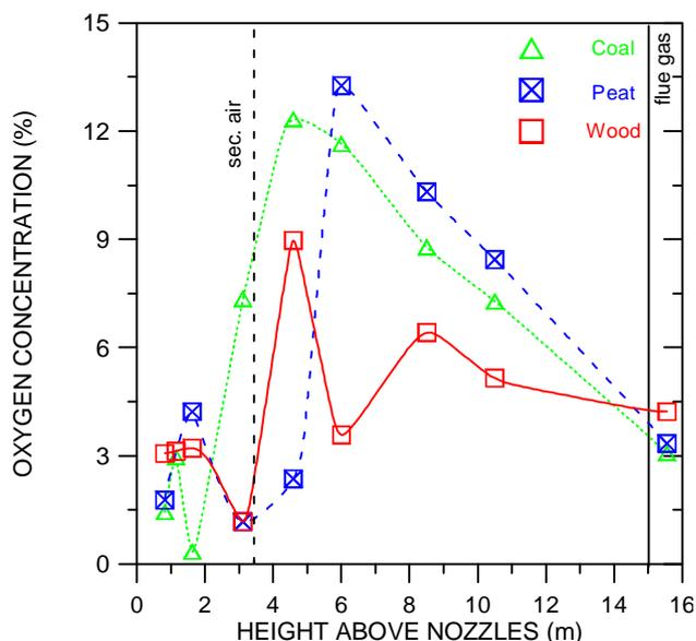
**Fig. 4.1.1** Vertical cross-section averaged profiles of oxygen in the combustion chamber of a lab-scale CFB burning coal, peat and wood. Input data: [Fig4\\_1\\_1.xls](#)
