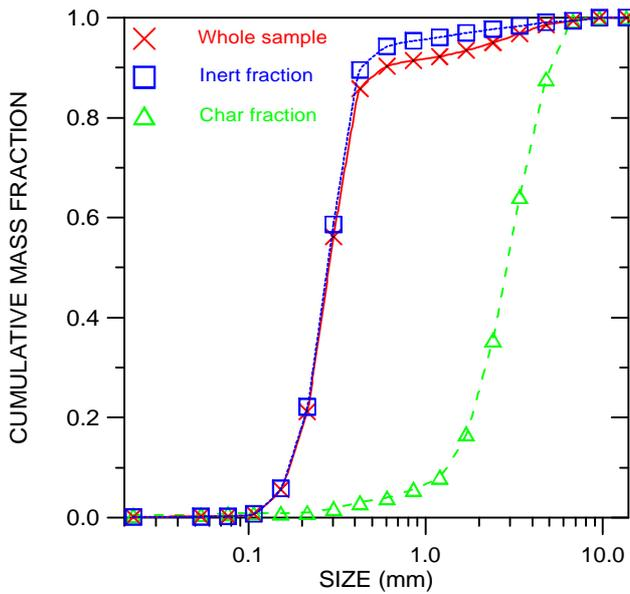
**Fig. 3.3.3.2** Cumulative mass fractions of the whole sample, the char fraction and the inert fraction. Sample taken during the Coal3 test from hole H2 (H= 0.56 meter) in the combustion chamber. Input data: [Fig333\\_2.xls](#)
