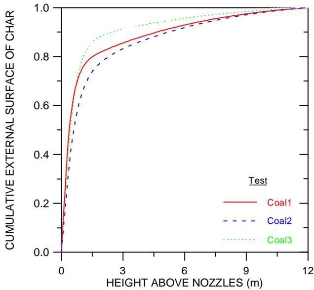
**Fig. 3.3.4.2** Cumulative external surface of char in the combustion chamber as function of height for the tests: Coal1, Coal2 and Coal3. Input data: [Fig334\\_2.xls](#)
