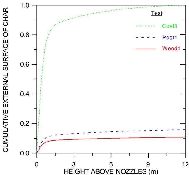
**Fig. 3.3.7.2** Cumulative external surface of char in the combustion chamber as function of height for the tests: Coal3, Peat1 and Wood1. Data for Peat1 and Wood1 normalised to the amount obtained for the Coal3 test. Input data: [Fig337\\_2.xls](#)
