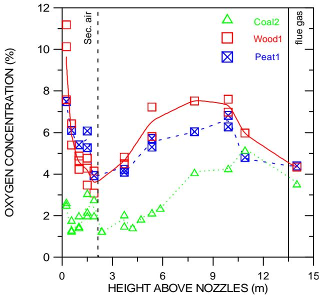
**Fig. 3.2.2.1** Vertical profiles of oxygen along the centre line in the combustion chamber for the tests Coal2, Peat1 and Wood1. Input data: [Fig322\\_1.xls](#)
