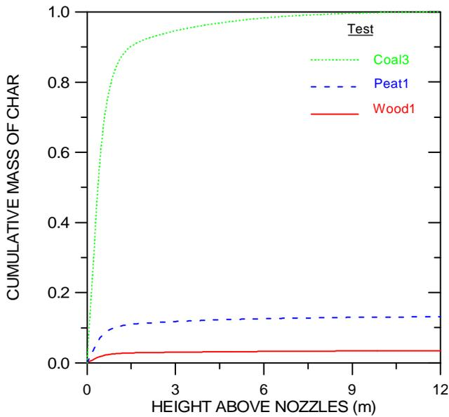
**Fig. 3.3.7.1** Cumulative mass of char in the combustion chamber as function of height for the tests: Coal3, Peat1 and Wood1. Data for Peat1 and Wood1 normalised to the amount obtained for the Coal3 test. Input data: [Fig337\\_1.xls](#)
