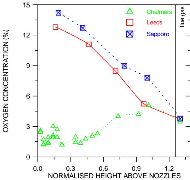
**Fig. 4.1.2** Comparison of the vertical profiles of oxygen along the centre line in the combustion chamber between the Chalmers boiler and two lab-scale CFB test units. Fuel: Bituminous coal. Test conditions: See Table 4.1.1. Input data: [Fig4\\_1\\_2.xls](#)
