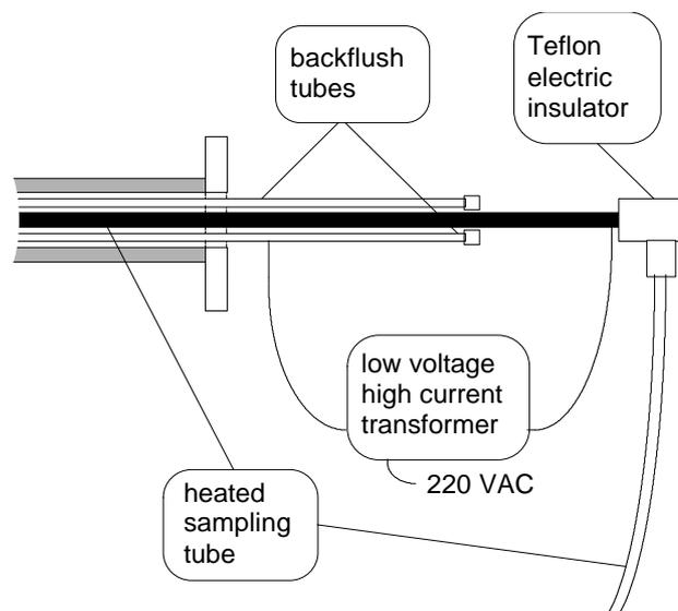
**Fig. 2.2.3** Rear part of the gas sampling probe.
