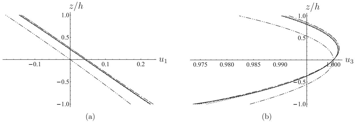
Fig. 1. Displacement in  $x$ -direction  $u_1$  (a) and  $z$ -direction  $u_3$  (b) for the first mode with  $p = 3$ : ---  $N = 50$ , ---  $N = 10$ , - - -  $N = 6$ , - - - -  $N = 4$ , ...  $N = 3$ , -.-  $N = 2$ .
