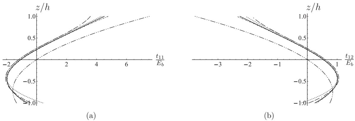
Fig. 2. Normal stress in  $x$ -direction  $t_{11}$  (a) and shear stress  $t_{12}$  (b) for the fundamental eigenfrequency,  $p = 3$ : ---  $N = 50$ , ---  $N = 10$ , - - -  $N = 6$ , - - - -  $N = 4$ , ...  $N = 3$ , -.-  $N = 2$ .
