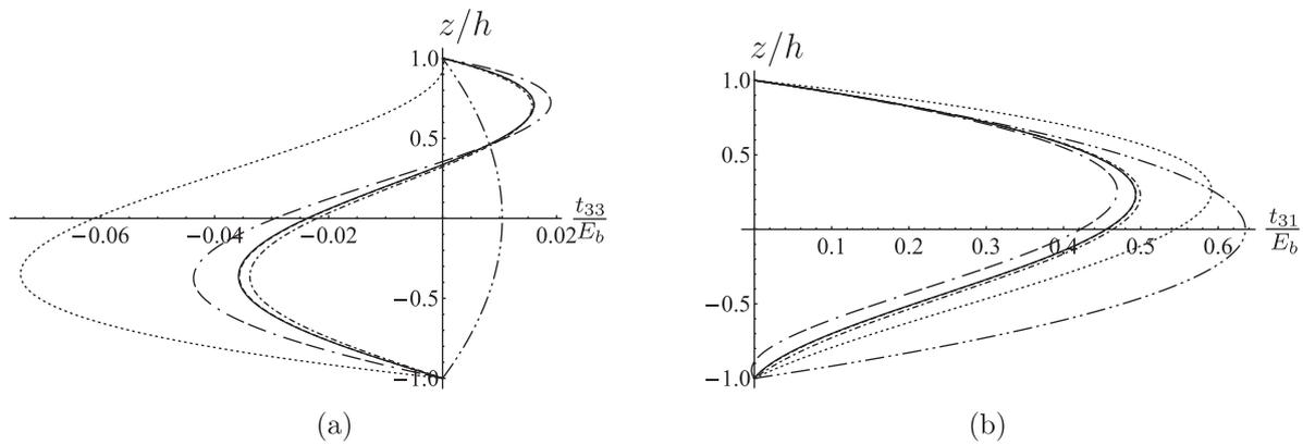
Fig. 3. Normal stress in  $z$ -direction  $t_{33}$  (a) and shear stress  $t_{31}$  (b) for the fundamental eigenfrequency,  $p = 3$ : ---  $N = 50$ , ---  $N = 10$ , - - -  $N = 6$ , - - - -  $N = 4$ , ...  $N = 3$ , -.-  $N = 2$ .
