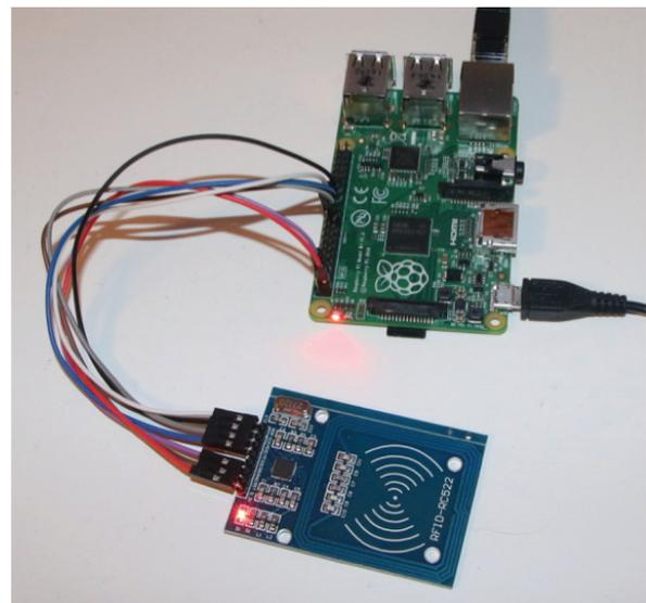
Fig. 3. A Raspberry Pi with the MFR522 board.
