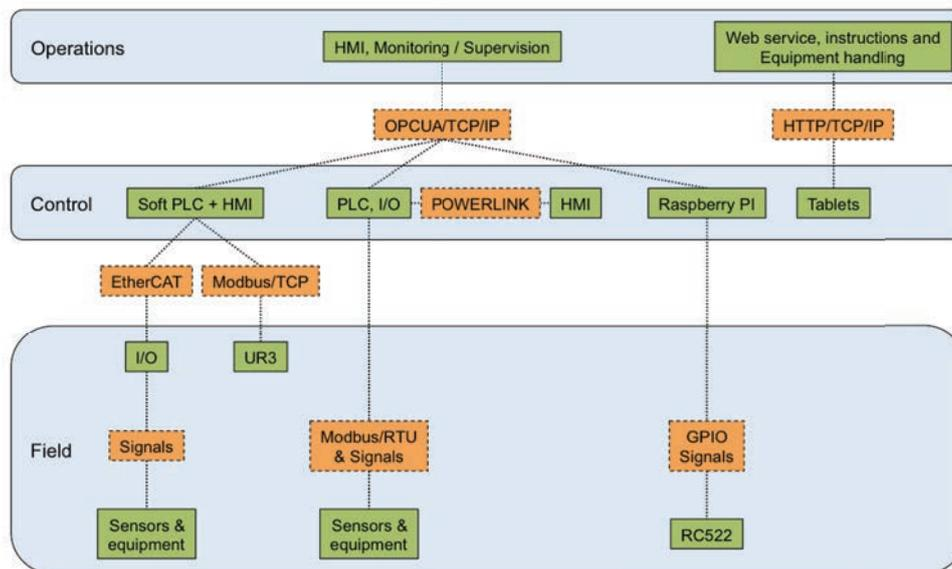
Fig. 4. System overview with equipment and communication protocols.
