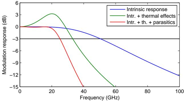
Fig. 4.1. Intrinsic and extrinsic modulation response extracted from the VCSEL used in Paper A with  $K$ - and  $D$ -factors of  $0.17 \text{ ns}$  and  $9.0 \text{ GHz}/\text{mA}^{1/2}$ , respectively, along with a parasitic pole,  $f_p \approx 17 \text{ GHz}$ .
