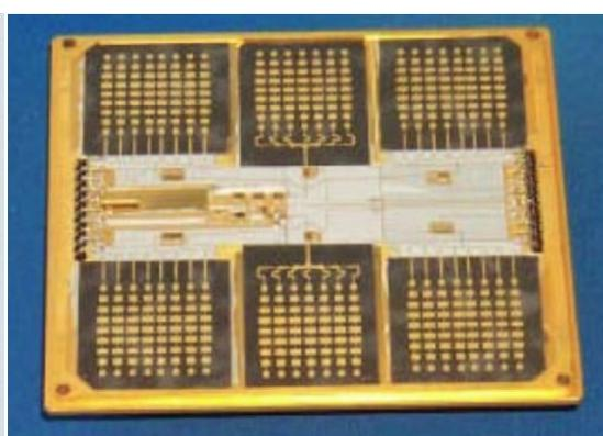
Figure 1.6 Photograph of ASTYX's 77 GHz radar sensor with microstrip patch antenna arrays [14]
