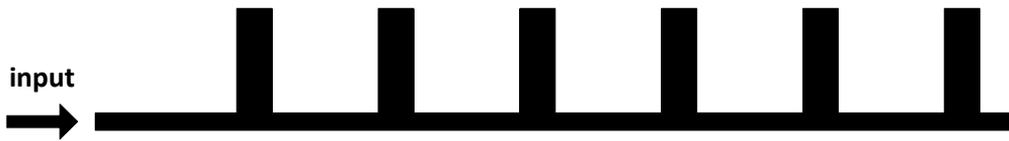
Figure 2.5 A microstrip comb-line antenna array composed of open-circuit stubs
