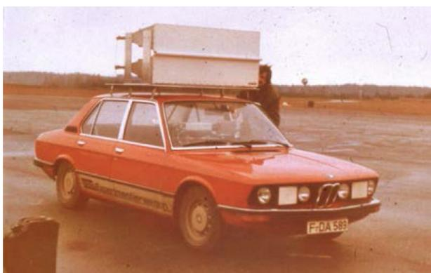
Figure 1.3 A 10 GHz automotive radar built in 1970s [11]
