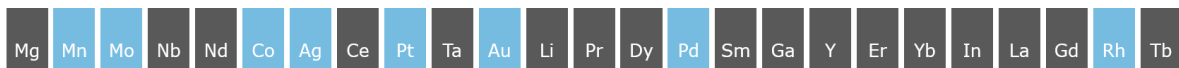
Figure 5. Scarce metals (in bright blue) for which potential for functional recycling is identified.
