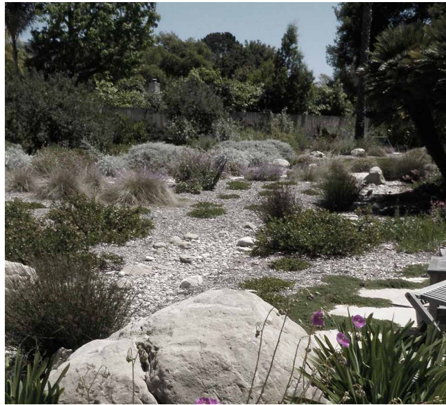
B. Bioswale is a ditch designed to delay and treat water. A dry bioswale can be used as a walking path (Wilson Environmental Contracting, n.d.).
