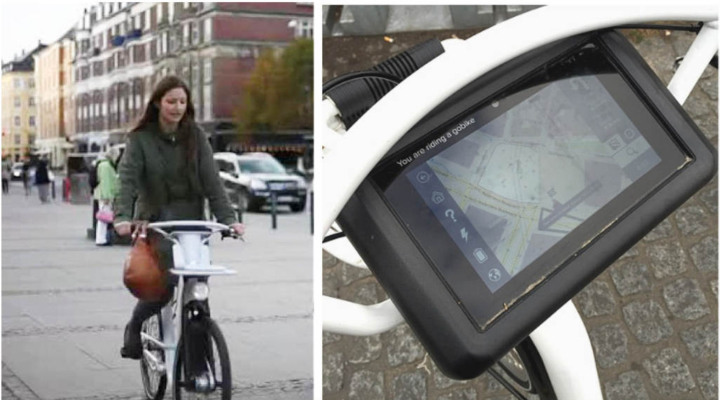
Figure 2.4: Map navigation interface displayed on tablet mounted under handlebars. Copenhagen City Bike, bycyklen.dk
