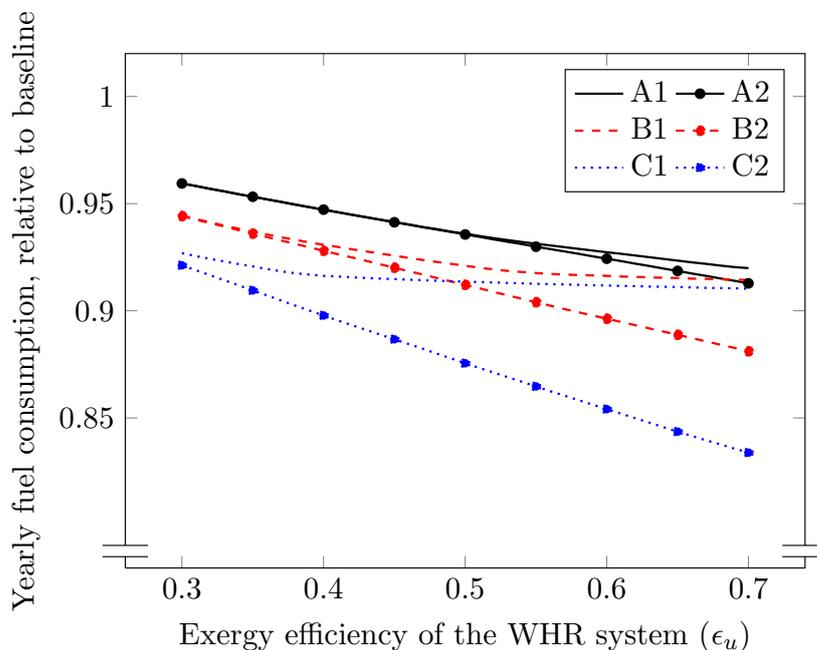
**Figure 5.6:** Calculated yearly fuel consumption with the installation of a WHR system on Ship-1, compared to baseline
