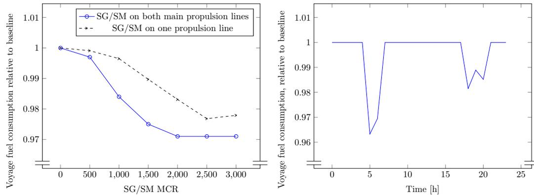
(a) Relative fuel consumption versus shaft generator/motor design power (b) Relative fuel consumption, effect of including heat demand in the optimisation<sup>1</sup>
