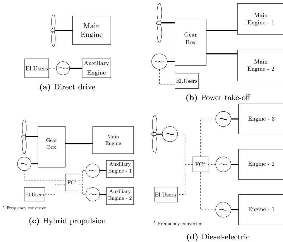
**Figure 2.4:** Schematic representation of alternative power system configurations
