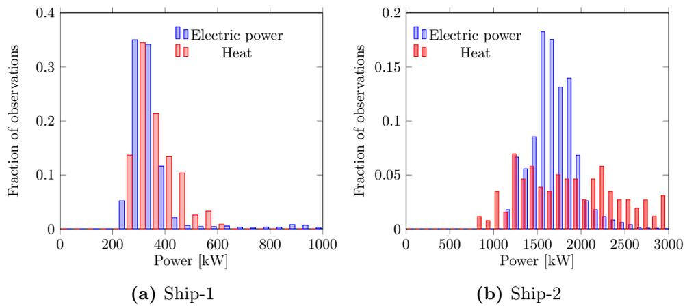
**Figure 5.2:** Case studies operational analysis: Auxiliary power distribution
