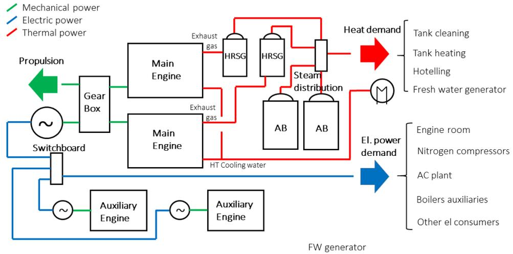
Figure 4.2: Conceptual representation of energy systems and flows of Ship-1
