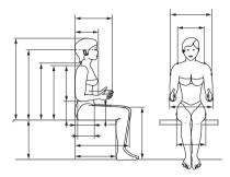
Figure 5 Structural dimensions in predefined static postures (University of Skövde, 2011)
