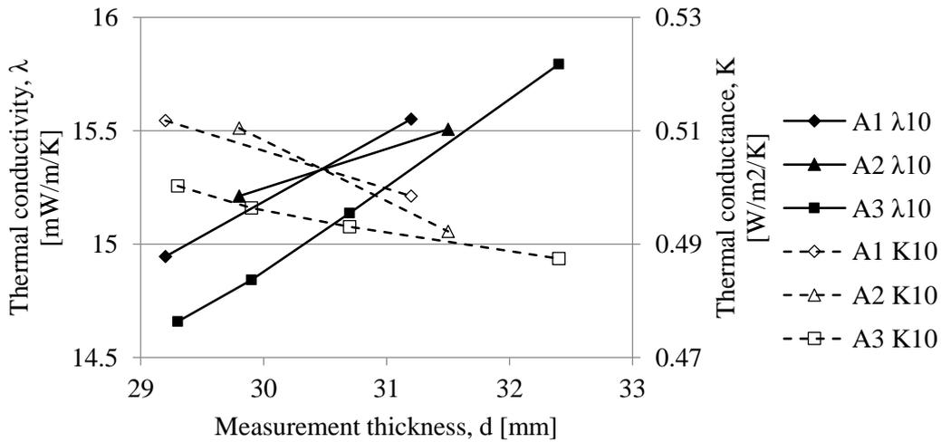
Figure 4.2: Relation between mechanical compression (measured as a thickness variation) and thermal conductivity for an aerogel blanket
