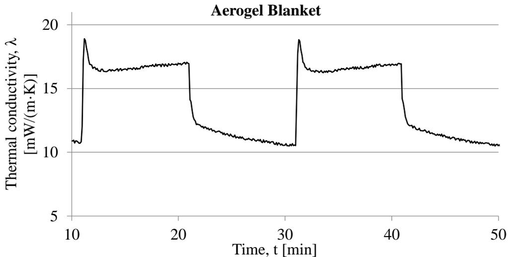
Figure 4.6: Measured thermal conductivity of an aerogel blanket at a varied pressure. The pressured was cycled between 2 kPa and atmospheric pressure at 20 min intervalls.
