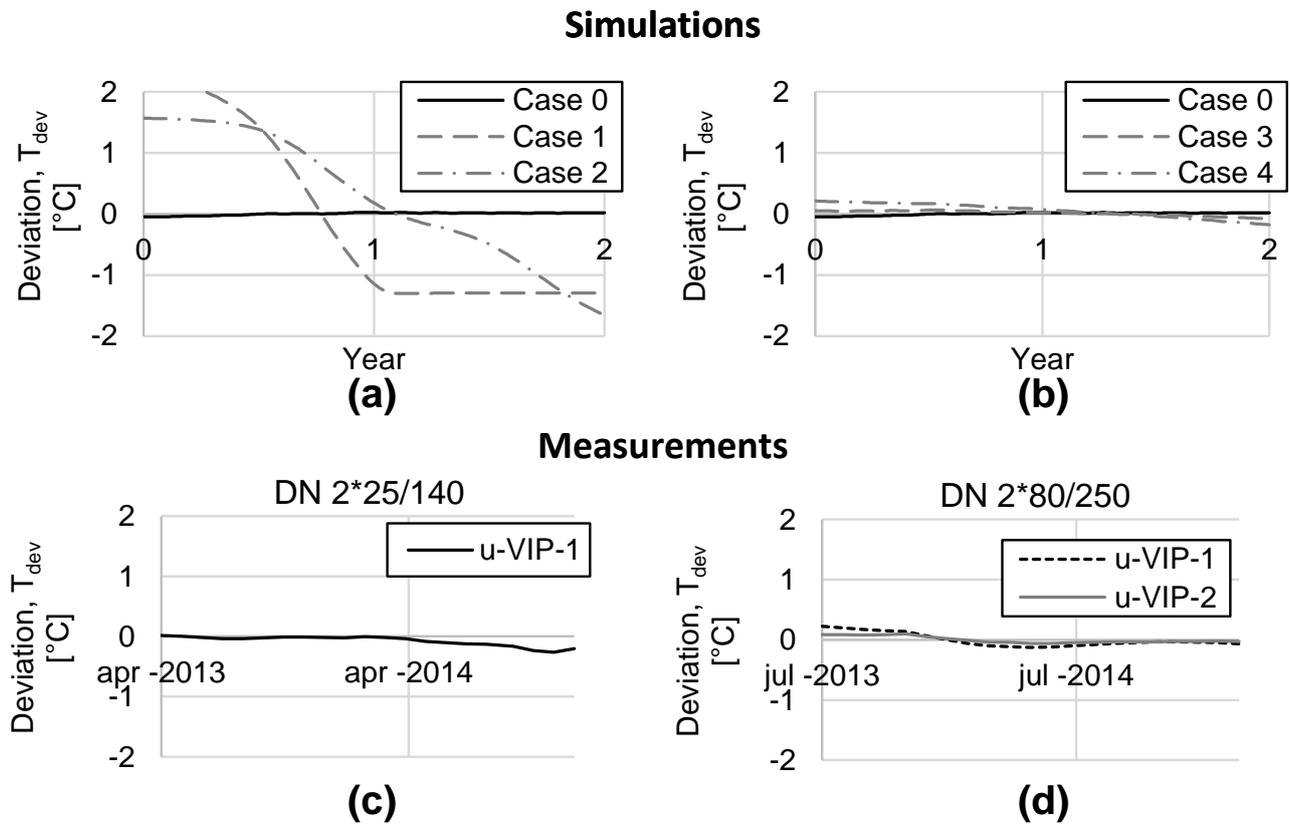
Figure 3.12: The resulting deviation between the superposition model and the results from measurements and simulations. The results from simulations are shown on top and the results from the measurements are shown at the bottom.
