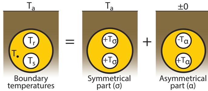
Figure 3.10: Description of the temperatures in the superposition model.
