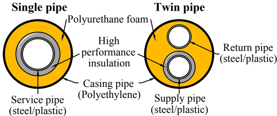
Figure 3.1: Concept for hybrid insulation district heating pipes.
