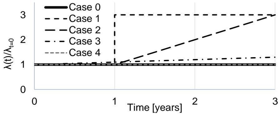
Figure 3.11: Description of how the thermal conductivity changes with time for the 5 simulation cases.
