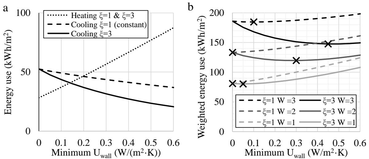
Figure 4.8: Effect of a variable U-value in an office building. In (a) the heating is compared to the cooling and in (since the minimum U-value have been used as baseline for the variation, the heating energy use is independent of the variation) (b) different weighting factors for the weighted relation between cooling energy and heating energy is presented.
