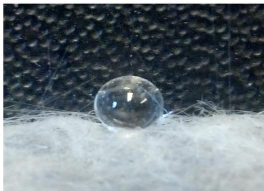
Figure 2.3: Water droplet on a hydrophobic aerogel blanket.
