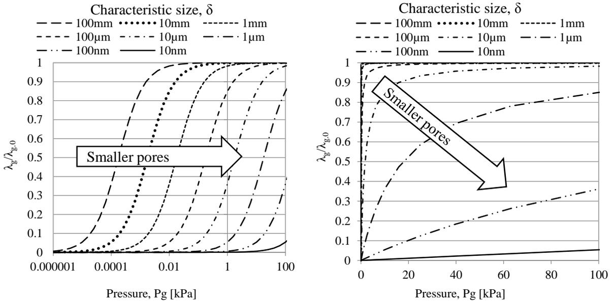
Figure 2.1: Principal figure of thermal conductivity through the air in a porous insulation for different pressures below atmospheric pressure (just above 100 kPa). To the left, the pressure axis is logarithmic and to the right the pressure axis is linear. The porosity of the material is assumed to be 1.
