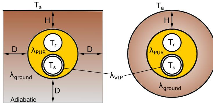
Figure 3.3: Description of the two dimensional simulation models with a square domain to the left and with a circular domain to the right.
