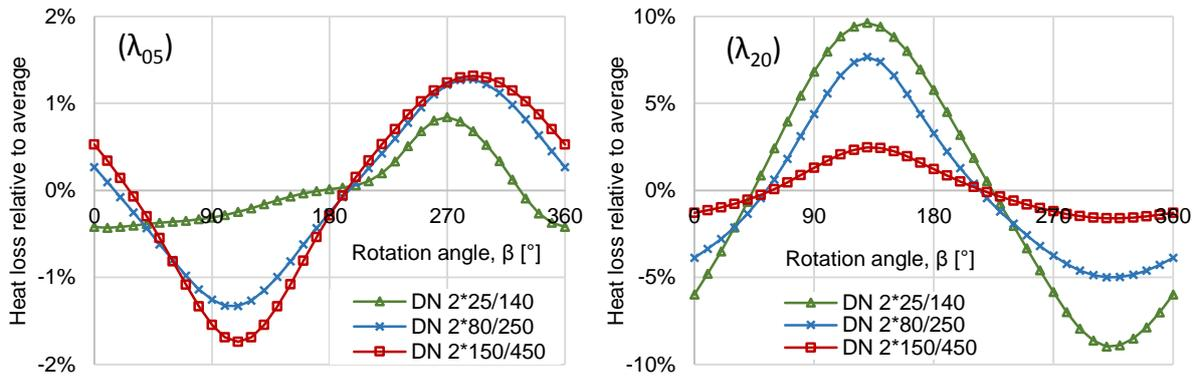
Figure 3.6: The heat loss relative to the average for a variation in the rotational position,  $\beta$  of the VIPs.
