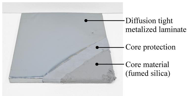
Figure 2.4: The layers of a vacuum panel with a fumed silica core.
