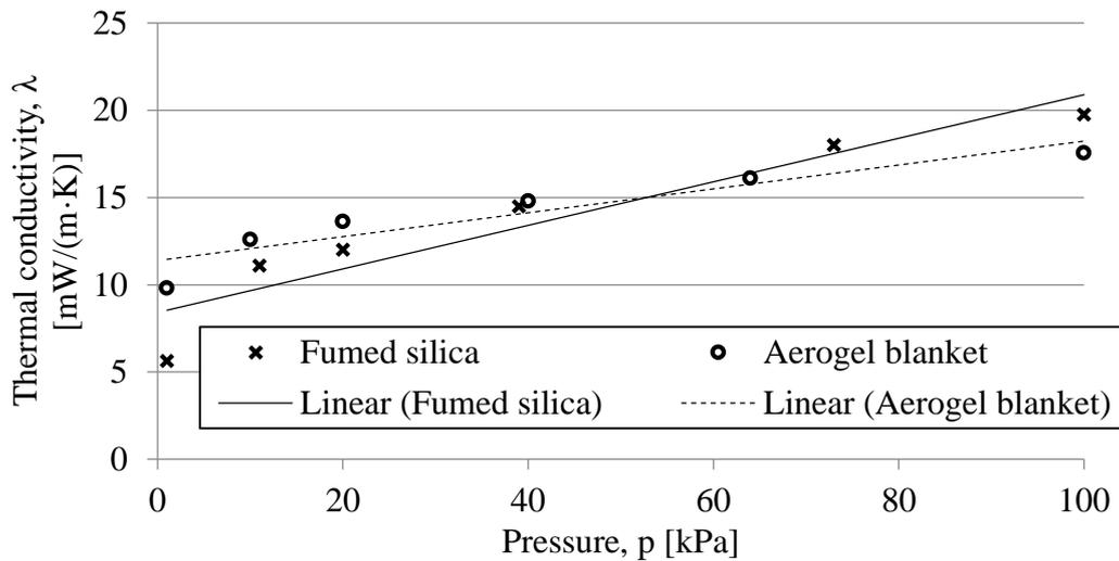
Figure 4.4: Relation between pressure and thermal conductivity for a fumed silica and an aerogel blanket
