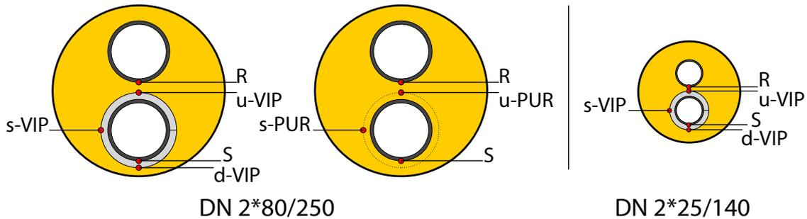
Figure 3.8: Position of thermocouples in the field measurement pipes. Each point is measured in at least two positions along the pipe.
