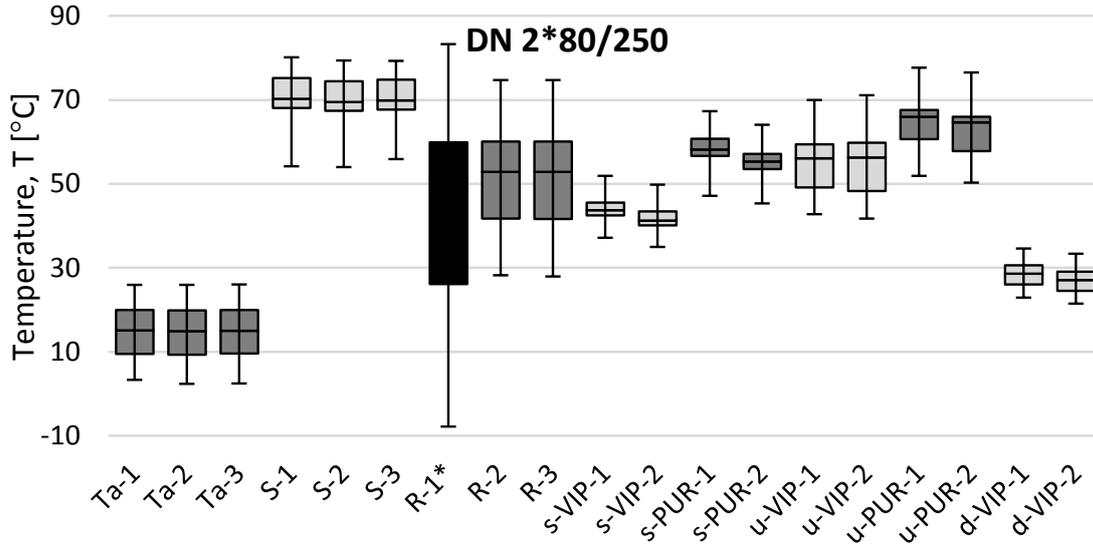
Figure 3.9: Boxplot of the temperature measurements in the pipe with dimensions DN 2\*80/250. The boxes show the minimum/1st quartile /median /3rd quartile/maximum of the measured temperatures. The temperatures are presented in alternating dark and light color corresponding to the same measurement position.
