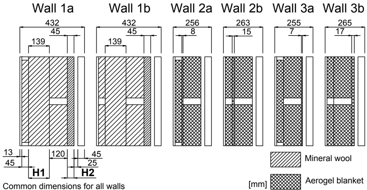
Figure 4.3: Description of the different walls used in the simulations. All walls have a simulated U-value of 0.10 W/m²K.
