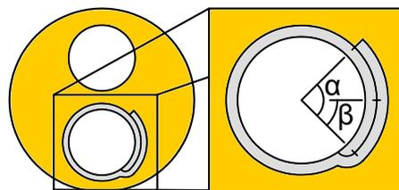
Figure 3.4: Definition of the VIP overlap. The overlap is defined by two angles,  $\alpha$  and  $\beta$ . The angle  $\alpha$  correspond to the overlap length and the angle  $\beta$  correspond to the placement of the beginning of the overlap, relative to the horizontal axis.
