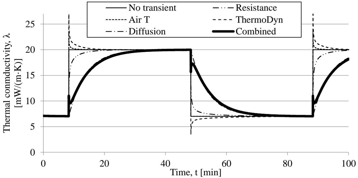
Figure 4.7: Simulated change in thermal conductivity of a fumed silica at varying pressure. The pressure was changed between 2 kPa and 100 kPa at 40 min intervals. The figure show the consequence of different transient effects. The curve for diffusion is almost completely covered by the combined result
