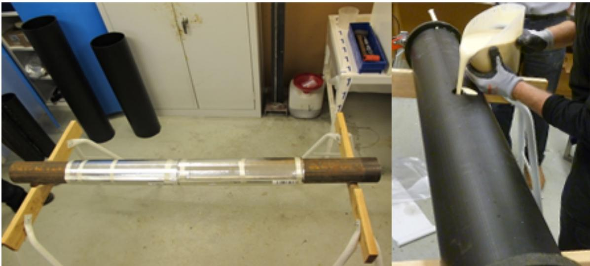
Figure 3.5: Prototype production of hybrid insulation district heating pipe with vacuum insulation panels.
