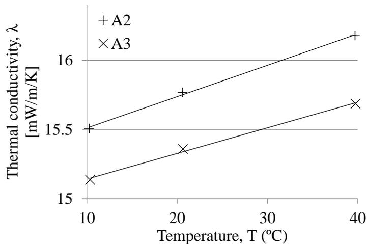
Figure 4.1: Relation between temperature and thermal conductivity for two samples of the aerogel blanket.
