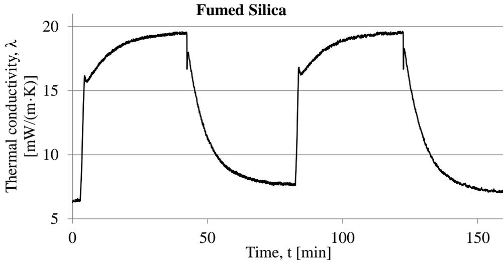
Figure 4.5: Measured thermal conductivity of a fumed silica at a varied pressure. The pressured was cycled between 2 kPa and atmospheric pressure at 40 min intervalls.
