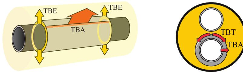
Figure 3.2: Description of the thermal bridges in the vacuum panel. The left image describes the thermal bridges at the edge of the panel (TBE) and along the panel (TBA). The right image shows a cross section of a twin pipe which also has a thermal bridge between the service pipes (TBT).
