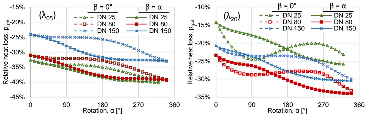
Figure 3.7: The heat loss relative to a reference PUR pipe depending on the length of the overlap.
