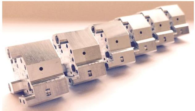
Figure 1. SWI band 2 integrated receiver front-end prototypes with integrated smooth wall spline horn antenna.
