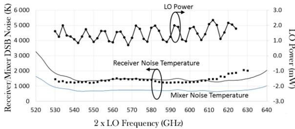
Figure 11. Measured band 1 receiver front end performance compared to simulations of the receiver and mixer noise performance versus LO frequency. Applied optimum LO pump power during measurements is also shown.
