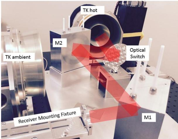
Figure 8. Room temperature Y-factor setup.
