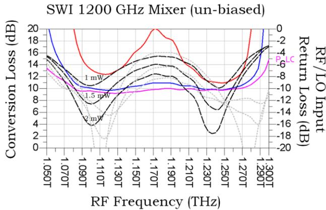
Figure 4. Simulated band 2 unbiased mixer performance.
