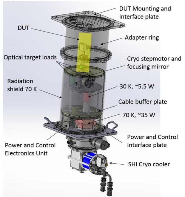
Figure 9. Cryogenic test setup under development.
