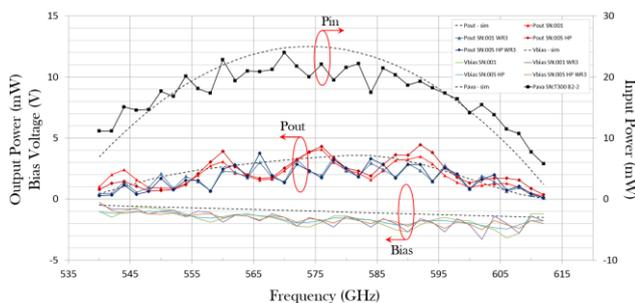
Figure 12. Measured and simulated performance of two band 2 600 GHz TMIC doubler breadboarding modules.
