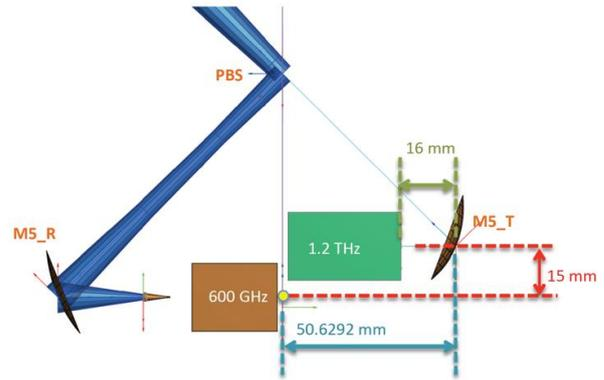
Figure 2. The SWI reflector system showing the relative position of the band 2 receiver unit relative the current band 1 receiver unit. Courtesy of Hyunjoon Kim, IAP, Bern.
