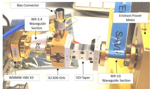
Figure 10. Photograph of the 600 GHz TMIC breadboard module under test using a 30 mW 300 GHz test source from Wasa Millimeter Wave AB.
