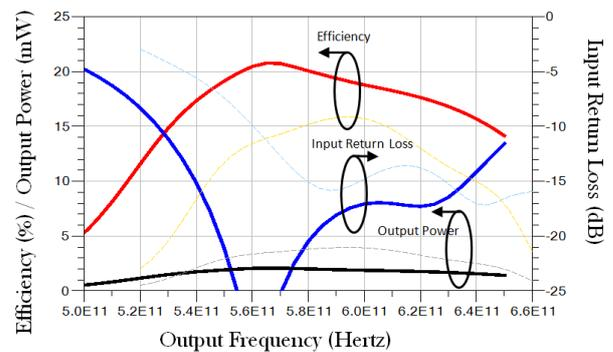
Figure 7. Simulated performance of the new improved 600 GHz doubler (solid) at 10 mW of pump power compared to the high power breadboard doubler (dashed) at 30 mW of input power.
