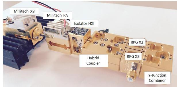
Figure 13. General LO testchain setup under development at Omnisys Instruments AB.
