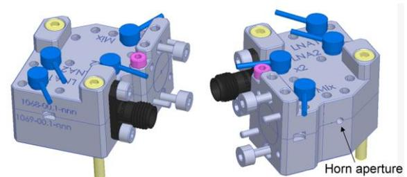
Figure 3. CAD model of the Band 2 front-end receiver unit with module integrated horn antenna, mixer, IF LNA, 600 GHz X2 multiplier and internal individual bias circuits for the LNA, mixer and multiplier.
