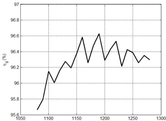
Figure 5. Simulated Gaussian efficiency of the smooth wall spline horn design versus frequency in GHz.
