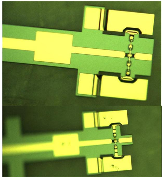
Figure 6. Photograph of the developed 4-anode (top) and 2-anode (bottom) 600 GHz X2 breadboard multiplier TMIC's with excess 4 mW of output power.
