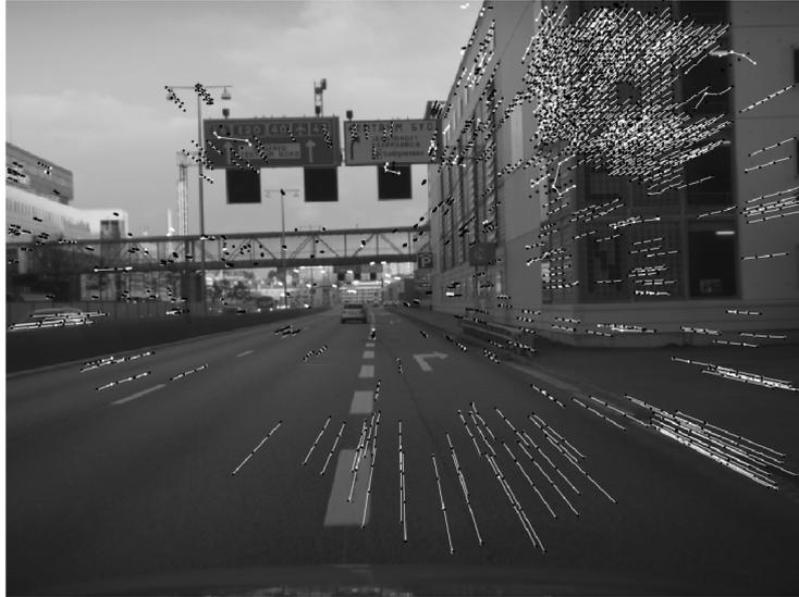
**Figure 5.7:** Reprojection error visualized for points that have been seen in four consecutive frames.
