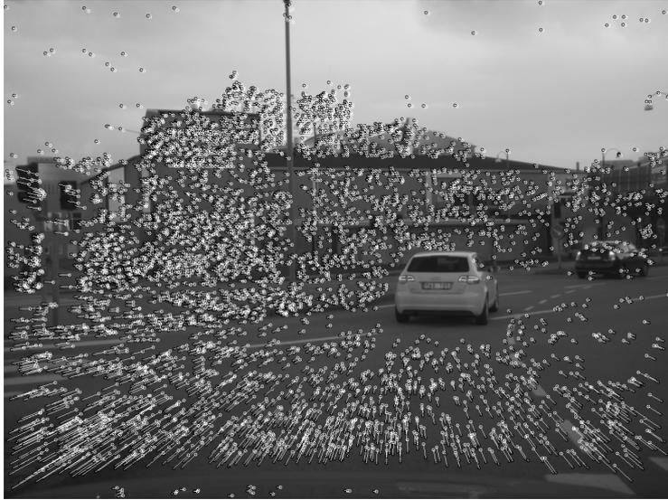
**Figure 5.5:** Matches that fulfill both Lowe's criterion and epipolar constraint.
