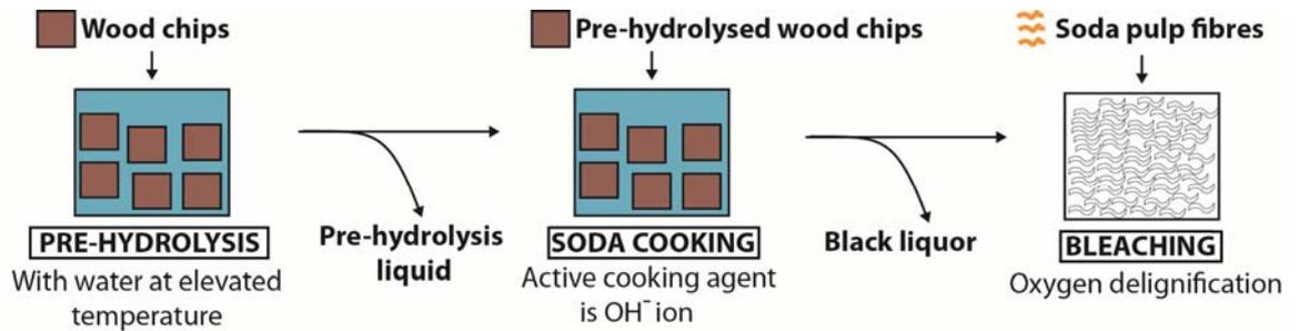
**Figure 3.** The main steps in a pre-hydrolysis soda cooking process.
