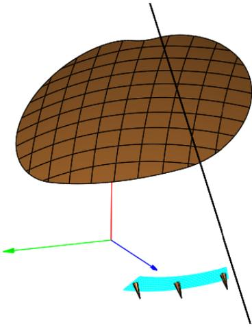
Fig. 2 Torus push-broom antenna with projected aperture  $D$  and focal length  $f$  of 5 m. The three feed positions represent scan directions of  $0^\circ$  and  $\pm 20^\circ$ . The feed array is shown in light blue.
