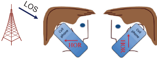
Fig. 1. Illustration of the random orientations of a wireless user device causing the user-random Pure-LOS, or briefly Random-LOS
