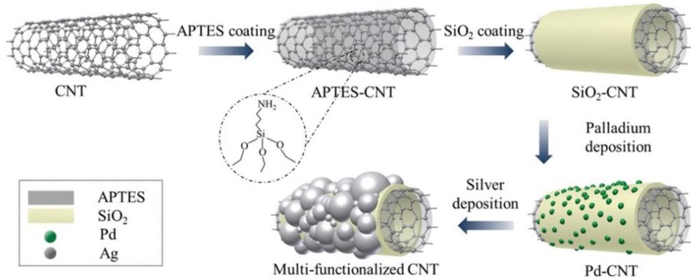
Figure 3.21: Schematic of the various modification steps in the synthesis of multi-functionalized CNT-based hybrid nanowires. The surface of CNTs was coated with APTES, silica, palladium nanoparticles, and silver nanoparticles. (from Paper E)
