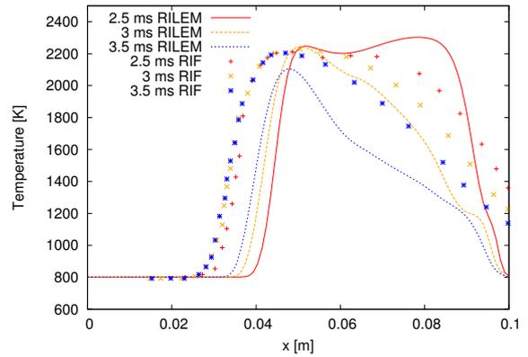
**Figure 4:** Comparison between interpolated values of the temperature on a line running along the length of the simulated combustion chamber and results from Pitsch et al [25] within the CFD domain at  $t = 2.5, 3, 3.5$  ms. On the horizontal axis of the plot, 0 corresponds to a position at the bottom of the chamber and a value of 0.1 corresponds to a position immediately below the nozzle.
