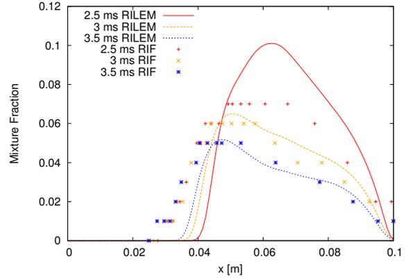
**Figure 3:** Comparison between interpolated values of the mixture fraction on a line running along the length of the simulated combustion chamber and results from Pitsch et al [25] within the CFD domain at  $t = 2.5, 3, 3.5$  ms. On the horizontal axis of the plot, 0 corresponds to a position at the bottom of the chamber and a value of 0.1 corresponds to a position immediately below the nozzle.
