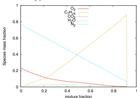
**Figure 5:** Mass fractions of individual chemical species within the mixture fraction space of the LEM at  $t = 0.5$  ms
