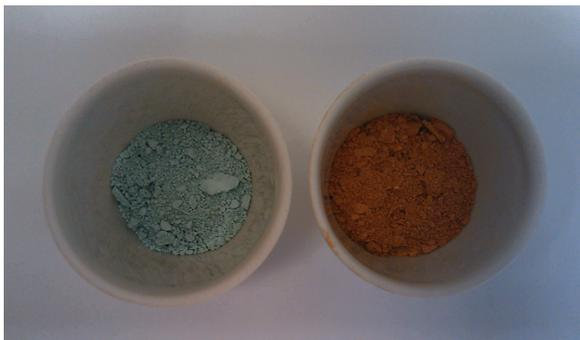
**Figure 4.2:** *Chabazite samples after ion-exchange with copper (left) and iron (right).*
