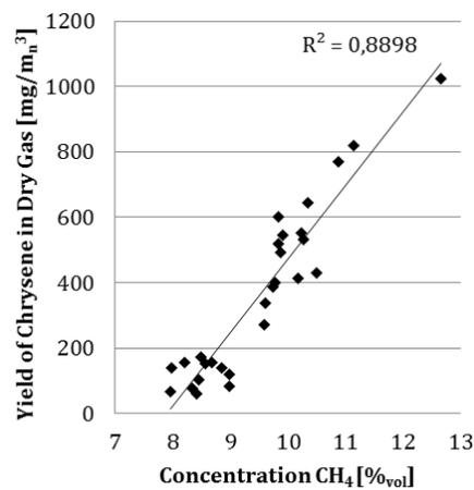
Figure 4. Yield of Chrysene as a function of  $\text{CH}_4$  concentration in the dry gas
