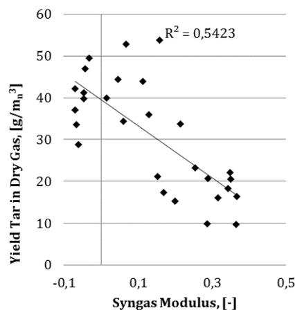
Figure 5. Yield of tar as a function of the syngas modulus
