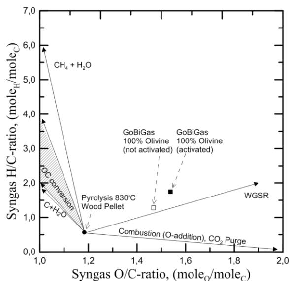
Figure 1. Illustration of how the syngas composition change with different reactions, described in detail by Larsson[13], and the examples are base on gas measurements from the GoBiGas-Gasifier.
