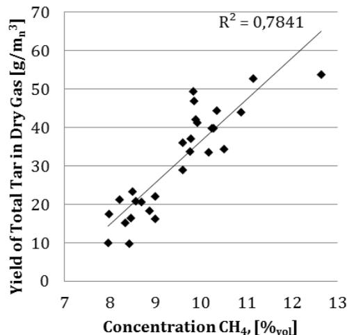
Figure 3. Yield of tar as a function of the concentration of CH<sub>4</sub> in the dry gas
