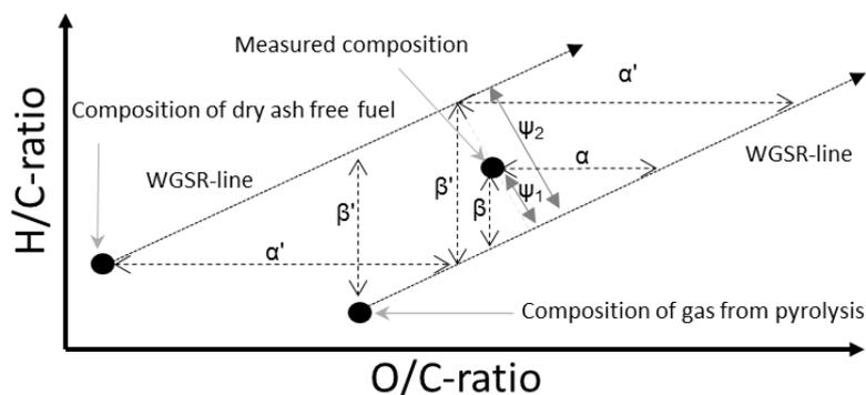
Figure 2. Illustration of variables used to calculate the syngas modulus,  $\Psi$ .
