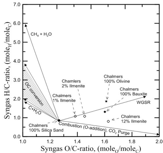
Figure 6. Comparison of the syngas composition using different bed materials in the Chalmers gasifier[11]. OC stands for organic compounds, which include tar and lighter hydrocarbons.
