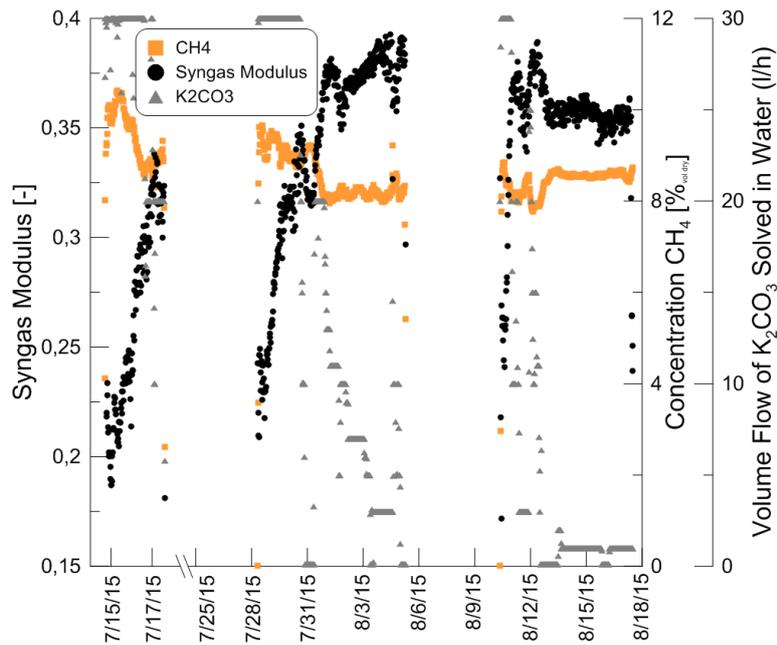
Figure 7. Trends for the syngas modulus (left y-axis), the  $\text{CH}_4$  concentration (right y-axis) and the amount of potassium added to the process (far right y-axis) is shown for 3 consecutive startups, all with used and previously active bed material.
