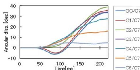
Fig. 16. Average time histories of the vertebral angular displacement relative to C7 for all volunteers in Test Series 1. The positive side is extension angle and negative flexion angle.
