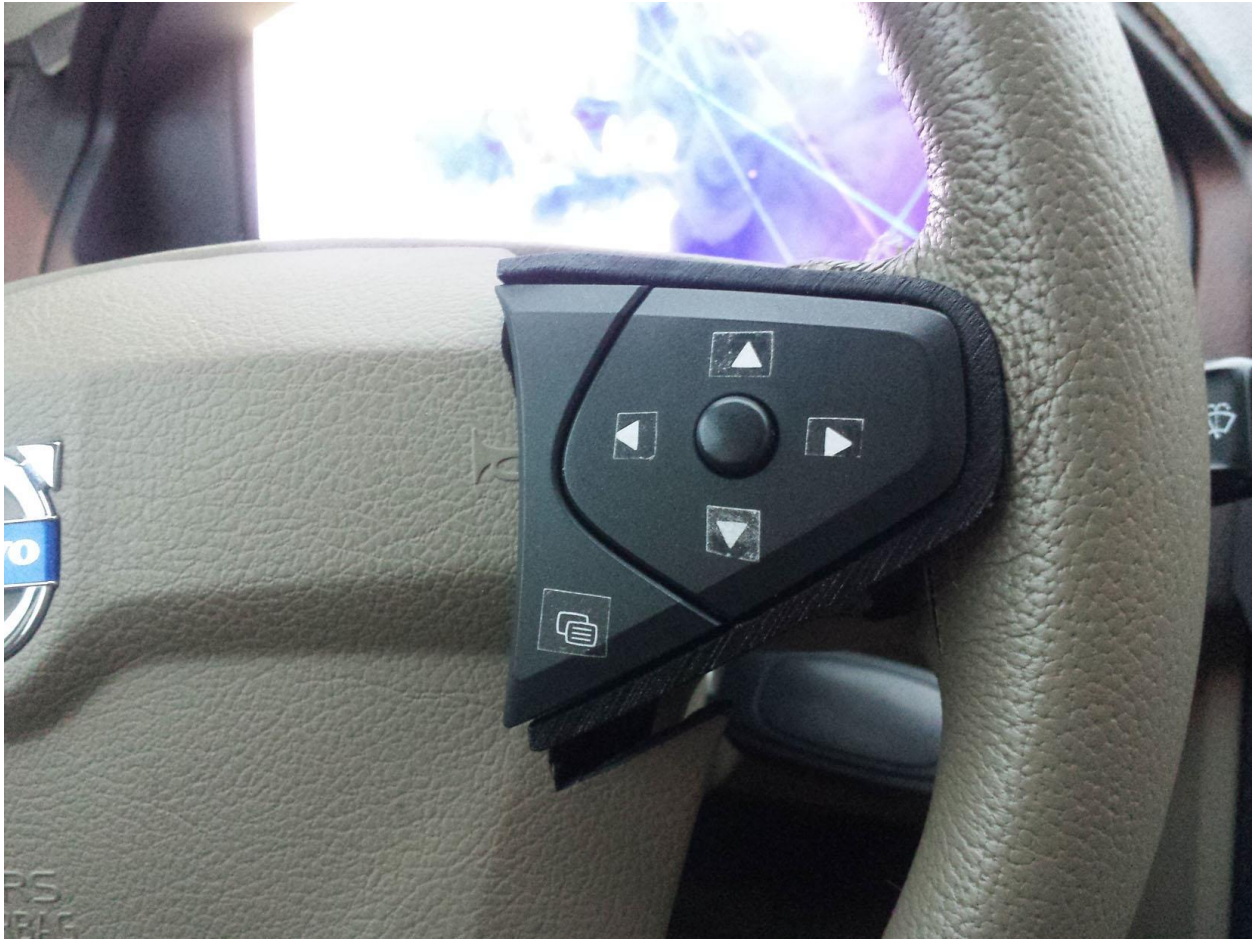
Figure 10. Input control for Volvo XC90 test vehicle
