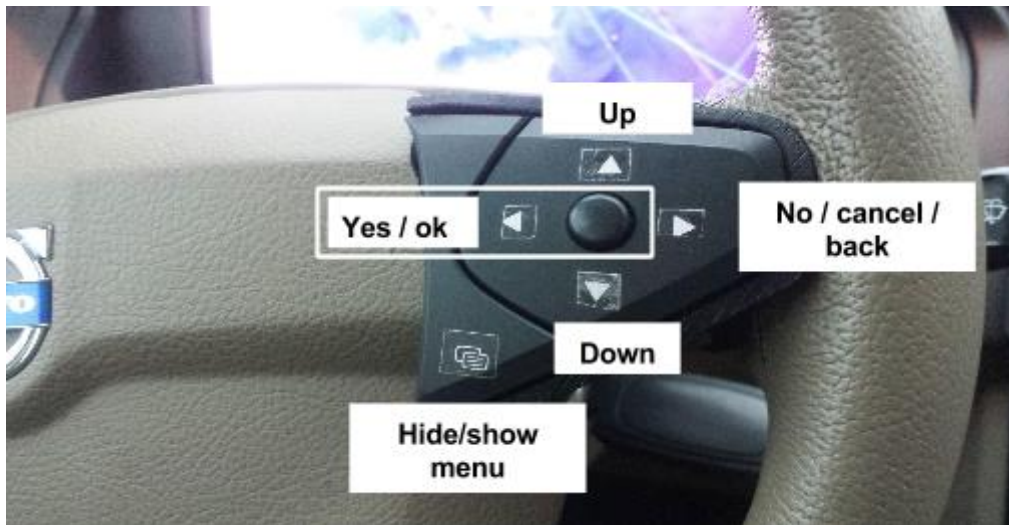
Figure 22. First set-up of interaction input for HUD
