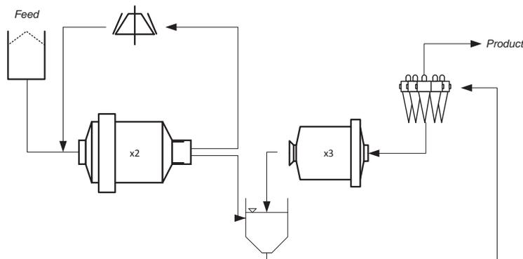
FIGURE 2. SABC (SAG-Ball-Mill-Crusher) example circuit
