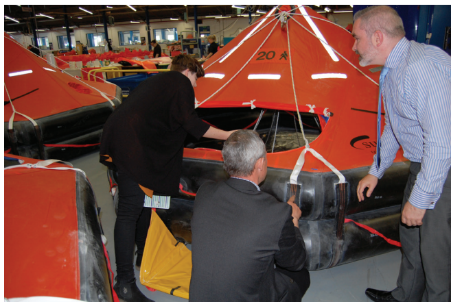
Figure 5. Inspection of 20 person davit launch liferaft undergoing testing
