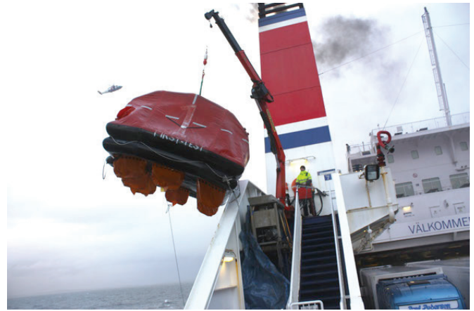
Figure 32. VIKING self-righting liferaft being lifted by a temporary crane on-board Stena Line vessel during testing in the FIRST-project (Swedish Sea Rescue Society, 2012)
