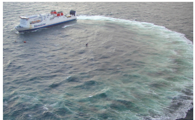
Figure 29. A ship from Stena Line performing the sea calming turn during testing of lifting liferafts (Lifeguard 901, 2011)
