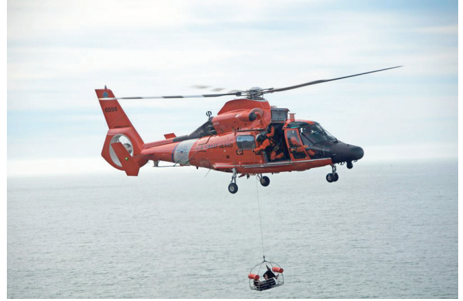
Figure 37. Rescue helicopter lifting with a foldable rescue basket (US Coast Guard, 2014)
