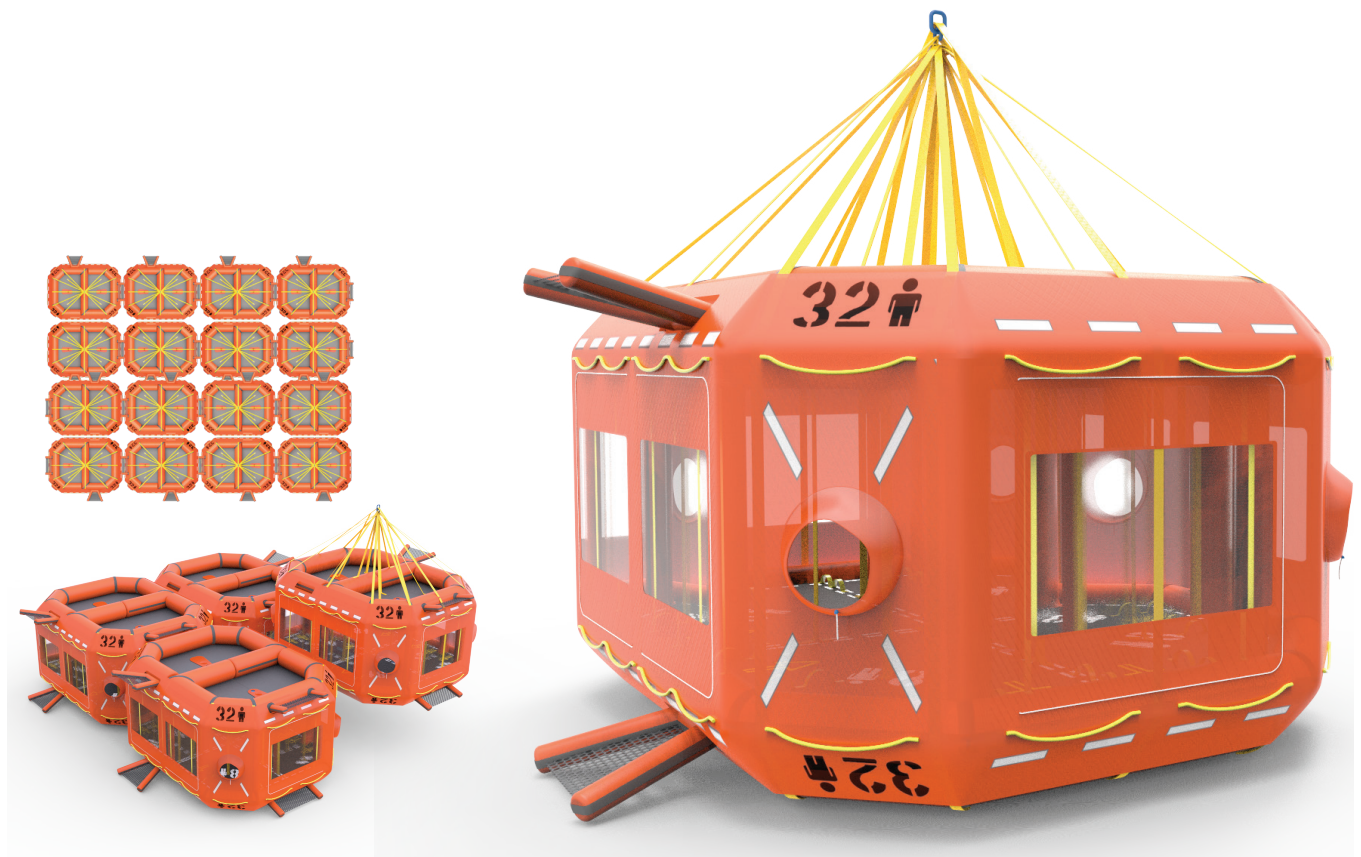
Figure 111. The MERS concept. Here being presented as a single raft unit, a raft section and an overview of the full system.
