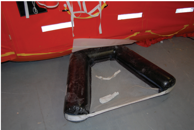
Figure 85. The aid for getting up from the water on RFD Beaufort Marin Ark 2
