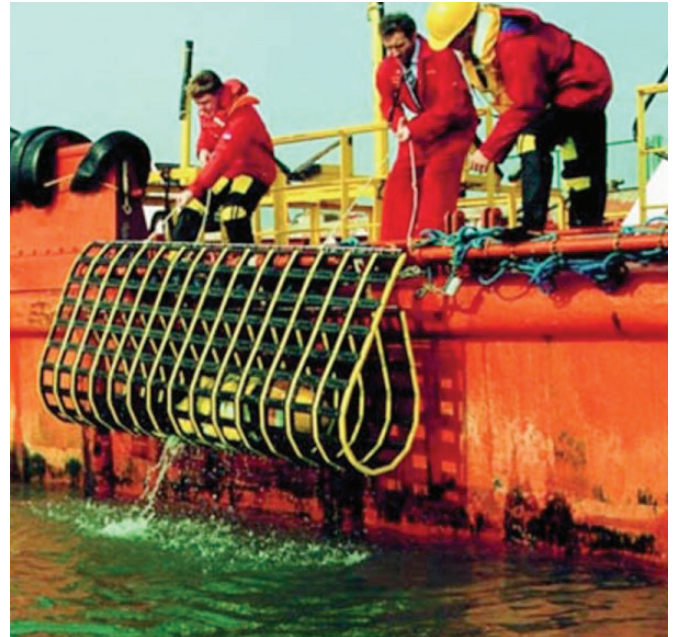
Figure 84. Use of a Jason's cradle. There are versions in fabric that could be better for inflatable products (Platypus Group, 2015)
