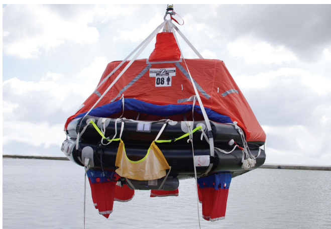
Figure 7. An eight person davit-launched liferaft being lowered to the water (Mercator Media, 2015)
