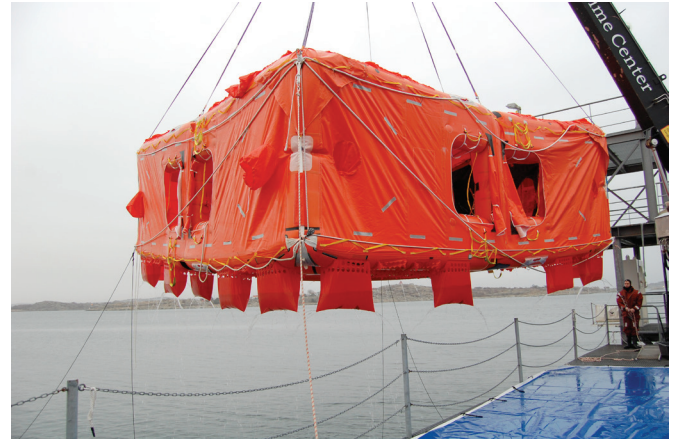
Figure 88. A Marin Ark 2 being lifted at the training facility (ÖMC). The long side sections are bending down, but since the raft is empty it is not critical.
