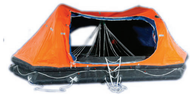
Figure 89. VIKING 39 person davit launch liferaft with a "forest" of lines inside (VIKING, 2006)
