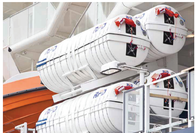
Figure 9. RFD throw overboard liferafts mounted on a ship (Survitec Group, 2014)
