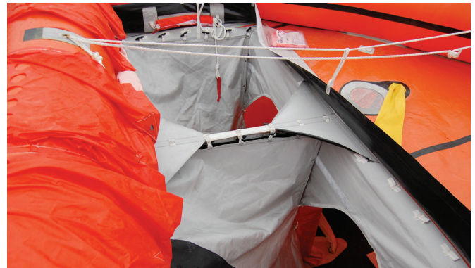
Figure 69. Openings for evacuation chutes in the Marin Ark roof
