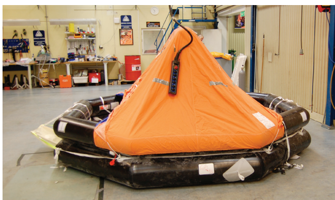
Figure 13. 16 pax liferaft inflated for pressure test
