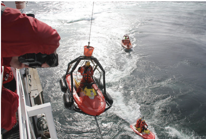
Figure 30. Rescuerunner being lowered in the drive through cradle (Matsson & Åslin, 2012)
