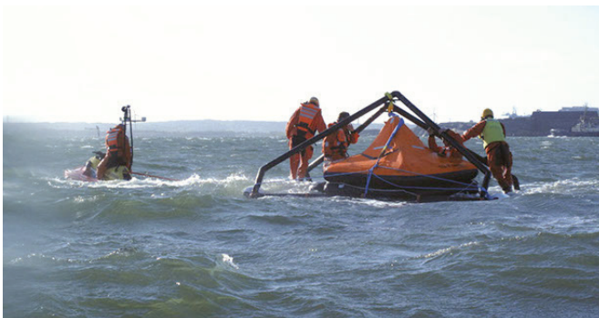
Figure 31. The liferaft lifting cradle (Falkman, Forsman & Hagman, 2009)
