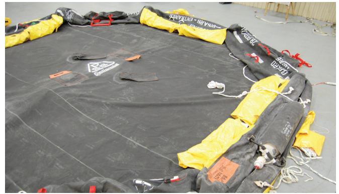
Figure 14. Unpacked and deflated, open and reversible liferaft during maintenance
