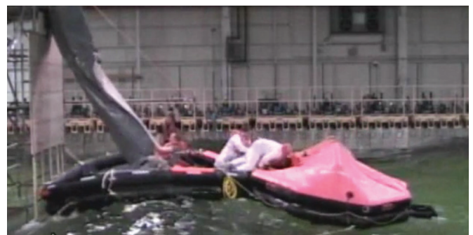
Figure 77. A Canadian test in a wave generator with rugby players going down an evacuation chute to a platform and entering a small liferaft. (Unknown, 2008)
