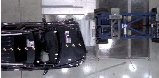
**Figure 20. MPDB test with Heavy Vehicle.**
