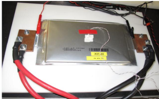
Fig. A.1 LG Chem 41 Ah battery.
