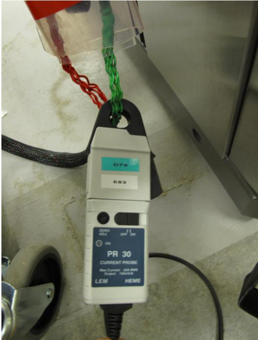
Fig. A.3 Current Probe Model PR30 used to measure the current during the experiments. It is a high bandwidth DC/AC current probe.
