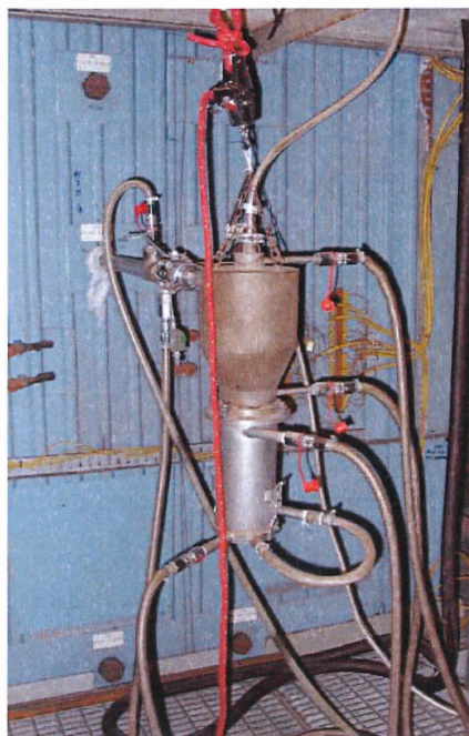
Figure 4 Schematic drawing of water-cooled particle extraction probe with cyclone and container (left) and photograph of the solids extraction equipment during the tests (right).
