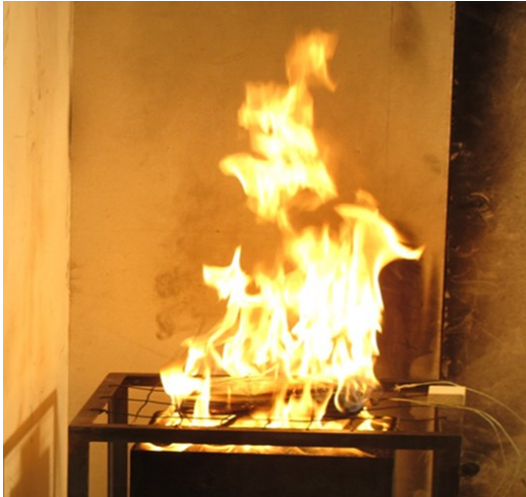
Figure 1. Fire test in EiG 7 Ah LFP pouch cells
