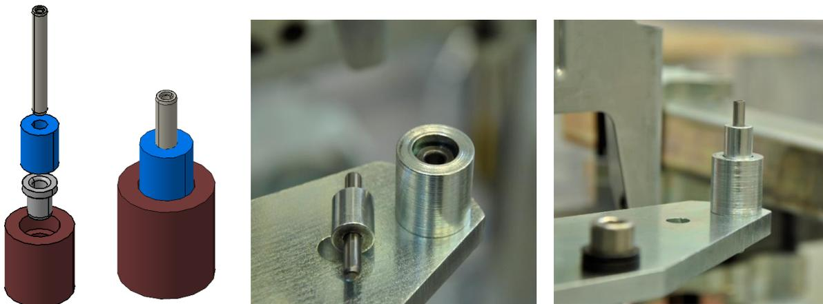
Fig. 4. Locator assembly of a cylindrical guiding unit, bushing, sleeve and a dowel pin
