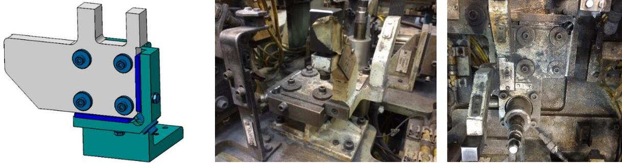
Fig. 3. (a) 3D model of a shimming plates and fixture part; (b) Fixture application at Olofström plant of VCC
