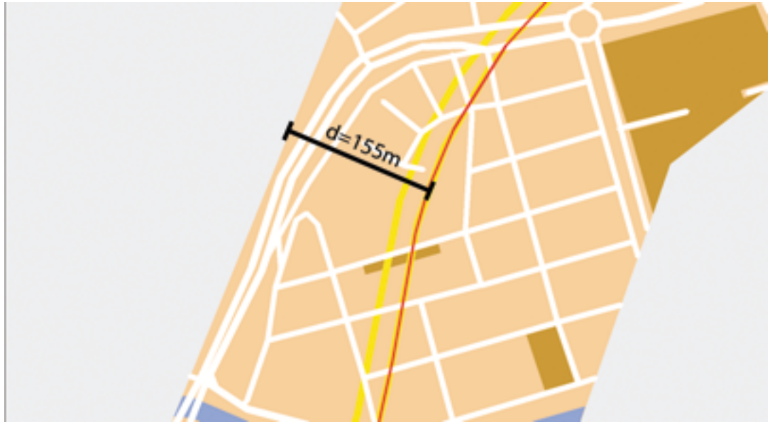
Figure 33: With the tile simplification set to 30 it generalizes the tiles too much, making the distance from the route to the corridor border too short.
