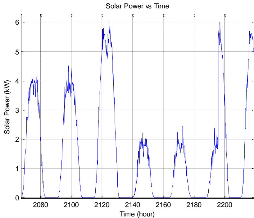
Fig. 11. Example of simulated solar power. Part of the total time range.
