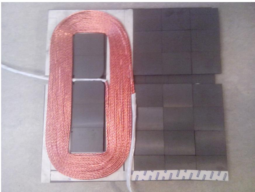
**Coils for wireless charging of vehicles using a resonant auxiliary winding**
