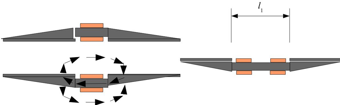
Figure 8a. Leakage flux paths. 8b. Divided coil.
