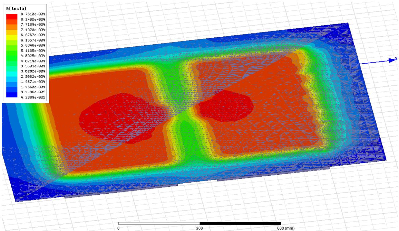
Figure 14. Flux density in the middle of the air gap of a bar design. Current is 150 A.
