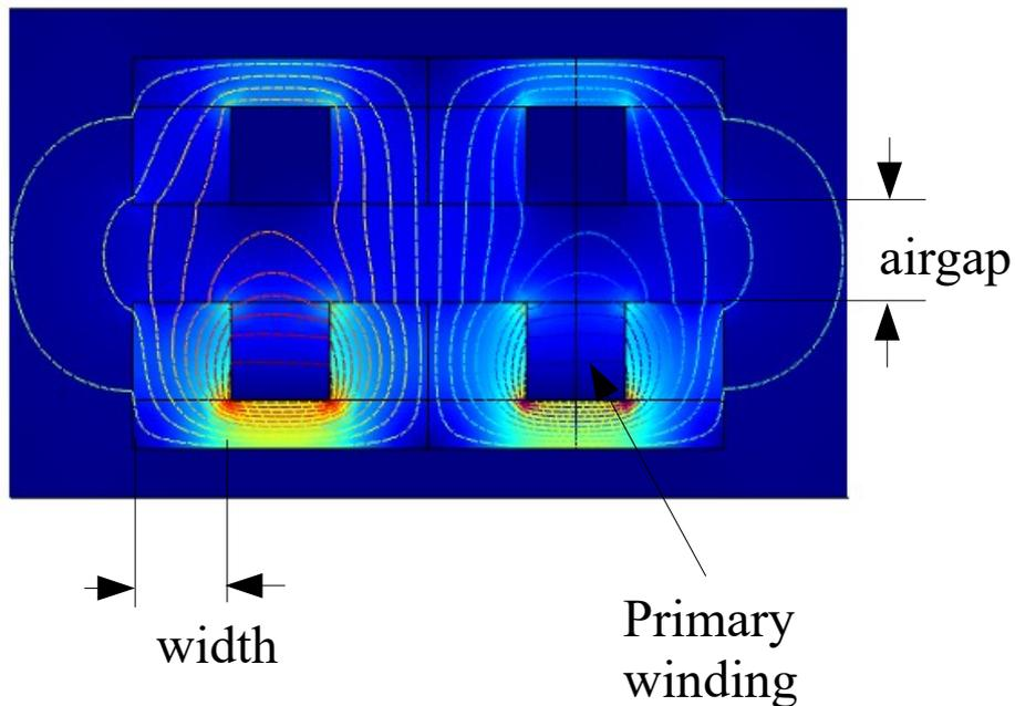
Figure 10. E-cores and primary winding.
