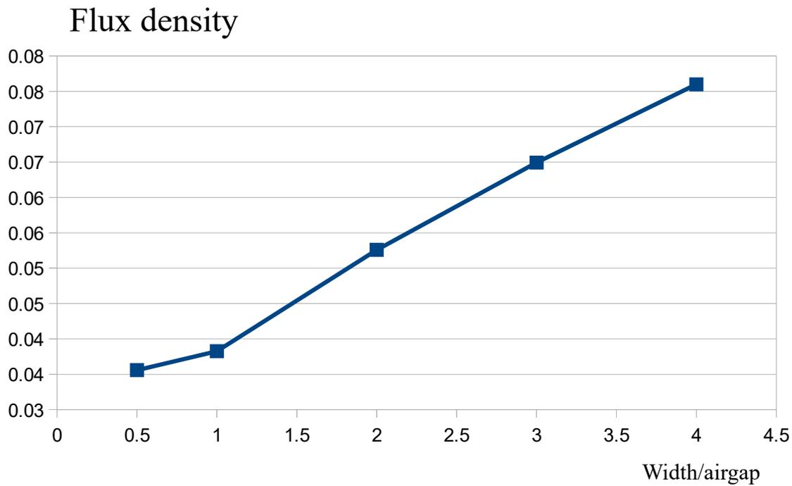
Figure 12. Relative flux density three air gap lengths from the core, flux density normalised to maximum air gap flux density.
