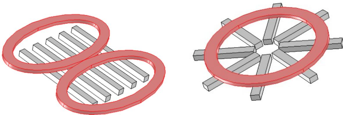
Figure 2a. DD-coil, Auckland [5]. 2b. Circular coil. Grey-ferrite red-copper
