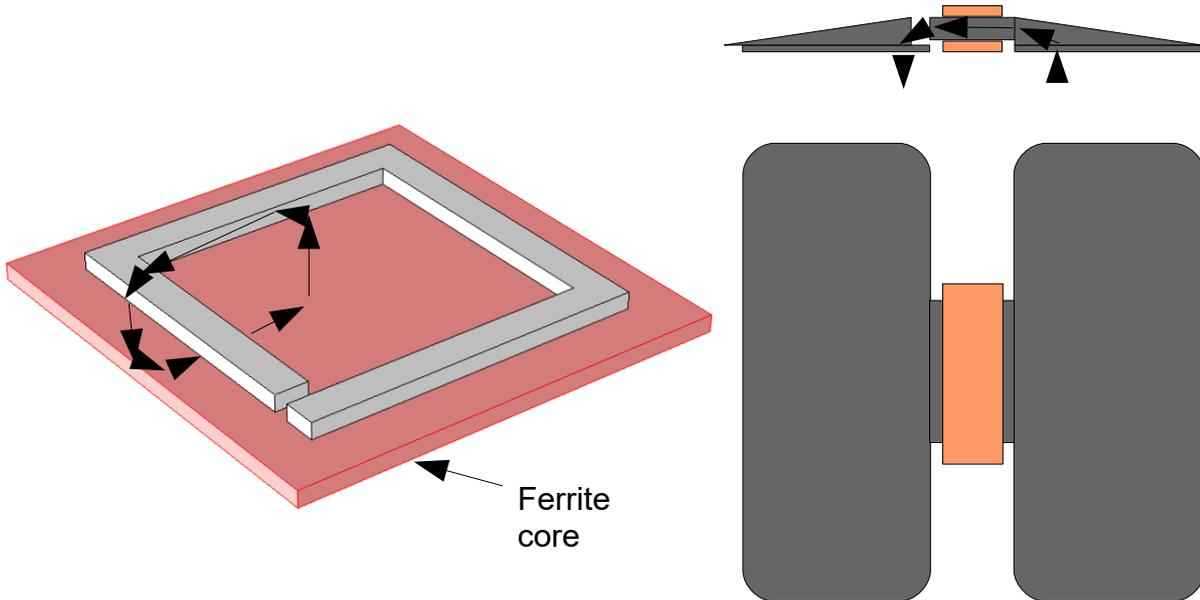
Figure 7a. Return path via ferrite core, circular coil. 7b. Return path via centre concentrated winding, bar type coil.
