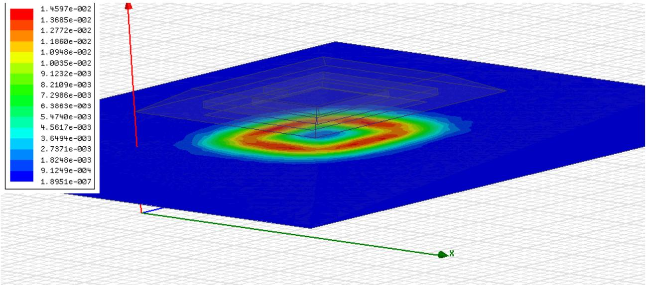
Figure 23. Flux density in the middle of the air gap of the Circular/Square coils.
