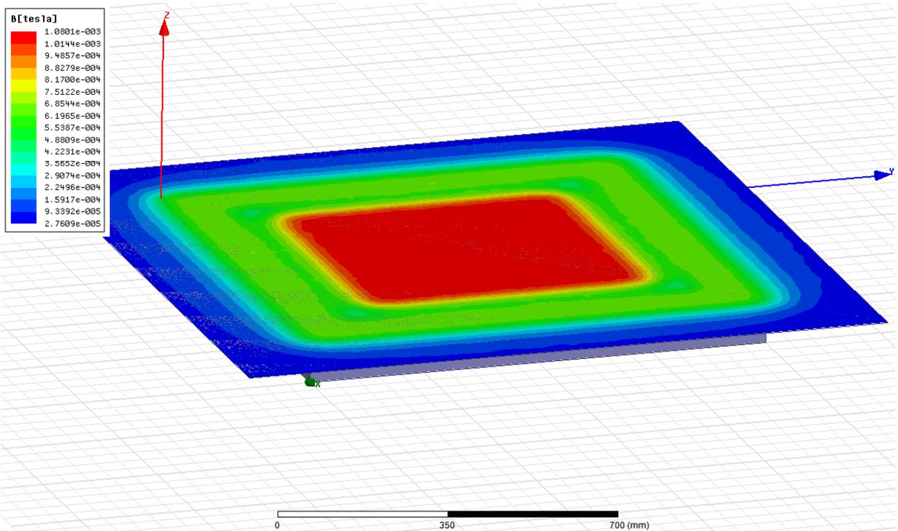
Figure 13. Resulting absolute flux density from a circular coil in the middle of the air gap, current in the sending coil is 150 A. Number of turns is one.
