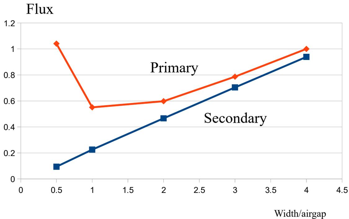
Figure 11. Relative flux vs relative width of the core,  $b_w$ , normalised with the air gap length.
