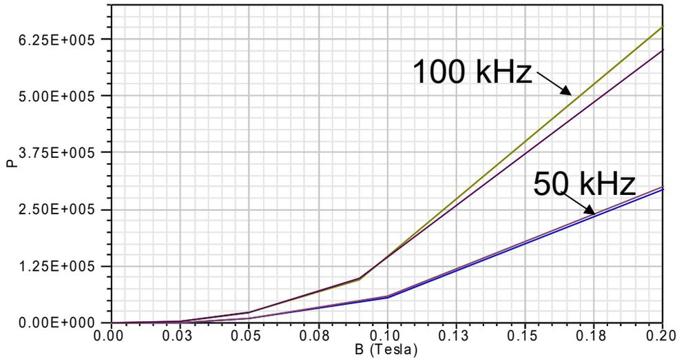
Figure 21. Core losses/W/m<sup>3</sup> as function of flux density approximated in Maxwell.
