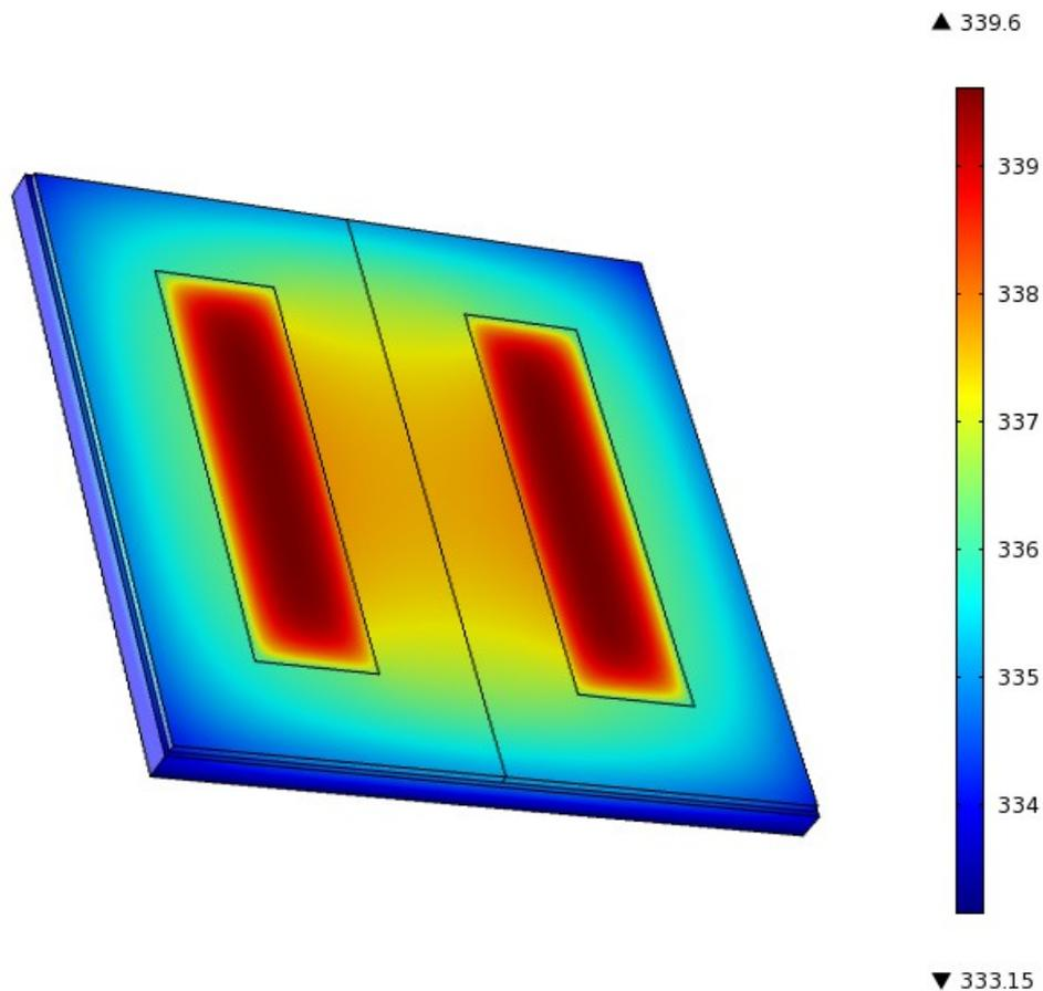
Figure 24. Resulting temperature /K at 90 W losses. Cooling of backside.
