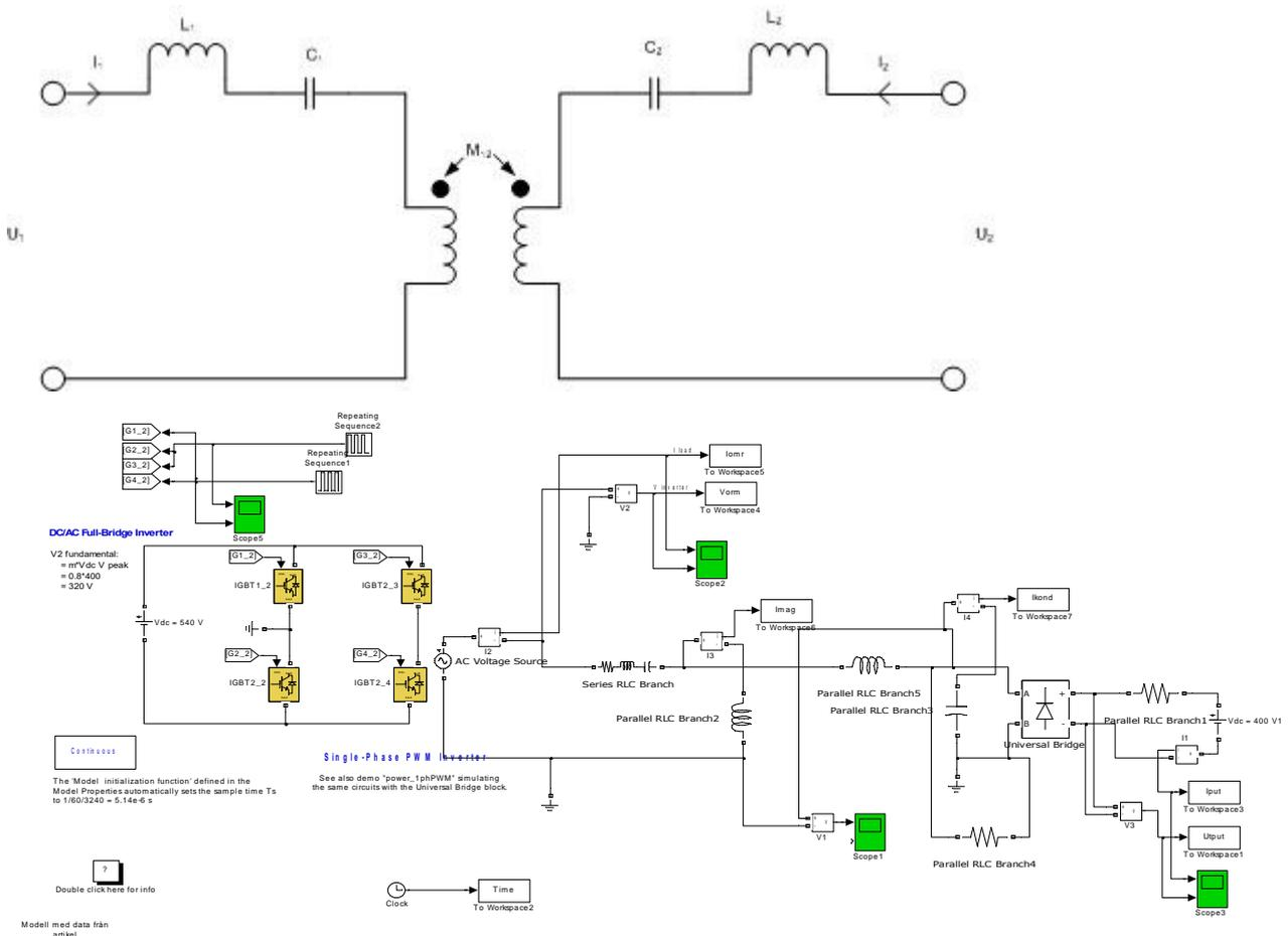
Figure 16. Two winding circuit and a representation in Simulink.
