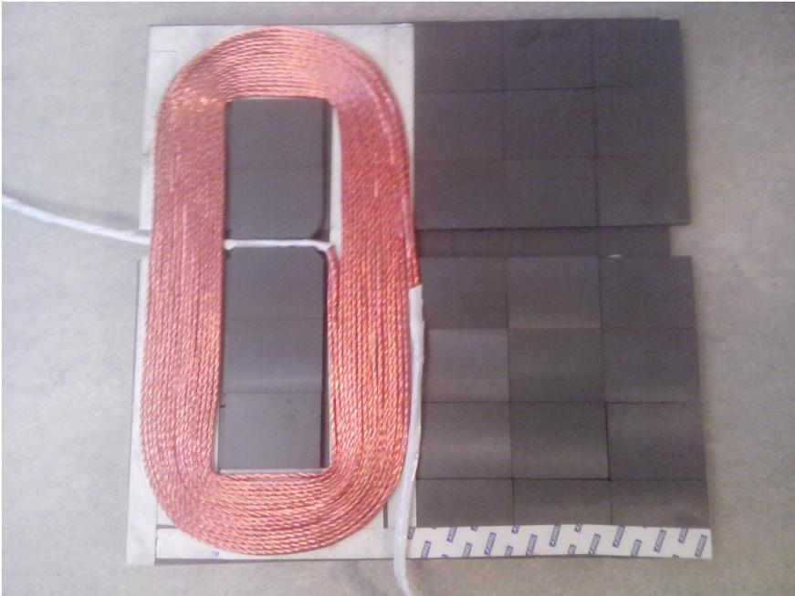
Figure 25. Prototype DD-coil.
