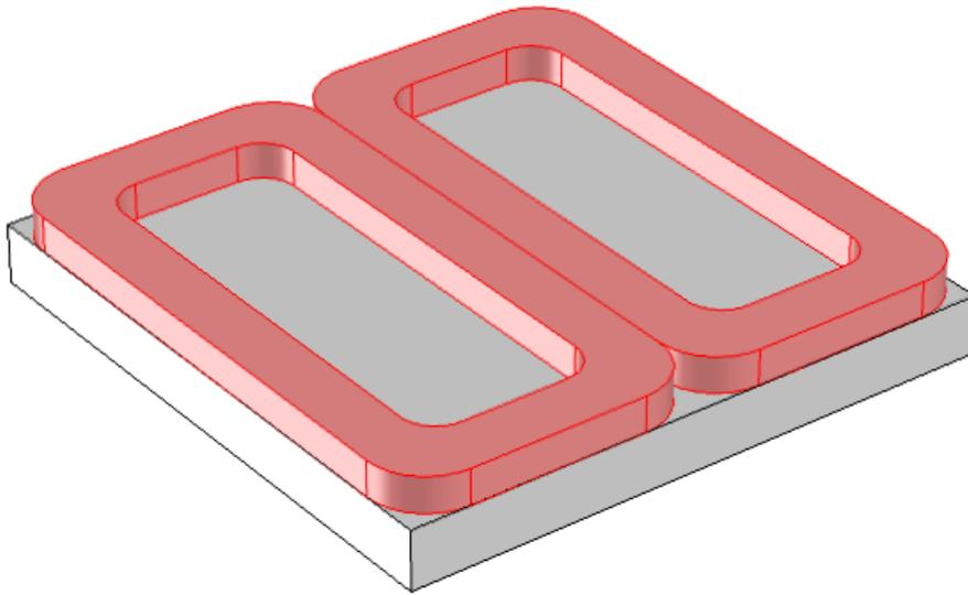
Figure 5. DD-coil.
