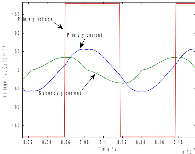
Figure 22. Simulated voltage and current to the coil.
