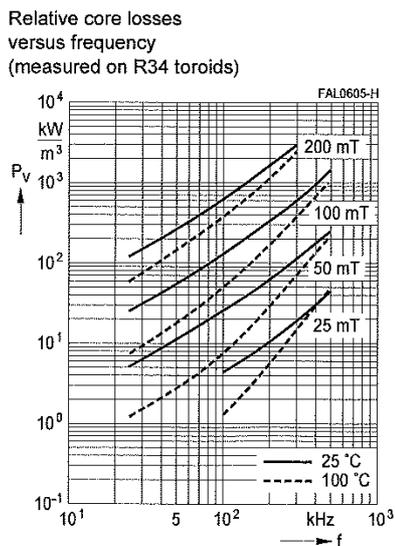
Figure 18. Core losses of N87 vs frequency.
