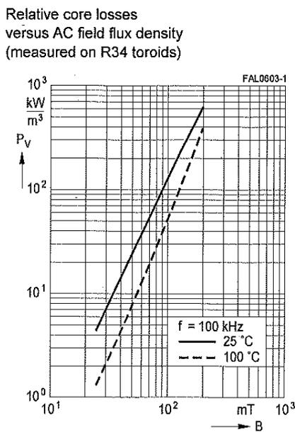
Figure 17. Core losses of N87 vs flux density at 100 kHz.
