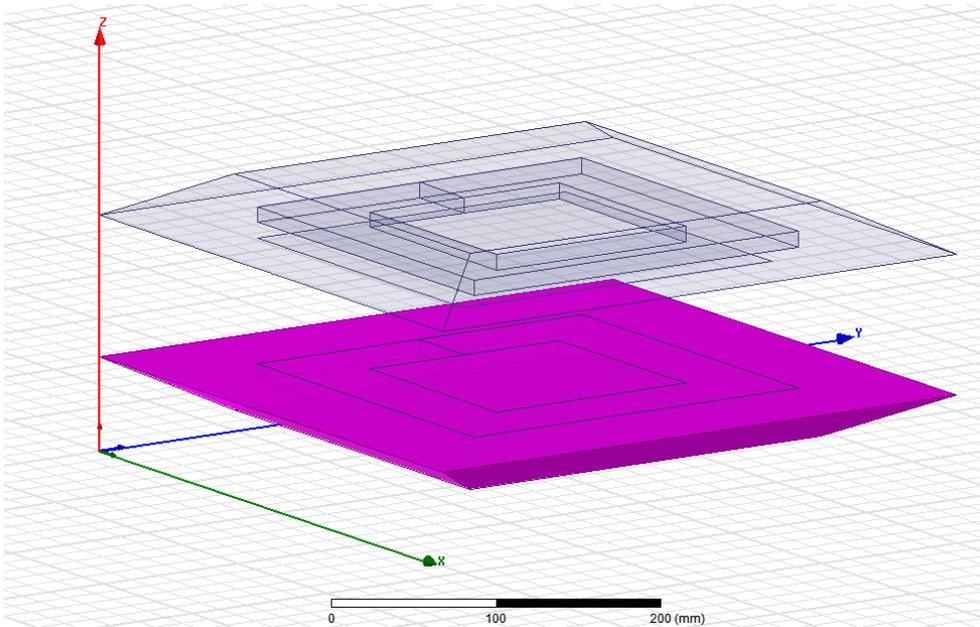
Figure 20. Analysed coil with a ferrite core and embedded winding.
