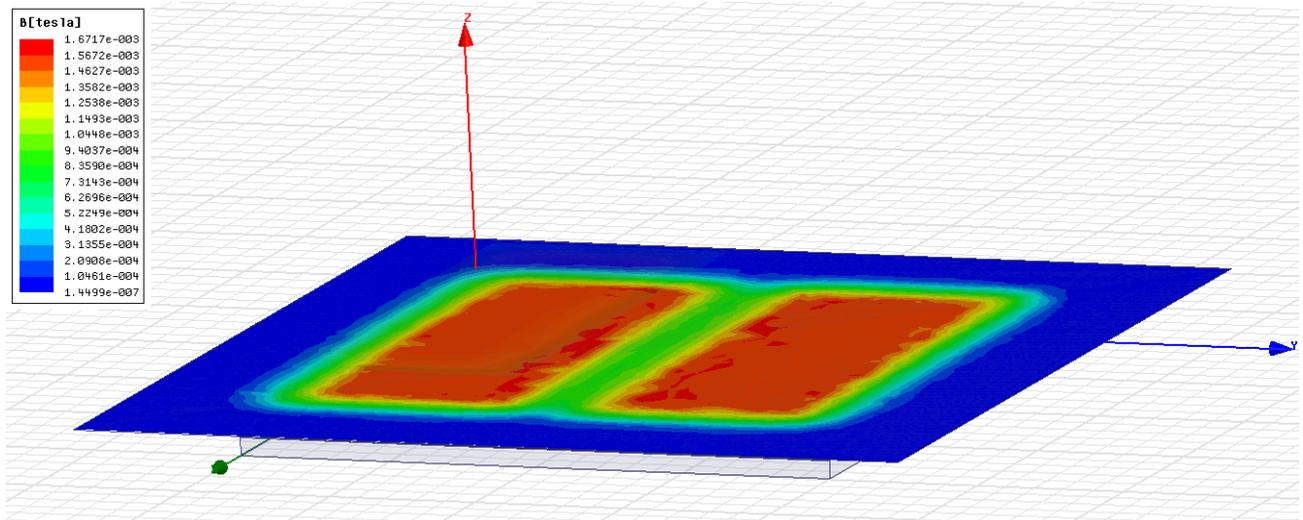
Figure 15. Flux density in the middle of the air gap from the DD-coil
