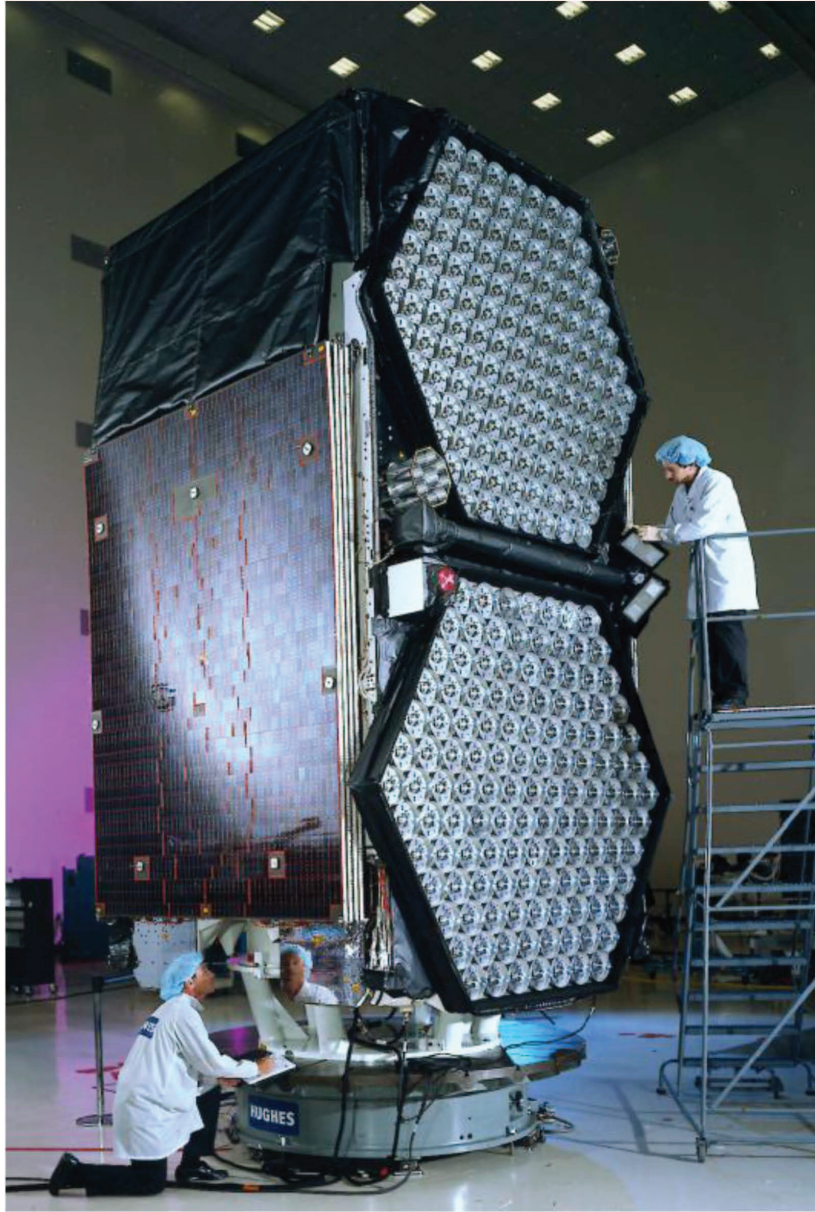
Figure 1.2: Two dense DRA:s of patch-excited antennas for MEO communication at S-band. For GEO applications, an order of a thousands elements is expected.
