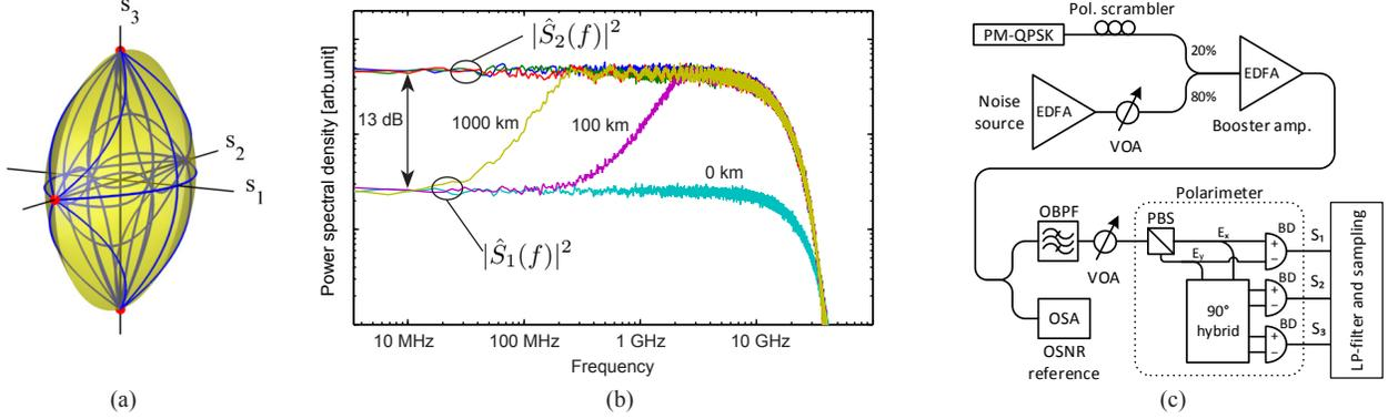
Fig. 1. (a) The Stokes representation of PM-QPSK. (b) The simulated spectrum of the Stokes parameters for different fiber lengths. (c) The experimental setup. VOA: Variable optical attenuator, OBPF: Optical band-pass filter, OSA: Optical spectrum analyzer, PBS: Polarization beam splitter, BD: Balanced detector, LP: Low-pass
