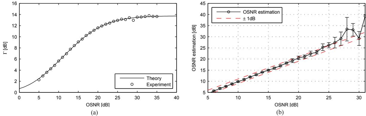
Fig. 2. (a) The theoretical curve for  $\Gamma$  together with experimental values. (b) OSNR estimation. The error bars represent the standard deviation of the dB-values of ten measurements.
