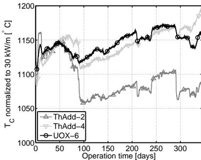
**Figure 5.2:** Measured  $T_C$  for rods *ThAdd-2*, *ThAdd-4* and *UOX-6*.
