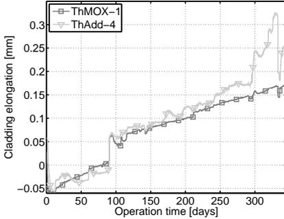
**Figure 5.6:** Cladding elongation measured for rods *ThMOX-1* and *ThAdd-4*.
