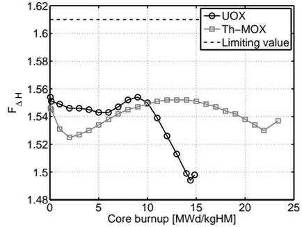
**Figure 4.5:**  $F_{\Delta H}$ , i.e. maximum rod power relative to core average rod power as a function of burnup, for the Th-MOX and the reference UOX core.
