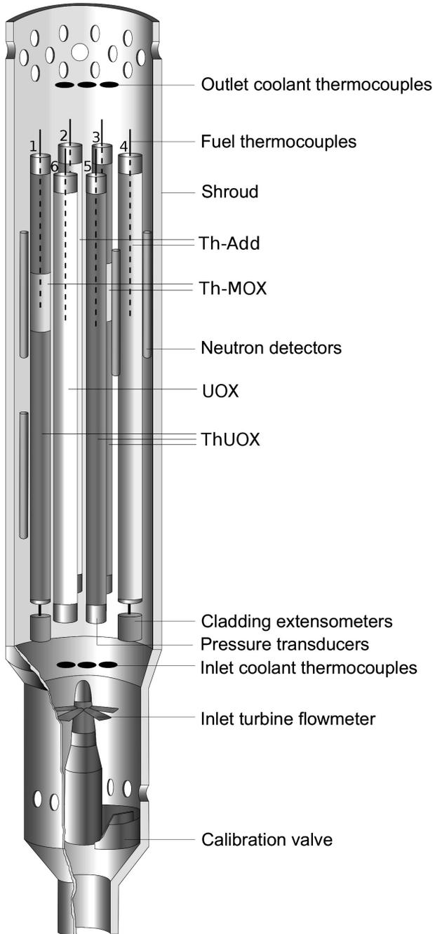
**Figure 5.1:** Schematic image of the testrig IFA-730.
