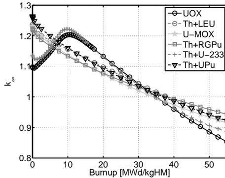
**Figure 3.1:** The infinite multiplication factor for the investigated fuel types.
