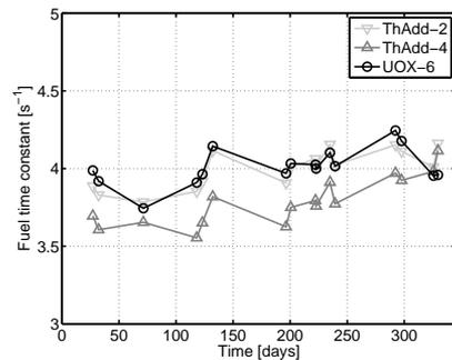
**Figure 5.3:** Scram time constants for rods *ThAdd-2*, *ThAdd-4* and *UOX-6*.
