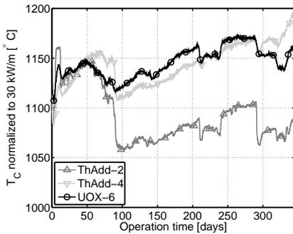
**Figure 5.2:** Measured  $T_C$  for rods *ThAdd-2*, *ThAdd-4* and *UOX-6*.
