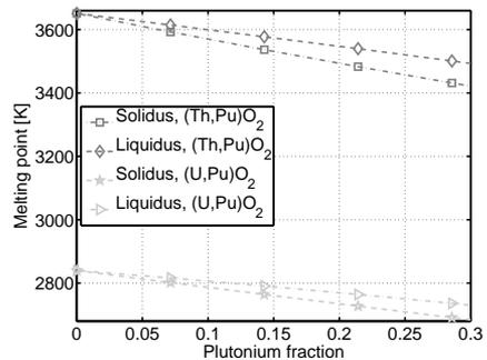
**Figure 5.9:** Solidus and liquidus temperatures for  $\text{Th}_{1-y}\text{Pu}_y\text{O}_2$  and  $\text{U}_{1-y}\text{Pu}_y\text{O}_2$  for  $\text{PuO}_2$  fractions lower than 30%.
