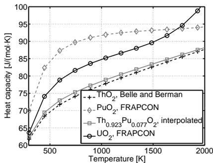
**Figure 5.10:** Heat capacity for  $\text{ThO}_2$ ,  $\text{PuO}_2$ ,  $\text{UO}_2$  and the present Th-MOX material.
