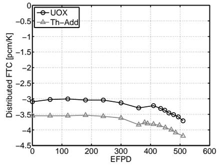
**Figure 3.5:** The FTC in the Th-Add and reference UOX cores.
