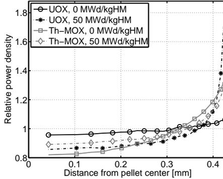
**Figure 5.12:** Radial pellet power profiles for UOX and Th-MOX fuel at 0 and 50 MWd/kgHM. The UOX fuel is enriched to 5% and the Pu concentration in the Th-MOX fuel is 8% with 80% Pu-239.
