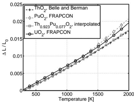
**Figure 5.8:** Thermal expansion of  $\text{ThO}_2$ ,  $\text{PuO}_2$ ,  $\text{UO}_2$  and the present Th-MOX material.
