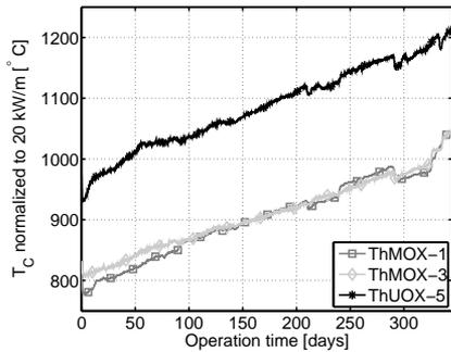
**Figure 5.4:** Measured  $T_C$  for rods *ThMOX-1*, *ThMOX-3* and *ThUOX-5*.
