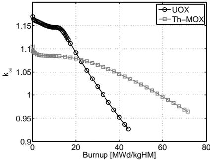
**Figure 4.4:**  $k_\infty$  development with burnup for the Th-MOX and the reference UOX fuel assembly.
