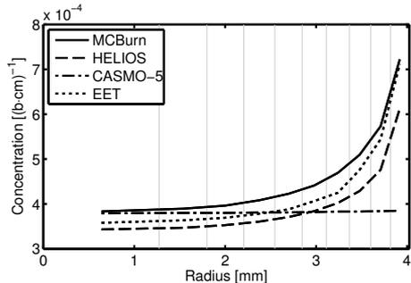
**Figure 4.2:** Modelled radial uranium distribution in the Th-MOX rod.
