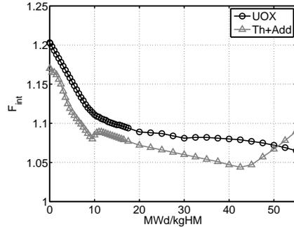
**Figure 3.3:** The assembly internal power peaking factor.
