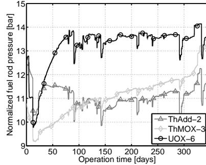
**Figure 5.7:** Fuel rod pressures measured for rods *ThAdd-2*, *ThMOX-3* and *UOX-6*.
