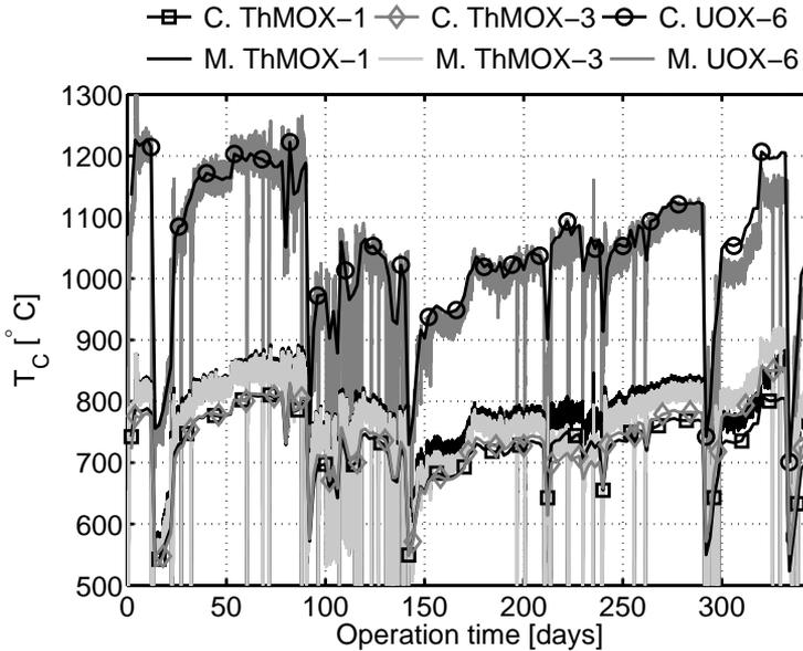
**Figure 5.13:** Calculated (C) and measured (M) fuel centerline temperatures for rods *ThMOX-1*, *ThMOX-3* and *UOX-6*.
