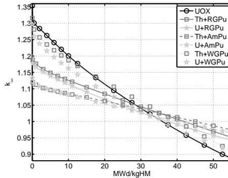
**Figure 4.3:**  $k_\infty$  development with burnup for the UOX reference and six of the investigated Th-MOX and U-MOX fuel types. The  $k_\infty$  curves for the 2RPu cases are omitted for clarity. They are very similar to those of the RGPu cases.
