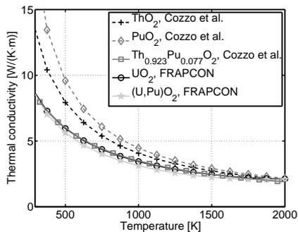
**Figure 5.11:** Thermal conductivity for  $\text{ThO}_2$ ,  $\text{PuO}_2$ ,  $\text{UO}_2$ , U-MOX fuel and the present Th-MOX material.
