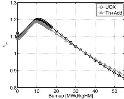
**Figure 3.2:**  $k_{\infty}$  development with burnup for Th-Add and a reference UOX fuel assembly.
