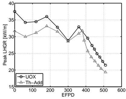
**Figure 3.4:** The peak LHGR in the Th-Add and reference UOX cores.
