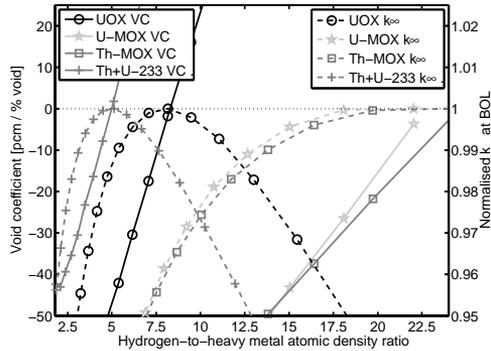
**Figure 4.6:** Normalized  $k_\infty$  and void coefficients for four different fuel types.
