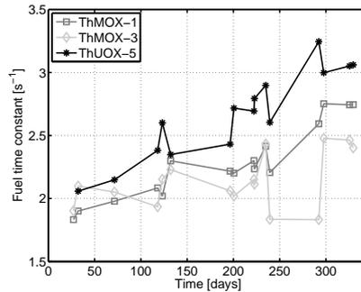
**Figure 5.5:** Scram time constants for rods *ThMOX-1*, *ThMOX-3* and *ThUOX-5*.
