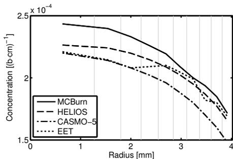
**Figure 4.1:** Modelled radial plutonium distribution in the Th-MOX rod.
