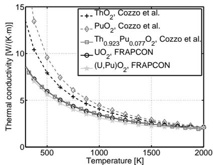
**Figure 5.11:** Thermal conductivity for ThO<sub>2</sub>, PuO<sub>2</sub>, UO<sub>2</sub>, U-MOX fuel and the present Th-MOX material.
