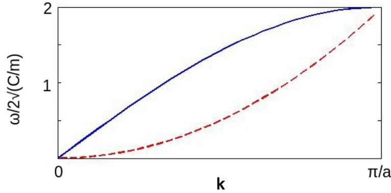
**Figure 3.2:** The dispersion relation derived from the spring model (solid blue line), and the dispersion relation for the flexural vibration of a thin plate (dashed red line).
