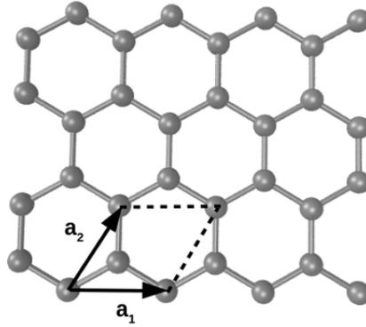
**Figure 3.3:** Lattice structure of graphene, with the lattice vectors  $\mathbf{a}_1$  and  $\mathbf{a}_2$  indicated by arrows.
