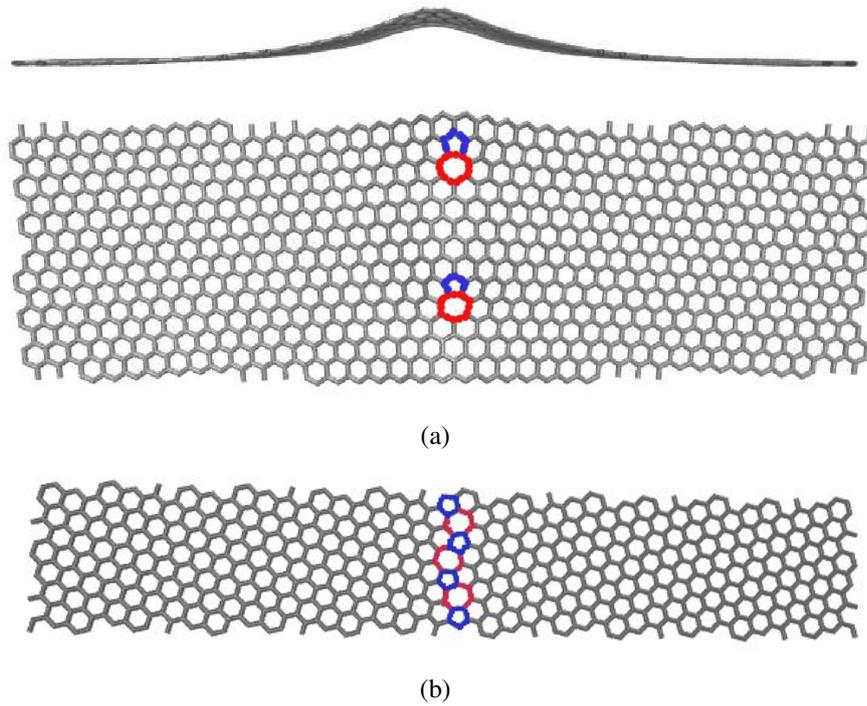
**Figure 3.8:** (a): A grain boundary with misorientation angle  $9.4^\circ$ , viewed from an in-plane direction (upper image) and from the direction perpendicular to the graphene sheet (lower image). This grain boundary clearly displays out-of-plane buckling. The dislocations are indicated in red (heptagon) and blue (pentagons). (b): A grain boundary with misorientation angle  $32.2^\circ$ .
