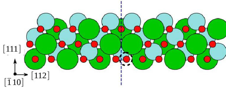
**Figure 5.2:** The  $(112)[\bar{1}10](0,0)$  grain boundary with a dashed circle indicating the oxygen site with the most negative segregation energy.
