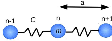
**Figure 3.1:** A one-dimensional chain of atoms with mass  $m$ , at distance  $a$  from each other and connected by springs with spring constant  $C$ .
