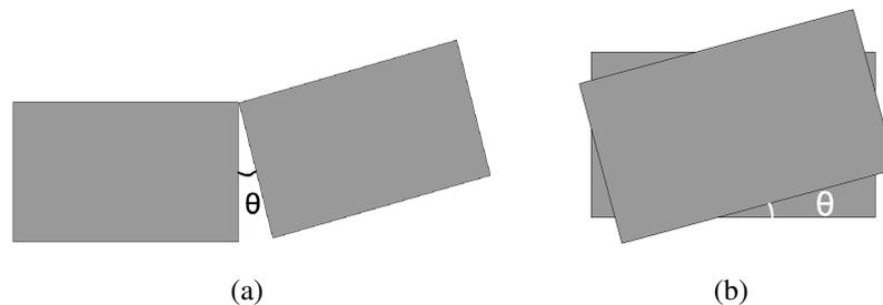
**Figure 1.2:** Schematic depicting the construction of a tilt grain boundary (a) and a twist grain boundary (b) with misorientation angle  $\theta$ .
