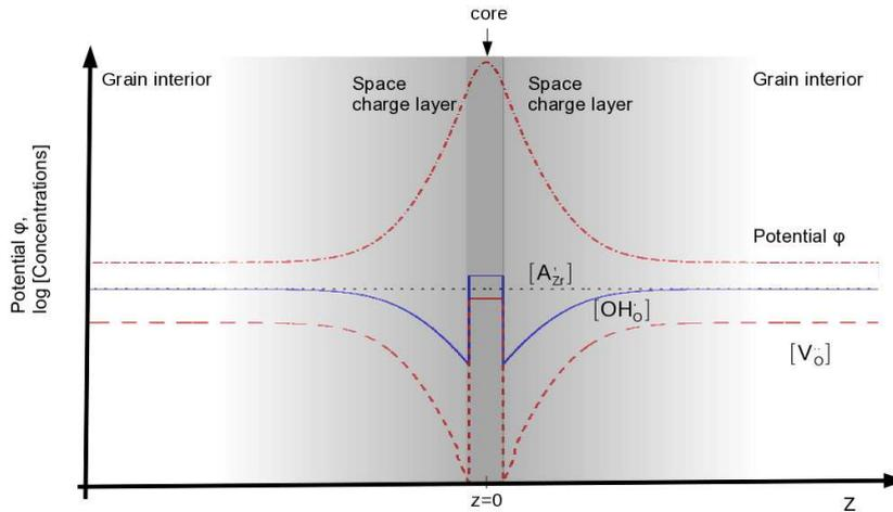
**Figure 2.7:** Schematic of a grain boundary with space charge layers in BaZrO<sub>3</sub>, assuming a constant dopant concentration. The figure has been redrawn based on Figure 1 in Paper III.
