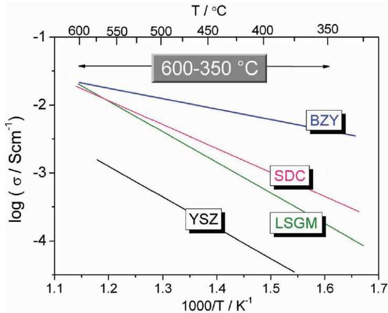
**Figure 2.3:** Temperature dependence of the conductivity of the oxygen ion conductors yttria-stabilized zirconia (YSZ), Sm-doped ceria (SDC) and doped lanthanum gallate (LSGM) compared to the proton conductor yttrium-doped barium zirconate (BZY). Figure from Ref. [15], ©2012 WILEY-VCH Verlag GmbH & Co. KGaA, Weinheim, reprinted with permission.
