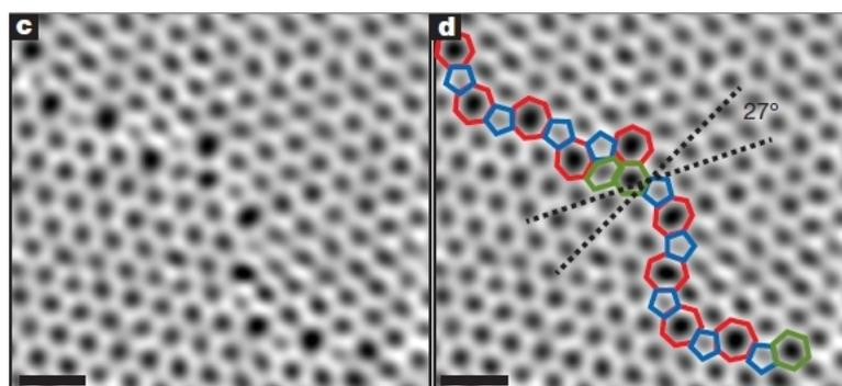
**Figure 3.6:** TEM image of a graphene grain boundary with  $27^\circ$  misorientation angle. In the right-hand image the defect structure of the grain boundary is indicated. Figure reprinted by permission from Macmillan Publishers Ltd: Nature, Ref. [81], copyright 2011.
