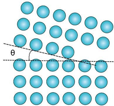
**Figure 1.1:** Two grains with the same structure and composition, but rotated by an angle  $\theta$  with respect to each other, forming a grain boundary.
