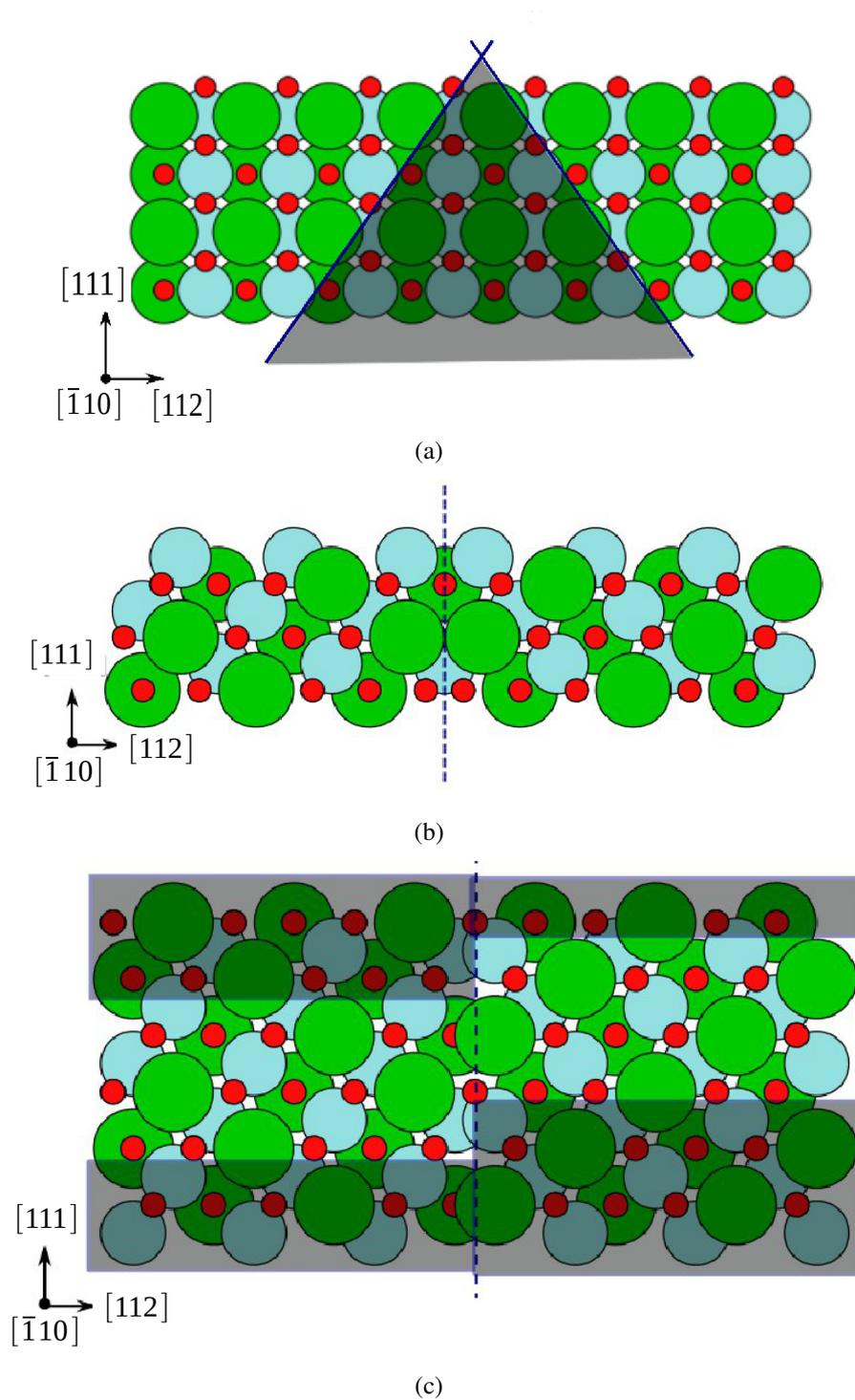
**Figure 5.1:** Creating the  $(112)[\bar{1}10]$  grain boundary. The block in 5.1(a) is cut perpendicular to the  $[112]$  and  $[\bar{1}10]$  directions. The shaded area is removed. Tilting around the  $[\bar{1}10]$  direction produces the symmetric configuration in 5.1(b). Displacement by  $2/3$  lattice periods in the  $[111]$  direction creates 5.1(c). Dashed lines indicate the grain boundary plane.
