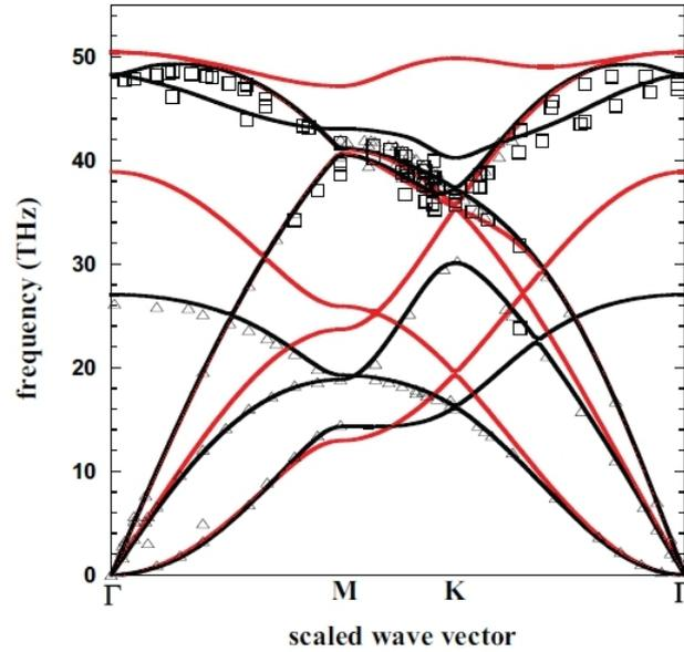
**Figure 3.5:** Phonon dispersion of graphene as calculated using density functional perturbation theory (black lines) and the bond-order potential used in Papers IV and V (red lines). The symbols represent experimental results. Reprinted with permission from Ref. [63]. Copyright 2014 by the American Physical Society.
