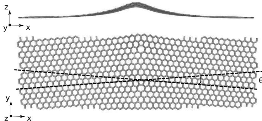
**Figure 6.1:** The  $9.4^\circ$  grain boundary, seen from the  $y$  direction (top) and the  $z$  direction (bottom). Figure from Paper V.
