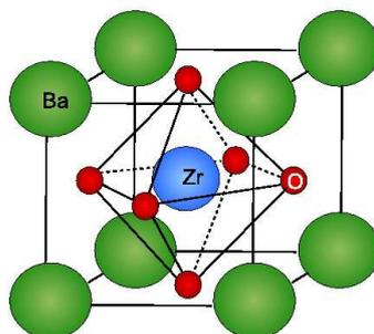
**Figure 2.2:** The cubic perovskite structure of BaZrO<sub>3</sub>.
