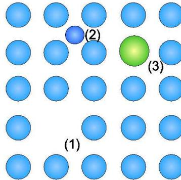
**Figure 2.5:** Schematic depicting point defect types, a vacancy (1), an interstitial (2) and a substitutional defect (3).
