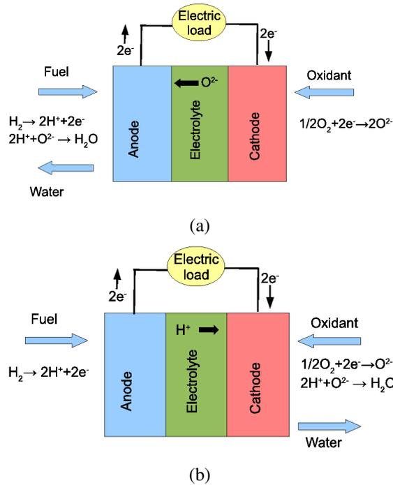
**Figure 2.1:** Schematic of fuel cells with (a) an oxygen ion conducting electrolyte and (b) a proton conducting electrolyte.
