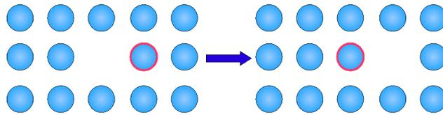
**Figure 2.8:** Schematic of the vacancy diffusion mechanism. An atom next to the vacancy (picked out in red) moves to fill the vacancy, which is thereby displaced one step to the right.
