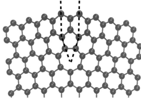
**Figure 3.7:** A dislocation in a graphene sheet. Dashed lines indicate the "added" strip of carbon atoms.
