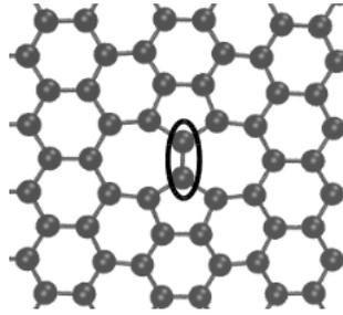
**Figure 3.9:** A Stone-Wales defect, with the rotated bond indicated by an ellipse.
