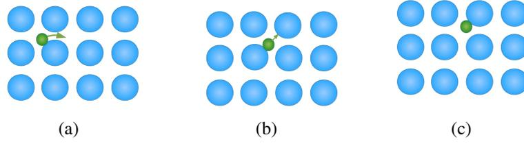
**Figure 2.6:** Schematic depicting the movement of a proton (green) in the oxygen sublattice (blue). The proton will first rotate around the oxygen ion (a) and then transfer to a second oxygen ion aided by relaxation of the oxygen lattice (b). Figure (c) shows the proton at the second oxygen ion.
