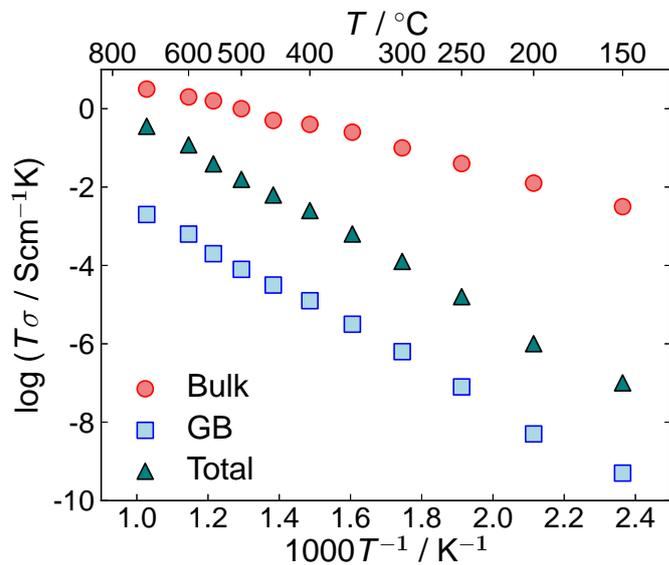
**Figure 2.4:** Comparison of bulk, grain boundary and total conductivity in BaZrO<sub>3</sub>. Bulk and grain boundary conductivities are taken from Ref. [23]. The total conductivity is calculated assuming a grain size of 1  $\mu\text{m}$ . Figure from [24], reprinted with permission.
