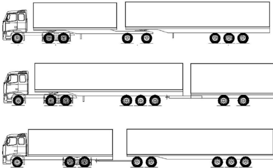
**Figure 2.1:** Illustration of vehicle combinations longer than 18.75 m currently allowed in Sweden: B-double (top), tractor semi-trailer and centre-axle trailer (middle), and truck dolly and semi-trailer (bottom). The figure is based on [3].
