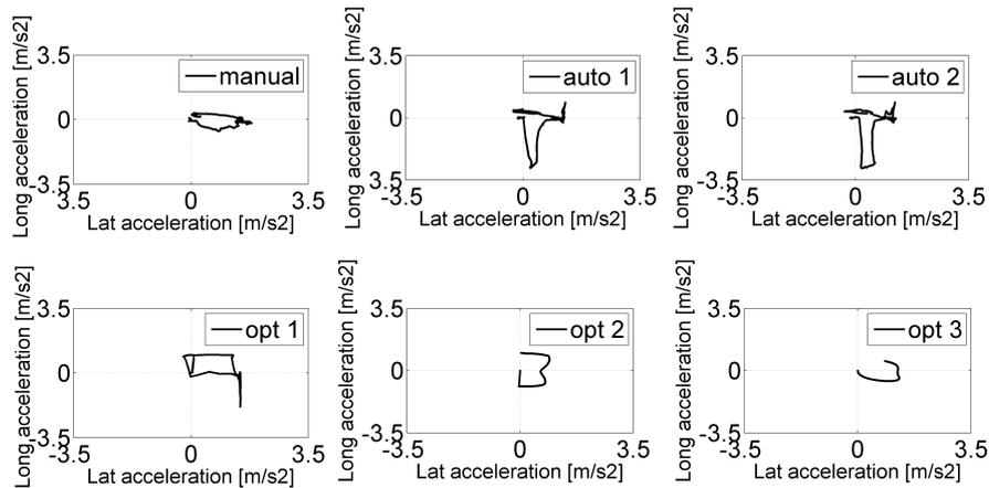
**Figure 5.2:** G-g diagram for a left curve with minimum radius of 150 m. The manual drivers had a mean speed of approximately 60 km/h during cornering. Mean values of manual driving (top left), automated driving 1 (top center), automated driving 2 (top right), opt 1 (bottom left), opt 2 (bottom center) and opt 3 (bottom right).
