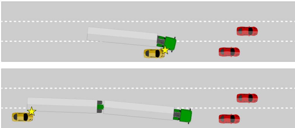
**Figure 3.1:** Top panel: Typical blind spot accident involving an existing vehicle combination, together with a lane change to the right in right hand traffic. Bottom panel: Hypothesized lane change accident including LVCs.
