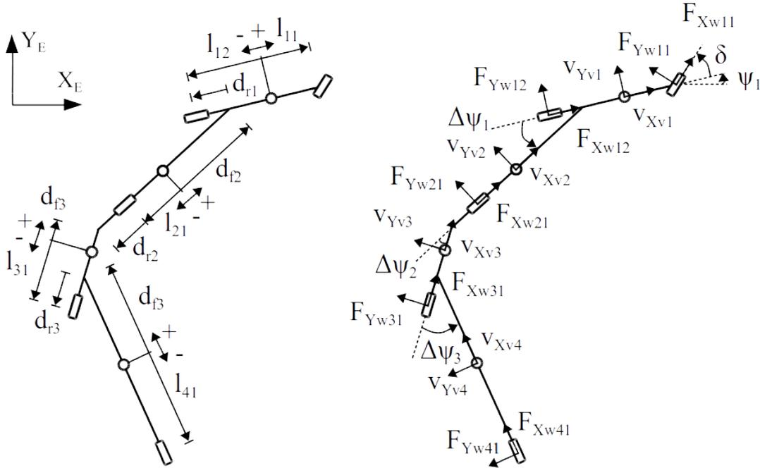
**Figure 4.3:** Illustration of a one-track model of an A-double combination. The left panel illustrates the spatial parameters of the vehicle model and the right panel illustrates the included motion variables and tyre forces. The spatial parameters are defined as positive if they are in front of the unit's CoG and negative if they are behind the CoG.
