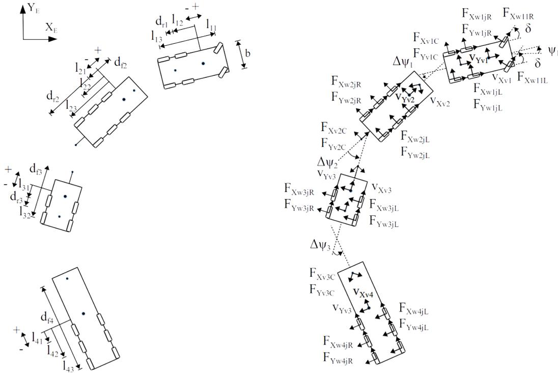
**Figure 4.2:** Illustration of a two-track model of an A-double combination. The left panel illustrates the spatial parameters of the vehicle model and the right panel illustrates the included motion variables and tyre forces. The spatial parameters are defined as positive if they are in front of the unit's CoG and negative if they are behind the CoG.
