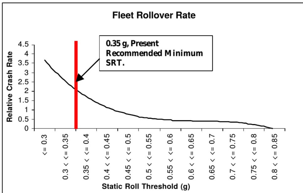
**Figure 4.5:** Illustration of relative crash rate versus static roll-over threshold for heavy vehicles in New Zealand. The recommended minimum static roll-over threshold (SRT) in New Zealand is  $0.35g$  (units of  $g$ ). Figure from Mueller et al. [26].
