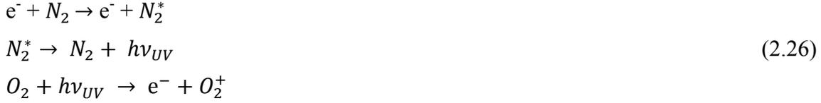
The frequency interval considered for UV photons  $h\nu_{UV}$  in air radiated by excited nitrogen molecules is 98 – 102.5 nm.
